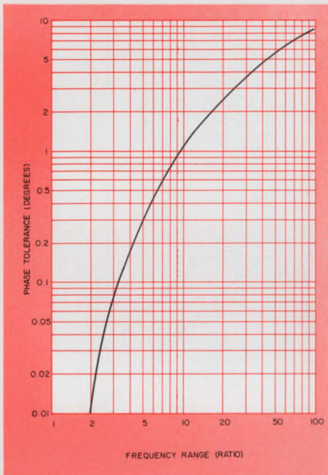
4. A four-pole phase shifter exhibits this theoretical relationship between frequency range and phase tolerance. If a tighter tolerance is required, more poles must be incorporated into the circuit.
