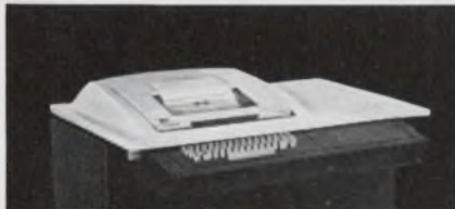
Inktronic® data terminals: A unique electronic, solid state terminal. Prints up to 1200 wpm. Forms characters through electrostatic deflection (no typebox). ASCII compatible.
