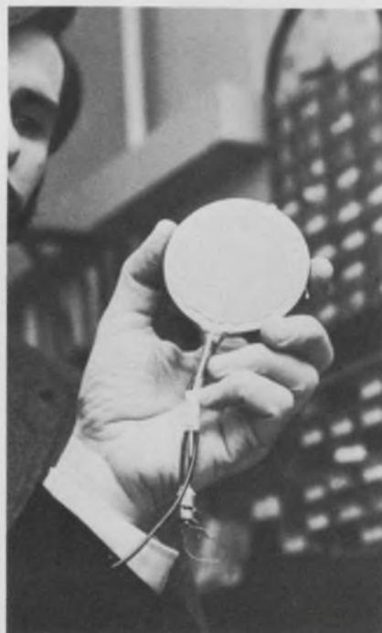
Experimental pacemaker uses biological feedback loop that eliminates the need for battery power.
