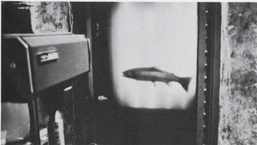
Salmon passes viewing window at the Willamette Falls, Ore., automatic counting station. A closed-circuit TV camera relays the picture to a video tape recorder later used in fish identification.
