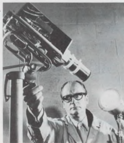
Color TV space camera withstands light from sun gun without damage.
