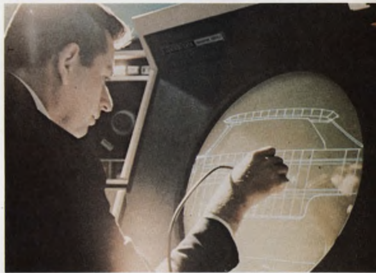
Automotive systems are designed by computer-aided design techniques at Ford Motor Co.'s Dearborn, Mich., plant (Session 4G).
