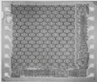
Model 1101 , a 256-bit MOSRAM with 1.5 \mu sec maximum access, drops in price by 60% to 73%. Now competes in price with small core memories.
