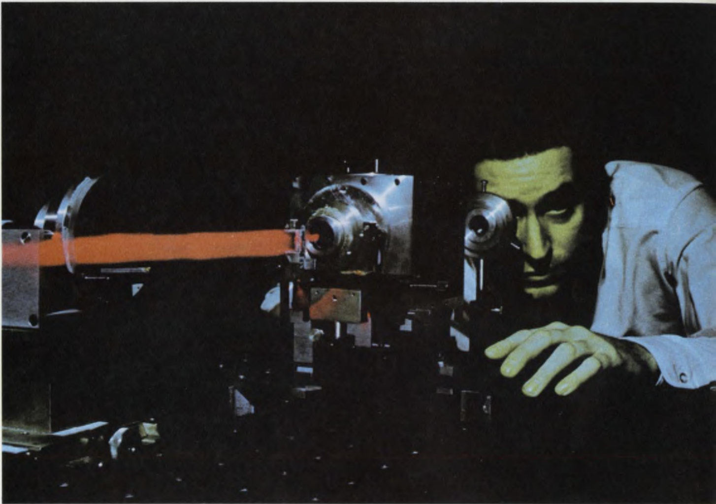
Peering into his upconverter is A. H. Firester of RCA, Princeton, N.J. The device is used to convert infrared
