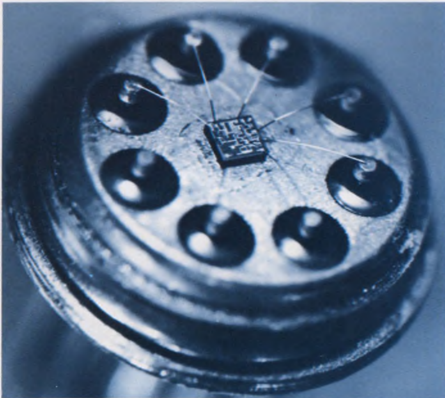
Differential IC operational amplifiers, which are also useful as direct-current amplifiers, can deliver output currents as large as 70 mA. p. U146.
