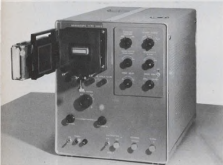
From dc to 5,000 MHz is the range of this Matsushita Nanoscope, which uses a traveling-wave CRT.
