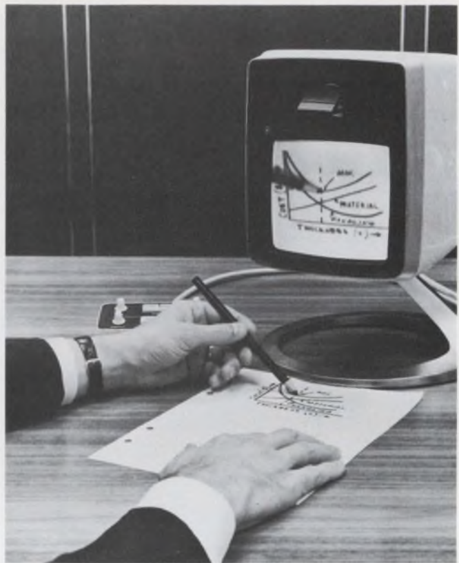
Picturephone developed by the Bell System can be used to transmit drawings or charts (Session 5B).
