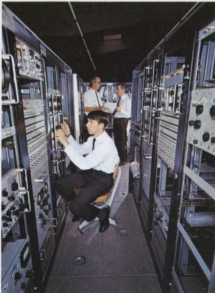
Checking out a satellite isn't simple. This mass of gear at Hughes Aircraft in El Segundo, Calif., is only part of the transportable systems test equipment needed to check out an Intelsat IV.
