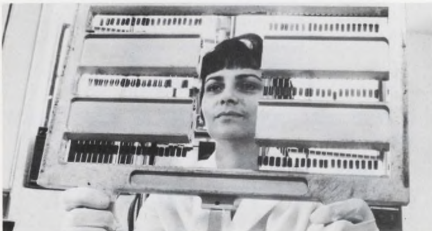
Solid-state rectifiers to replace tube components for color TV. Such devices eliminate sources of ionizing radiation.
