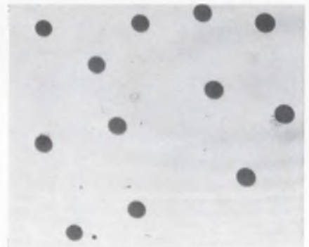
Before the bubbles are formed the magnetic domains look like fingerprint ridges and valleys. Domains shrink and bubbles appear (right). Bubbles shown above are about 1.4 mils in diameter.
