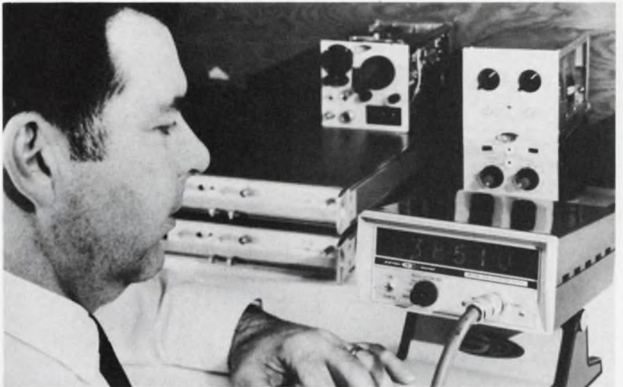
Miniature microwave counter by Systron-Donner counts from 300 MHz to 3 GHz. It will be on display at booth 1412.
