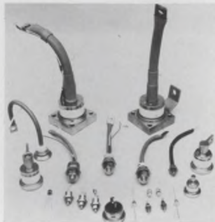
J-band solid-state generator (top) is manufactured by M. O. Valve under the Genalex trademark. Semiconductor devices (bottom) from AEI include SCR's and plastic rectifiers.
