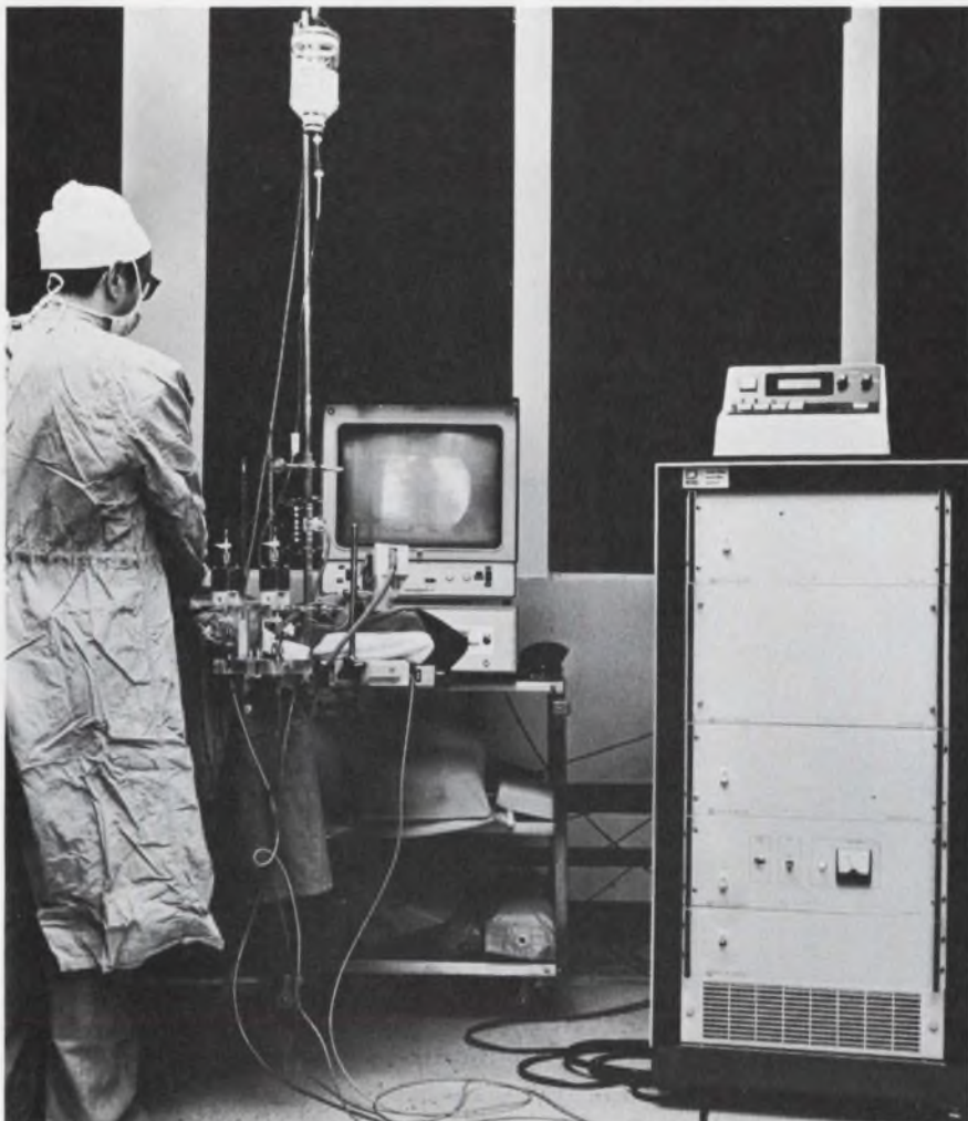
Video disc recording system (right) , developed by Data Disc Corp., is connected to standard X-ray equipment at Stanford University Medical Center in Palo Alto, Calif. The X-ray motion pictures are recorded and played back at slow speed for the physician.
