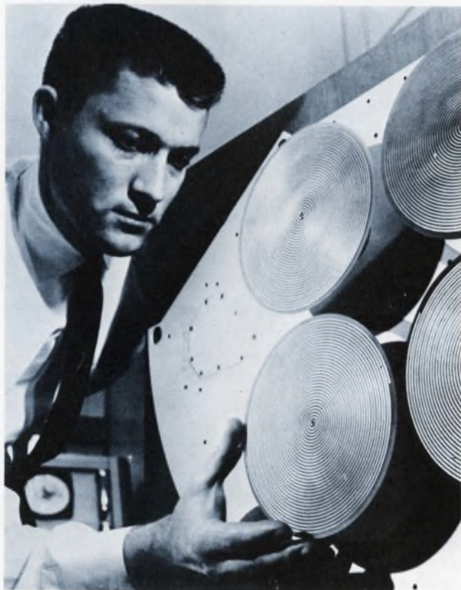
14. Four spiral antennas used for space-vehicle applications take advantage of the low-loss properties of silicone laminates. The antennas, made by Westinghouse, consist of copper strips, etched to form a spiral pattern, and bonded to a silicone-glass laminate. (photo courtesy Dow Corning Corp)
