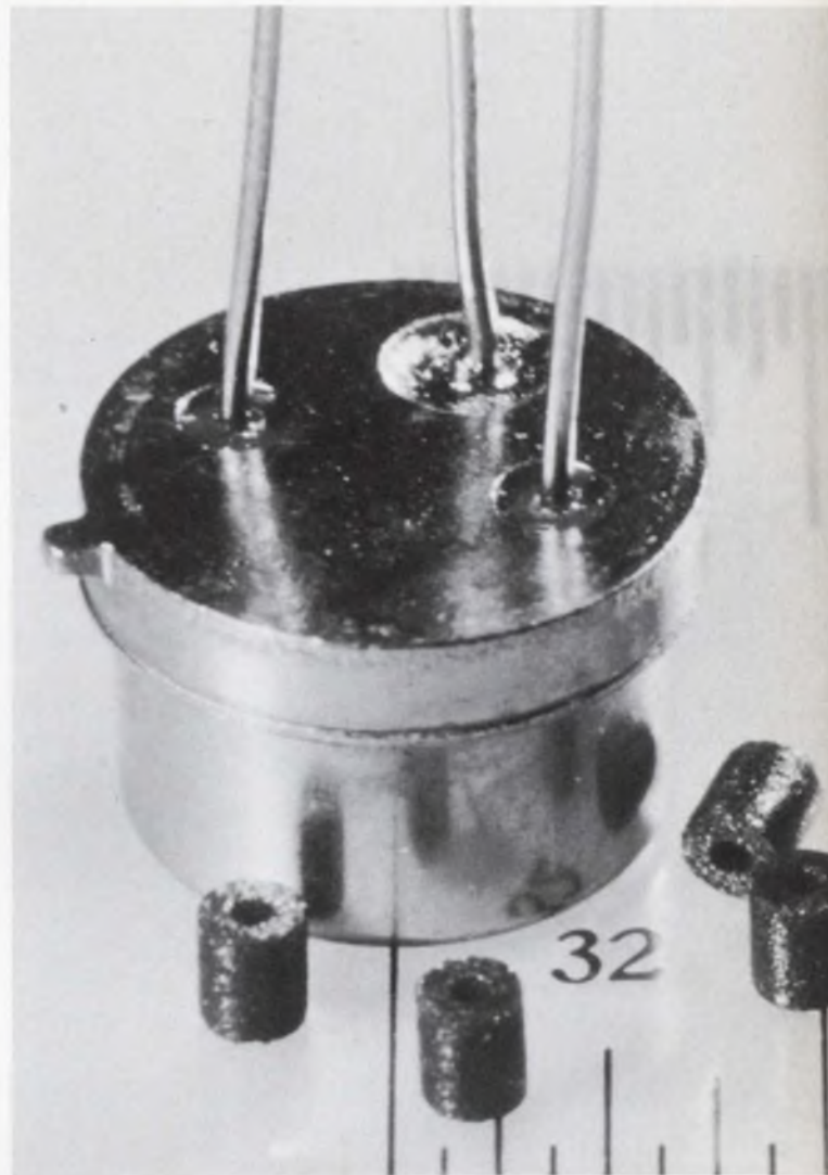
19. An example of the role of glasses in modern electronics is Corning Code 9013 lead-free glass, which is used for its constant dielectric properties.
