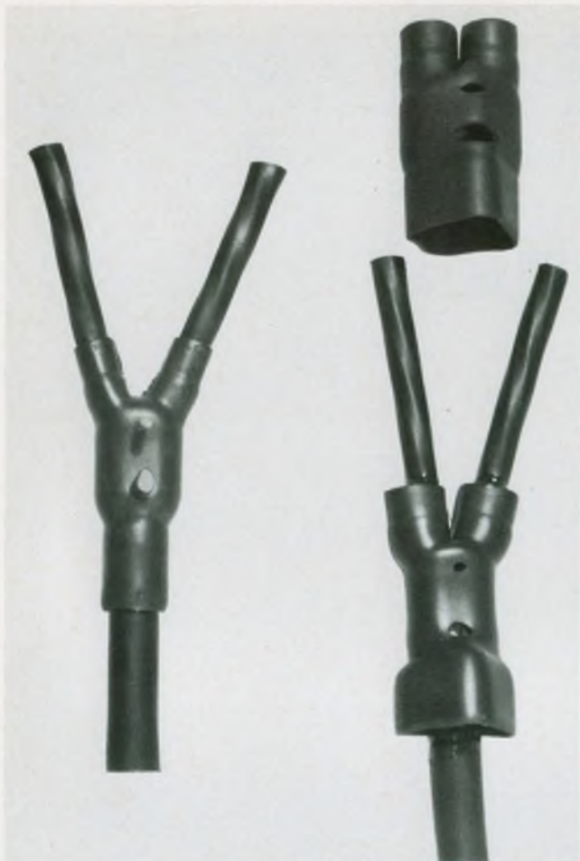
26. Irradiated, cross-linked polyolefins find use as heat-shrinkable cable boots. After being set in place, the oversized boot is heated, shrinking tightly around the cable. (photo courtesy Rayclad Tubes, Inc.)
