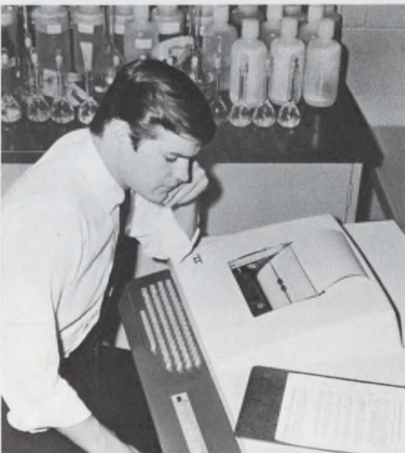
Data terminal prints up to 1200 words per minute over standard lines. p. 154.
