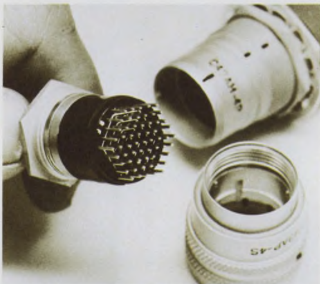
3. Miniature connector uses a glass-filled diallyl phthalate (DAP) molding compound to provide insulation between all of the 61 pins. Designed by Microdot, the multi-pin insert has a recommended working voltage of 750 V rms. (photo courtesy FMC Corp.)
