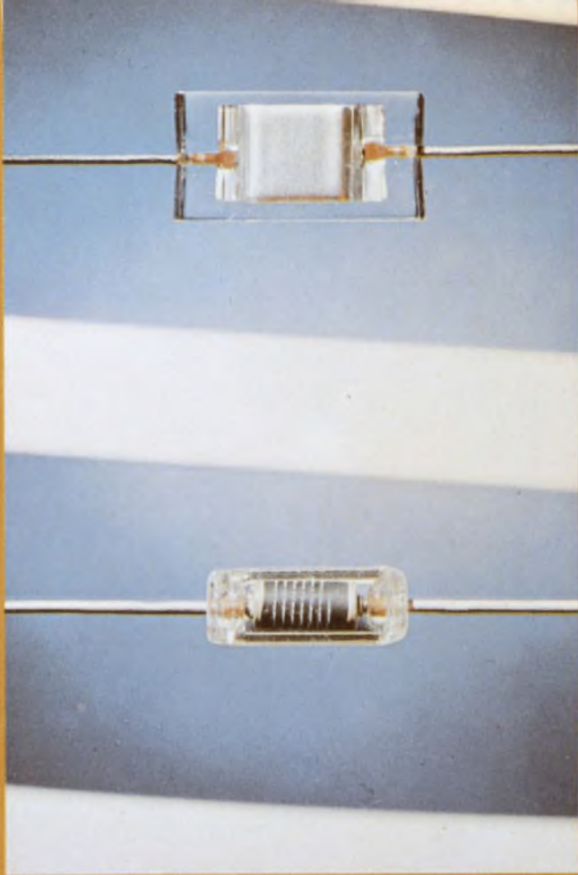
Glass is used as a sealer for this resistor and capacitor. The resistor element itself is a glass rod onto which a tin-oxide film is fused. (photo courtesy Corning Glass)
