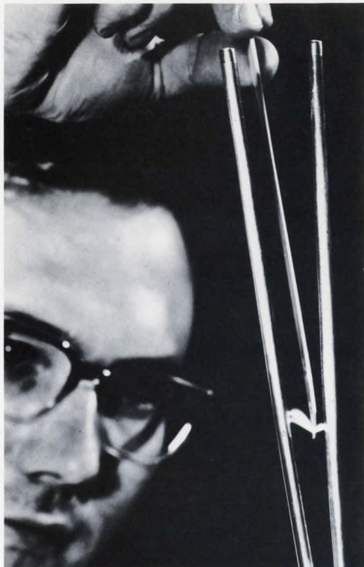
17. Dielectric strength capabilities of boron nitride are demonstrated by detouring a 10,000-volt arc with a 1/32-inch thin strip of the material.
