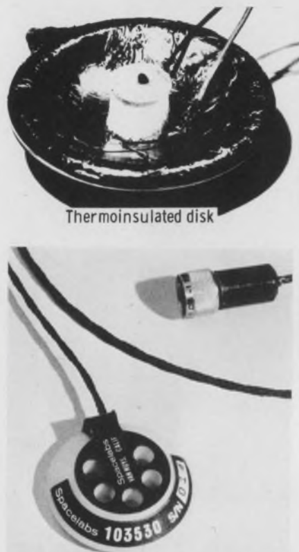
3. Relatively crude body-temperature sensor for Project Mercury, at top, compared with more recent Project Apollo skin-temperature sensor, at bottom. Rapid advance in sensor technology is evident.
