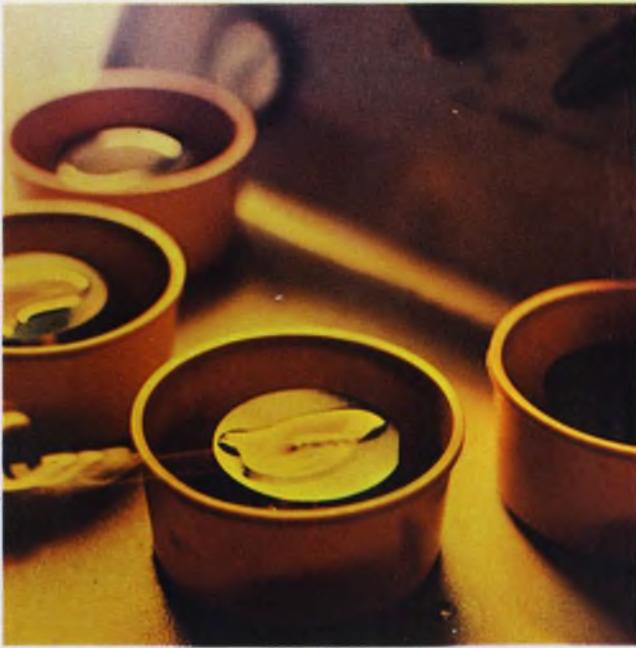
In an ultra-clean spinning hood, MOS wafers are coated with photoresist in preparation for photo-etching. The wafers are spun at 7000 rpm for 2 minutes to remove the excess, leaving a uniform coating of resist about 0.4 microns thick. The air in the hood is filtered to exclude all particles over 5 microns in diameter, and the photoresist to exclude particles over 0.5 microns, to minimize pinholes in the photoresist layer. Photo courtesy of National Semiconductor, Santa Clara, Calif.
