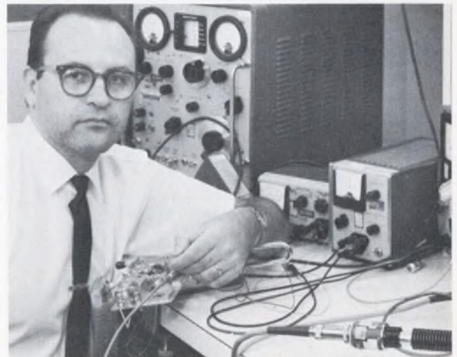
The author, Arpad D. Vincze, is holding a \times 24 frequency multiplier/rf amplifier chain.
