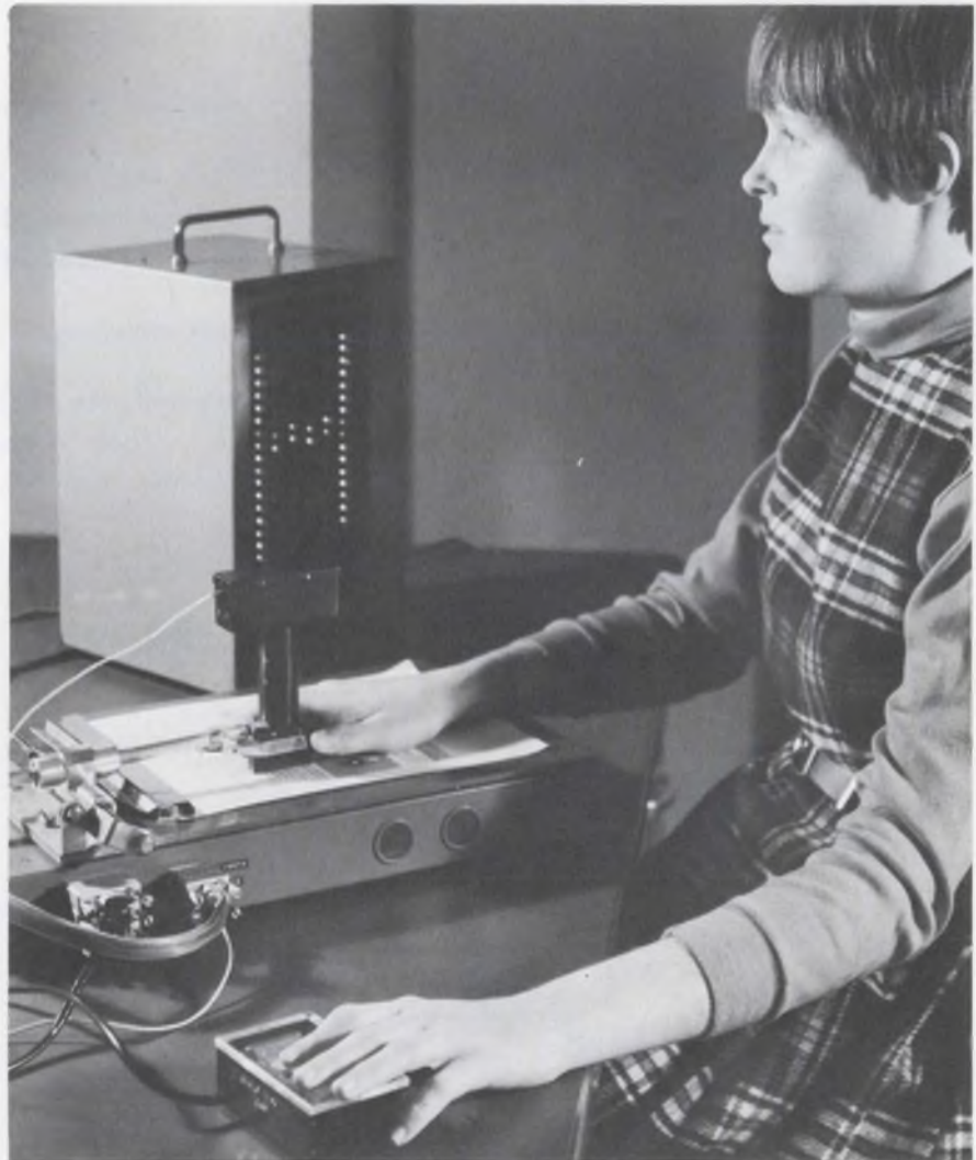
To use the Bliss-Linville portable tactile reading aid, the operator moves the probe along the line of print and feels a bundle of stimulator pins vibrating in the shape of the letters. The light display box is used for visual troubleshooting.
