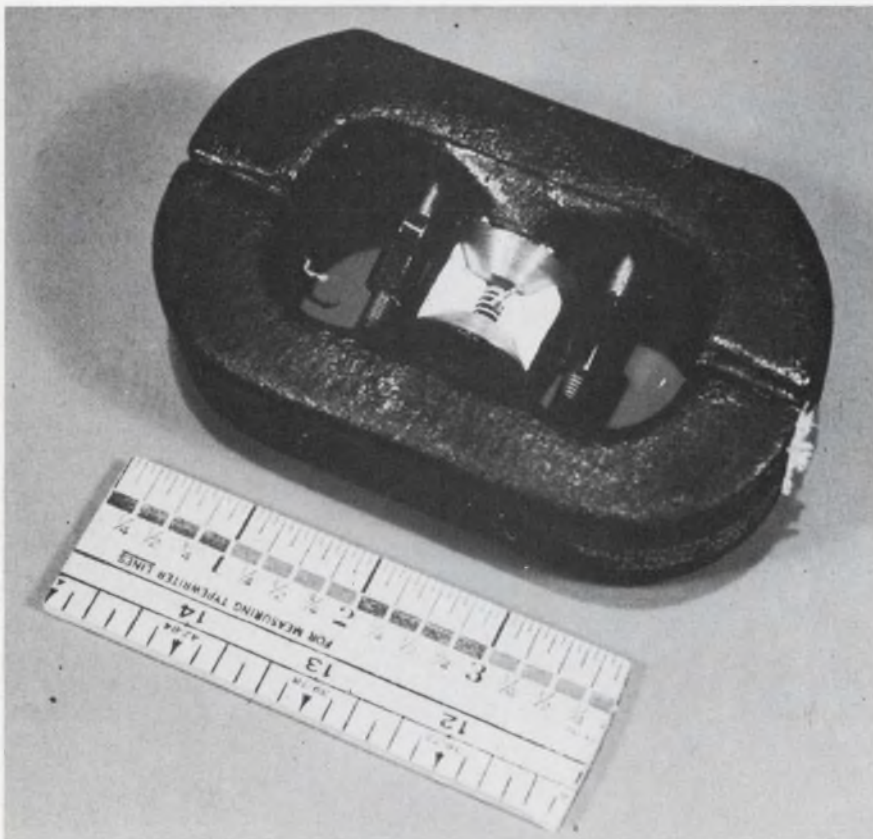
1. Lab model of ferrimagnetic echo system used by Lockheed scientists delays, amplifies, compresses and expands X-band microwave frequencies at room temperature.
