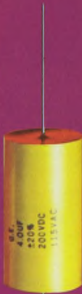
Polyester Tubular Capacitors (left) 296 standard ratings. 100 and 200 volts d-c, 0.0010 to 2.00 \mu f, -55 to 85C
