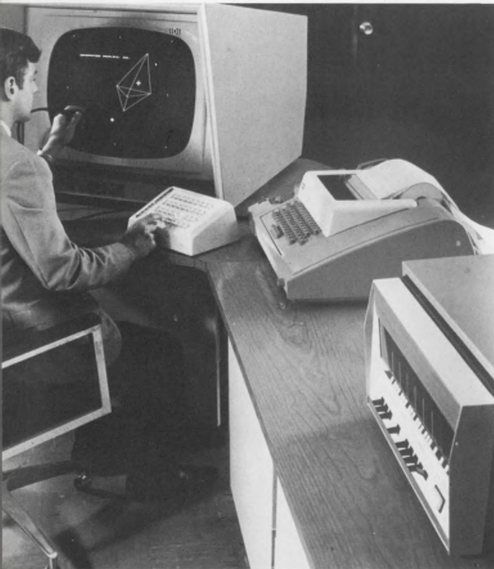
1. IDIOM graphics terminal has 32 function keys with changeable coded meanings. Informations Displays of Mt. Kisco, N.Y., sells it for $79,000.
