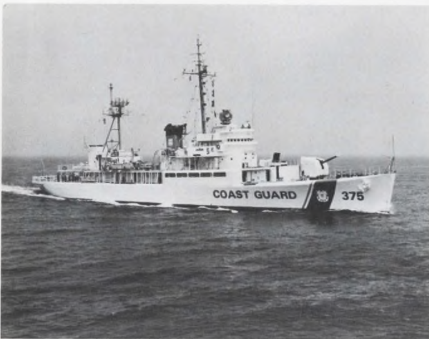
The Chincoteague is the first ocean-station Coast Guard cutter to receive the AN/SPQ-10 Shipboard Radar Set, a modernized version of the 1951 MK-56 Gun Fire Control Radar. Largely unchanged, the four-foot radar dish and pedestal are visible above and behind the bridge.
