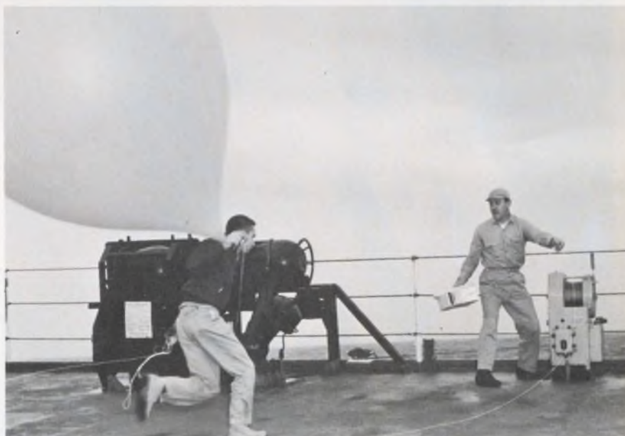
Weather balloons are launched every six hours from Coast Guard weather ships to provide meteorological data to the Weather Bureau and to commercial ships and aircraft. The SPQ-10 will track these to 100,000 feet and provide immediate outputs for teleprinter transmission.
