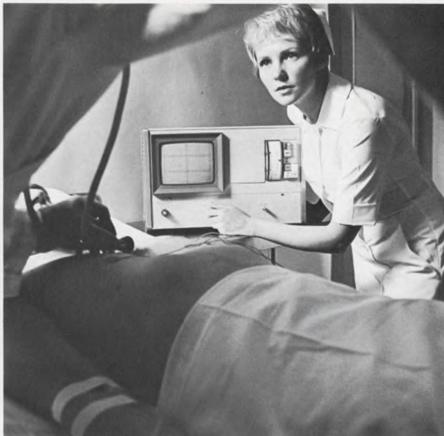
Bedside unit of patient-monitoring system contains an electrocardiogram channel, an oscilloscope display, a cardi tachometer, and an audio alarm. The unit was built by Honeywell, Inc., Denver.
