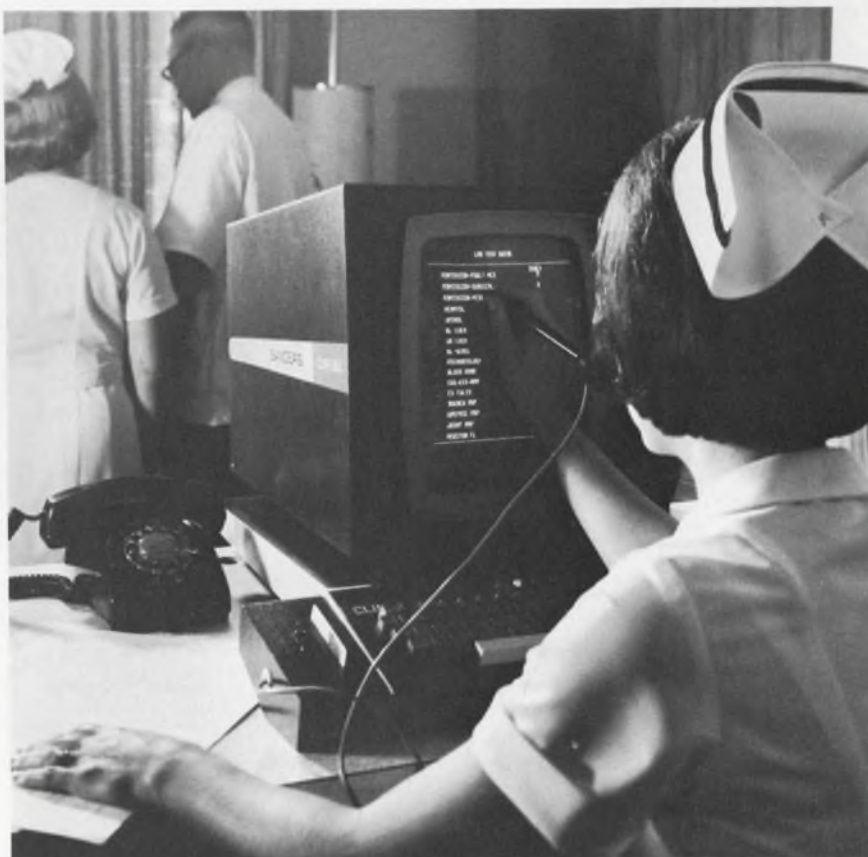
Nurse touches light pen to the display portion of a medical management system. Up-to-the minute patient data is provided in the system, developed by Sanders Associates, Inc., Nashua, N.H.
