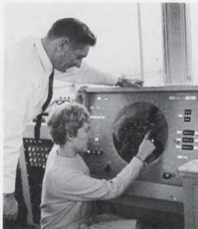
Radar beacon system shows Grumman engineers alphanumeric flight data on planes under test.
