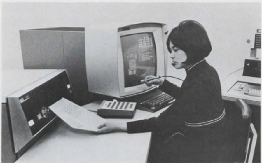
3. Copies from a graphics terminal can be made in 15 to 38 seconds in this system that uses IBM's 2250 unit and a new 3M photosensitive paper copier.
