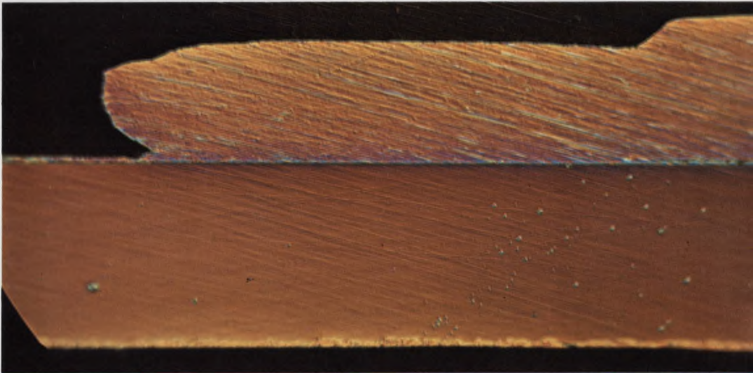
Aluminum lead is ultrasonically bonded to silicon which has been metalized with aluminum. This method of bonding does away with contaminants, evolves little heat or pressure, and gives a strong bond. Since ultrasonic
