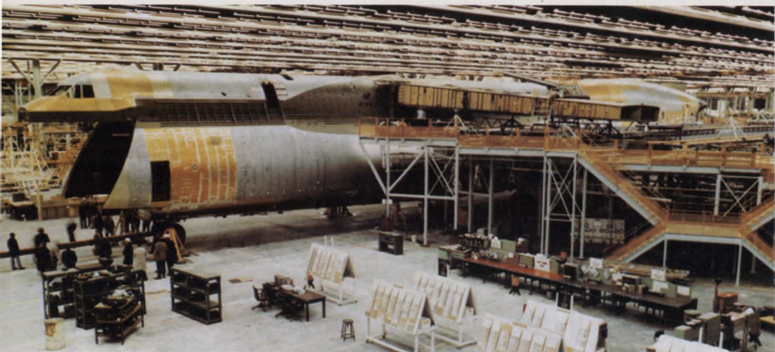
The Air Force C-5A Galaxy, under construction at the Lockheed-Georgia Co. plant in Marietta, Ga., will carry up
