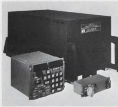
The Litton LTN-51 inertial-navigation units include, at left, the platform and computer system, a control display unit and a mode selector switch. On the right is the control display, as installed in the cockpit of an American Airlines plane during recent flight tests.
