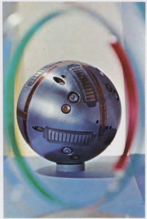
A gimballess stable sphere houses the electronics in the Nortronics inertial platform, which can operate at any altitude.
