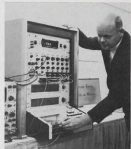
Dynamic testing is performed by Computer Test Corp. tester by connecting a sampling oscilloscope to an internal pulse generator.
