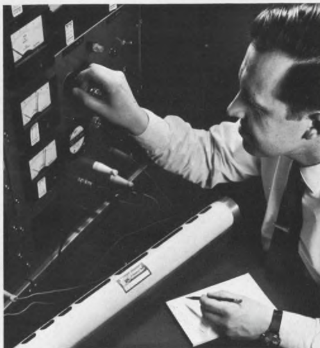
Testing an O-type delay line, Jack Lucken adjusts the bias voltage on the electrode that controls the delay.
