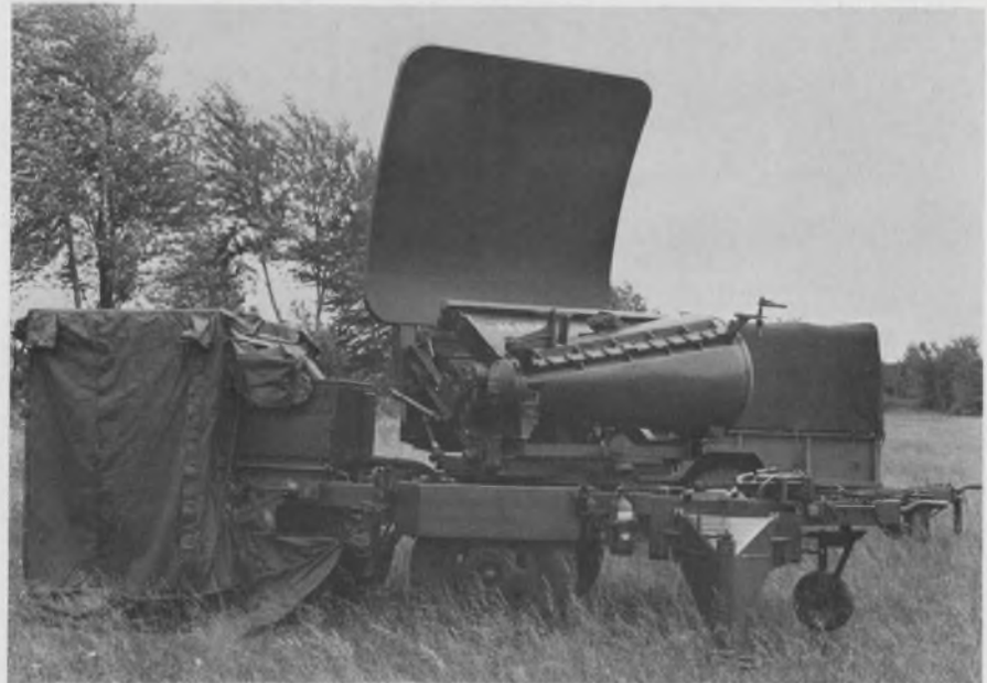
Mortar-and-rocket-locating radar, AN/MPQ-4 , which has been around for 10 years, is proving itself against the Viet Cong. General Electric is building additional systems, but the Army still seeks an omnidirectional mortar locator.
