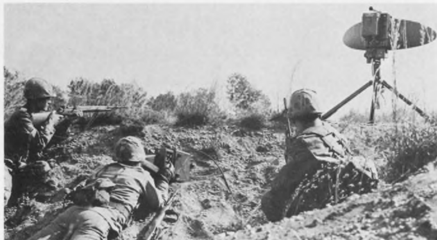
Infantry troops use the AN/PPS-5 to detect the approaching enemy. The soldier in the center position is viewing target movement on a dual CRT attachment, but headphones can also be used to hear Doppler tone changes.
