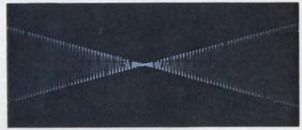
Crossover null on scope display helps to establish the equal-amplitude test signals.
