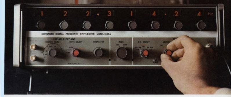
**Computer-aided design and integrated-circuit construction in this new Frequency Synthesizer bring a new level of perfection to signal generation.** The new "4th generation" Model 3100A Digital Frequency Synthesizer obsoletes just about every current concept of general purpose signal sources. Pick your frequency from 0.01 Hz to 1.3 MHz in 0.01 Hz steps. The result—signal purity you can
