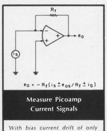
1.5pA/°C ( $i_b$ ) and noise of only 0.1pA the 147 can resolve signal currents as low as one picoamp. Voltage drift errors ( $e_{os}/R_f$ ) are negligible for  $R_f$  greater than 10<sup>7</sup> ohms. Flame detectors, phototubes, ion gauges, and semiconductor tests are typical applications.
