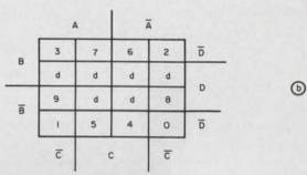
2. The basic Karnaugh map (a) has 16 possible states for a four-stage binary shift register. Each decade of the decade shift register is also made up of four flip-flops but is limited to only 10 possible states (b).
