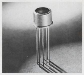
Hybrid op amp ranges to 200 kHz and is packaged in a TO-5 can. Page 90
