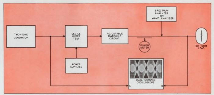
1. **Basic setup for two-tone test** may use one of three popular read-out devices—oscilloscope. spectrum analyzer and wave analyzer. Each should be chosen accord-
