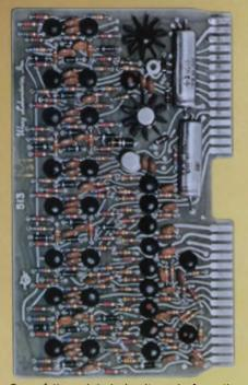
One of the printed circuit cards from the Model 320 calculator. All resistors on this card are Allen-Bradley Type CB  $\frac{1}{4}$  watt hot molded resistors.
