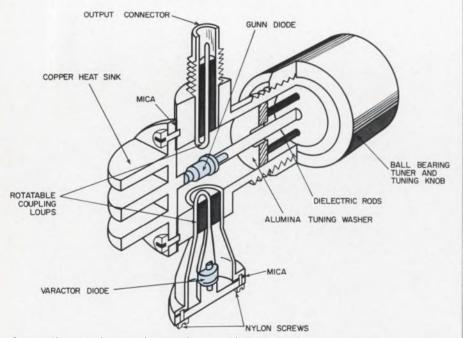
**Gunn-effect device**, to be used as a klystron replacement, contains a Gunn diode oscillator and a varactor diode for electronic tuning. This British device is about  $1 \cdot 1/2$  inches long and uses a dielectric washer for mechanical tuning.
