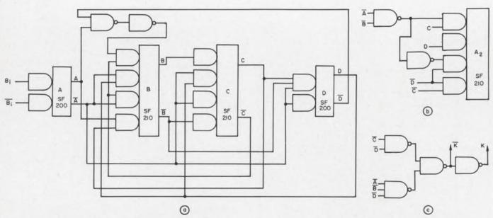
5. Four flip-flops and one quad gate are needed to implement one decade of the converter (a). The carry may be generated by using the two spare gates and some of the gates of the next decade (b), or by using a further pair of gates (c). The first method (b) is slightly faster than the second (c).
