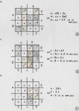
3. The Boolean equations for each flip-flop are found by enclosing the states that change on the next shift. The simplified equations hold if internally crossconnected J-K flip-flops are used.
