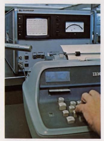
**Subject loudness** is plotted on the scope face while the meter shows the absolute loudness. Hewlett-Packard's loudness analyzer selects the proper spectrum with comb filters and performs complex analog signal processing to arrive at these data, which formerly had to be calculated manually. But there are no linear integrated circuits in the filter system.
