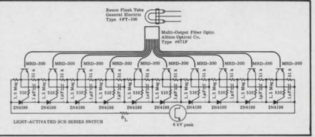
MRD300 combined with 2N4198 ELF° SCR (600 V) gives total ton of 300 ns. Single light source coupled by multiple-output fiber optic bundle transmits light to photo transistors. Fast ton is accompanied by gate isolation advantage.
