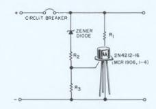
SCR Crowbar Over-Voltage Protection for DC Operation
