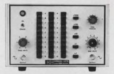
MODEL 4100, brand new R-C Oscillator with push-button frequency control. Sine- and Square-Wave simultaneously from 0.01 Hz to 1 MHz. Price \$550, Provides performance of higher priced units. 5%" H x 8%" W x 14½" D.
