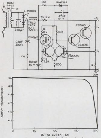
**Improved temperature stability** is the result when a pchannel FET is used as a reference element in this lowvoltage, regulated power supply capable of delivering up to 18 mA.
