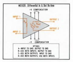
New linear I/C boasts differential outputs as well as differential inputs . . . making it a good universal operational amplifier.
