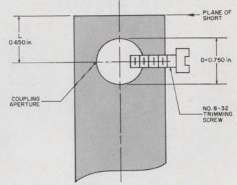
**Trimming screw** increases coupling bandwidth from 71 to 96 MHz at a center frequency of 2 GHz.
