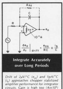
amplifier performance for integrator circuits. Gain is high too  $(A=10^6)$ giving  $10^{17}$  ohm equivalent leakage resistance  $(AR_d)$ . Low bias current allows small capacitors to be used for a given accuracy.
