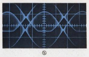
(36, 30 and 39 dB below the fundamental was measured for the third-, fifth- and seventh-order products for (a), and 27, 30 and 45 dB for (b), respectively.) The lower traces are the inputs.
