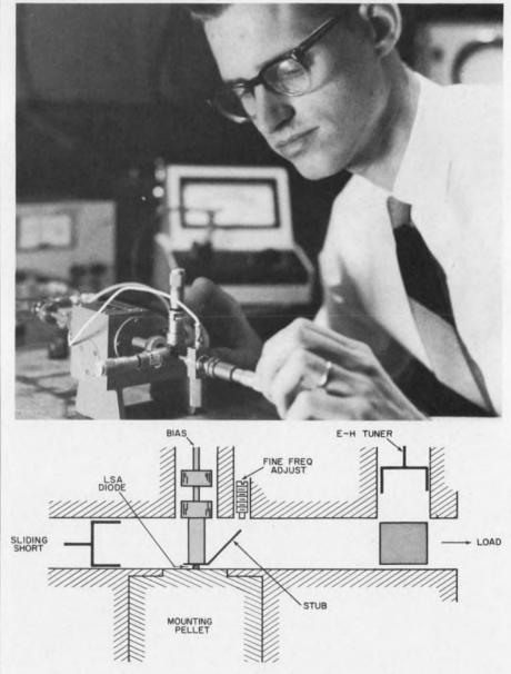
An unpackaged LSA millimeter-wave oscillator is adjusted by Dr. John A. Copeland. The circuit produces 20 mw of cw power between 44 and 88 GHz. The waveguide short and tuner load the circuit for maximum output. Frequency is primarily determined by the tab-like stub.
