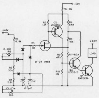
**Two independent delay times** are obtained with this circuit. The switching of the load by applying +48 V to the input is delayed by the amount determined by  $R_{13}$  and  $C_1$ . Off delay is determined by  $R_{14}$  and  $C_2$ .
