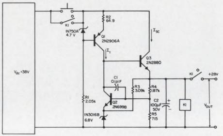
Relay protects regulator circuit against short-circuit overloads.
