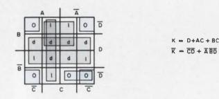
4. All possible states are enclosed on this Karnaugh map since the carry digit (K) is generated by gates and not by a flip-flop.
