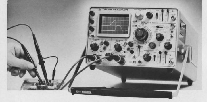
**The Tektronix Type 454** is an advanced new portable oscilloscope with DC-to-150 MHz bandwidth and 2.4-ns risetime performance specified at the probe tip. The new P6047 10X Attenuator Probes and the optional FET and current probes are designed to solve your measurement problems.
