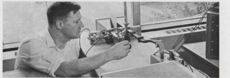
**Experimental X-band radar** at Cornell uses a limitedspace-charge-accumulation-(LSA) diode to obtain 60 watts of peak power. At left, Prof. Lester F. Eastman tunes the diode mount. At right, the transmitter assembly (the
