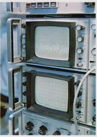
**Noise signals are replacing impulse trains** in many tests. A typical noise signal from the Gaussian output of Hewlett-Packard's pseudo-random noise generator is shown on the general-purpose oscilloscope (top trace). A multichannel analyzer monitors the noise pattern and plots its probability density function, which verifies the Gaussian nature of the noise (bottom trace).
