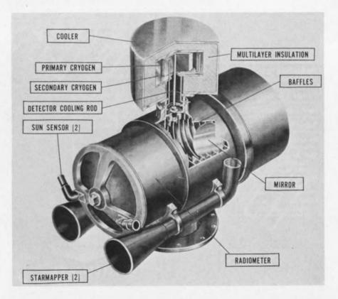
sensing is paramount, for if detectors could determine the true terrestrial horizons fore and aft of a spacecraft along its orbital path, then the bisector of this angle would be the true local vertical, or the position over the Earth. The need for complex on-board instrumentation would be eased.
