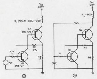
**Solid-state snap switch** uses two complementary silicon transistors (a). It turns on for  $V_{1n} = 1.4$  V and turns off when  $V_{1n} = 1.1$  V. A simple oscillator is shown in (b).
