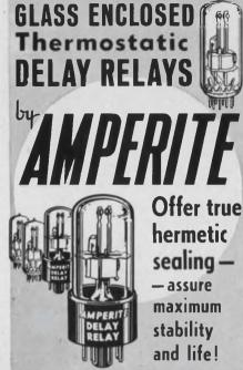
Delays: 2 to 180 seconds Actuated by a heater, they operate on A.C., D.C., or Pulsating Current ... Being hermetically sealed, they are not affected by altitude, moisture, or climate changes . . . SPST only --- normally open or normally closed . . Compensated for ambient temperature changes from -55° to + 80°C. ... Heaters consume approximately 2 W. and may be operated continuously. The units are rugged, explosion-proof, long-lived, and inexpensive! **TYPES: Standard Radio Octal**
