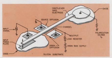
Westinghouse plans production of its resonant-gate transistor, a microcircuit filter element. As its biased gold beam moves, the MOS channel depletes the current path, causing an output. Evaluation units are available.
