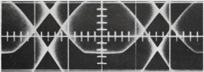
Distortion can be read in three ways that range from approximation to evaluation of all
