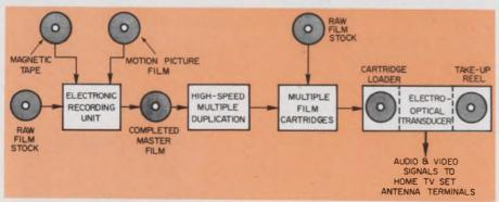
**Electron-beam scanning** permits playback of monochrome or color motion pictures on home TV sets. Variations in light intensity are converted into audio and video signals that are coupled to the antenna terminals of a TV set. Commercial prerecorded film is packed in 7-inch cartridges.
