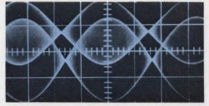
3. **Good output envelope** (top trace) shows no distortion. The bottom trace is the input. The measured third-, fifth- and seventh-order imd products are 30, 49 and 53 dB below the fundamental, respectively.
