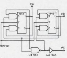
Three-phase square-wave generator can be realized with two flip-flops and half a quad 2-input gate. put is shorted, to avoid continuous heating by Q3.
