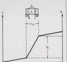
V=VOLTAGE AT ANY GIVEN POINT  $V_0 = ANODE VOLTAGE$   $V_D = DOMAIN VOLTAGE = V_0 - E_sL$   $E_s = \frac{dy}{dx} = FIELD INTENSITY$ L = LENGTH OF SAMPLE L\_D = DOMAIN WIDTH 2. Creat voltage access a p
