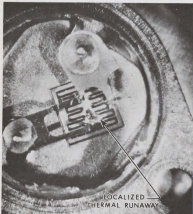
5. Results of secondary breakdown are seen on an npn silicon chip. The damaged area is indicated by the arrow.
