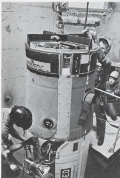
Minuteman II guidance section is installed atop third stage in silo at Vandenberg AFB.
