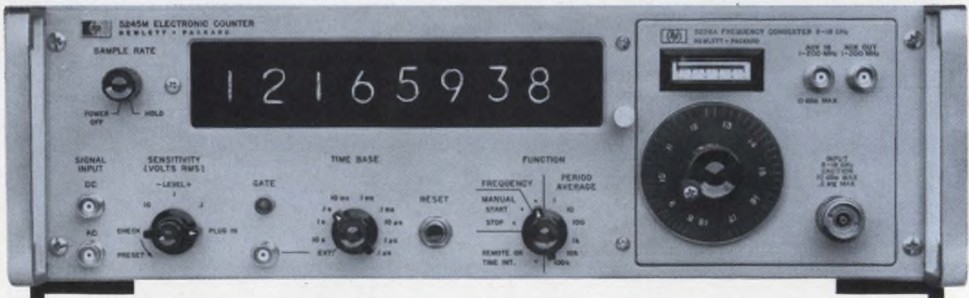
5245M COUNTER WITH NEW 5256A 8 TO 18 GHz FREQUENCY CONVERTER PLUG-IN
