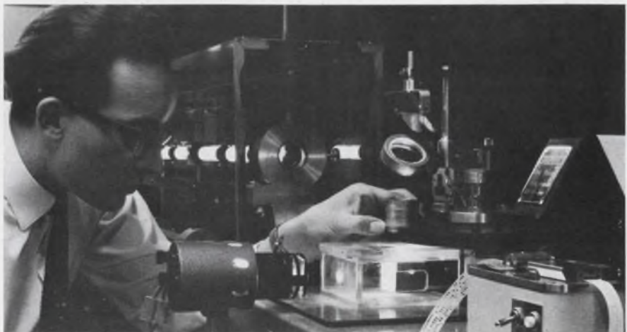
Interconnection patterns are deposited directly onto a semiconductor substrate by means of a helium-neon laser.
