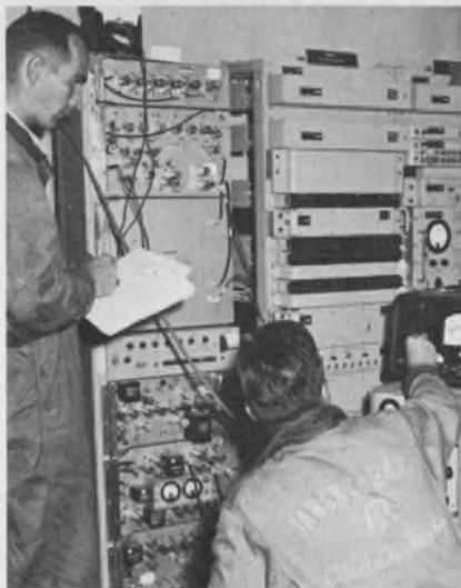
Sensitivity and dynamic range of an amplifier are being measured by Atlantic Research engineers to determine its compatibility.
