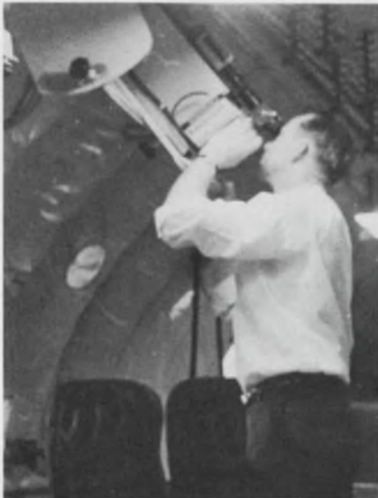
One of the two laser-referenced interferometer spectrometers is aimed by engineer Robert Pierce. Instruments are sensitive in 1- to 8-micron band and have nitrogen-cooled detectors.
