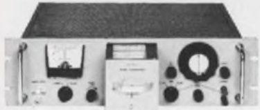
Model SR-60 Price: $850.00 Model SR-60. WWVB-60 khz. Will calibrate any local standard up to 5 \cdot 10^{10} within a short period. Can be easily operated by any technician and performs in any part of the Continental United States.
