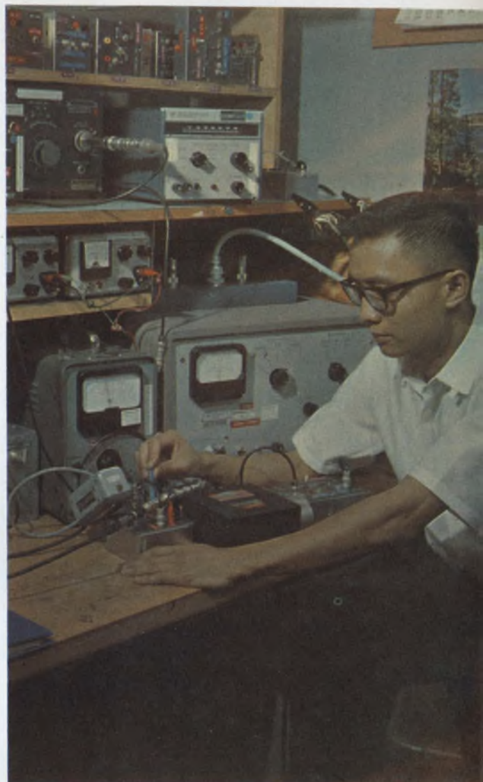
Noise figure measurements on an rf FET mixer are made by Siang Pink Kwok of Motorola Semiconductor, Inc. (Paper 8/1).
