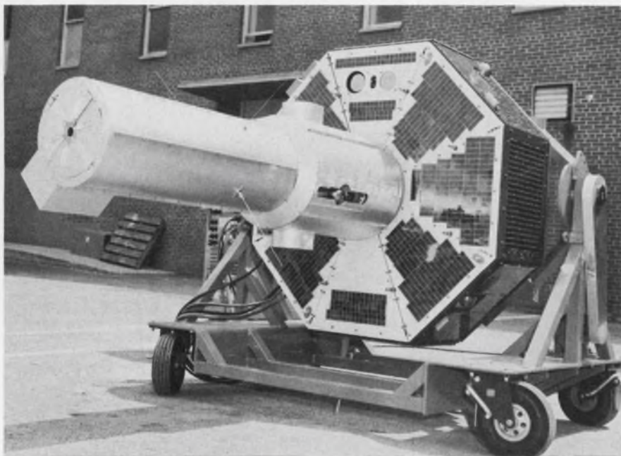
The Dodge satellite undergoing sunlight tests at the Applied Physics Laboratory of Johns Hopkins University before being shipped to Cape Kennedy.
