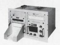
The BH103 incorporates a 100-point Scanner with direct digital readout and prints the data on folded paper. i.e., EVENTS, TEMP °F, TIME.
