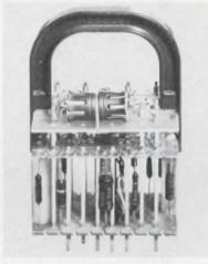
Mounting matched transistors for thermal stability so electrical characteristics stay identical is simple with back-to-back Therma-Link dissipators/retainers. Also used as heat sinks.
