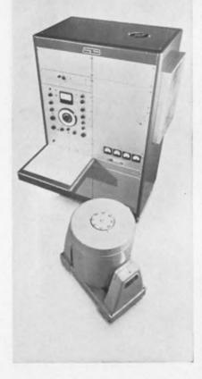
The shaker's moving element and its suspension are warranted for two years — a guarantee unmatched in the industry. System control is "push-button" — simple yet safe. It is thoroughly protected for all overdrive conditions with automatic shutdown circuits. For the complete story on Unholtz-Dickie test equipment, write today.
