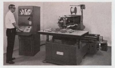
Tape-programmed TERMI-POINT Automatic Wiring Machine routes and fully terminates a  $10^{\prime\prime}$  lead in less than four seconds.
