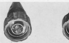
3. To remove cured urethane and reclaim expensive brass connector parts from this power connector (left, both photos), Uresolve was used to remove Products Research Corp. 1538 cable encapsulant. Neoprene cable jacket is unaffected (right, both photos).
