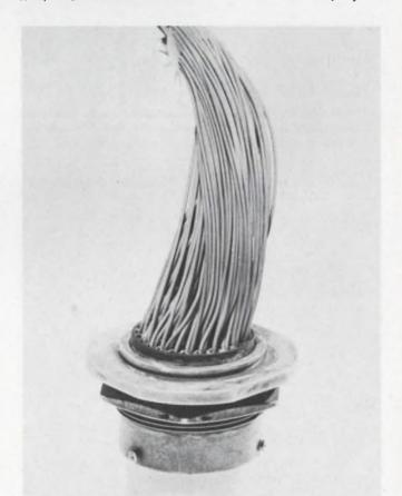
2. To replace a faulty wire in this cable assembly, Coast Pro-Seal 794 cured urethane encapsulant was removed with Uresolve. Materials of construction include anodized aluminum shell, neoprene insert, gold-plated connector, copper wire, irradiated polyethylene cable insulation and fluorinated silicone O-ring. The only material affected other than the urethane was the O-ring.
