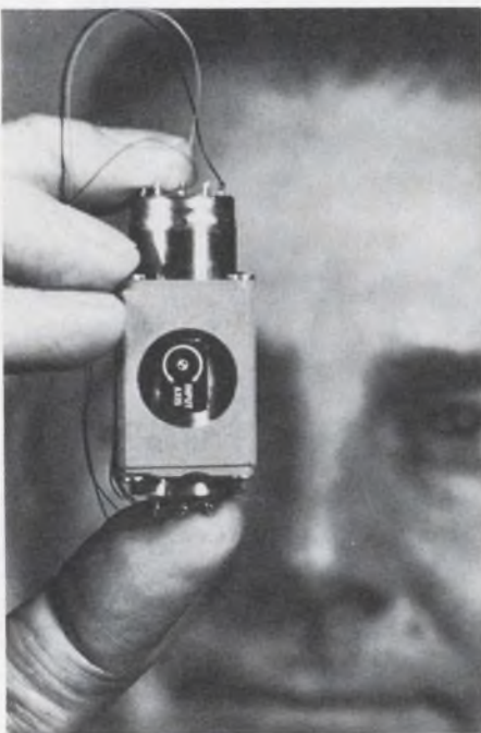
The DART gyro for aerospace use.
