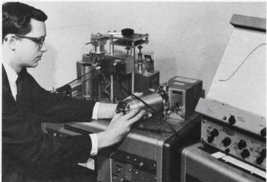
Photoelectric cell is plugged into new photodetector response recorder by National Bureau of Standards engineer David Goebel. A plot, representing a 4-minute scan of a photoelectric device, is shown on the x-y recorder. The monochromatic light source is in the background.
