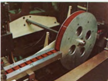
Fifth testing station tests 30 switching parameters at 25°C.
