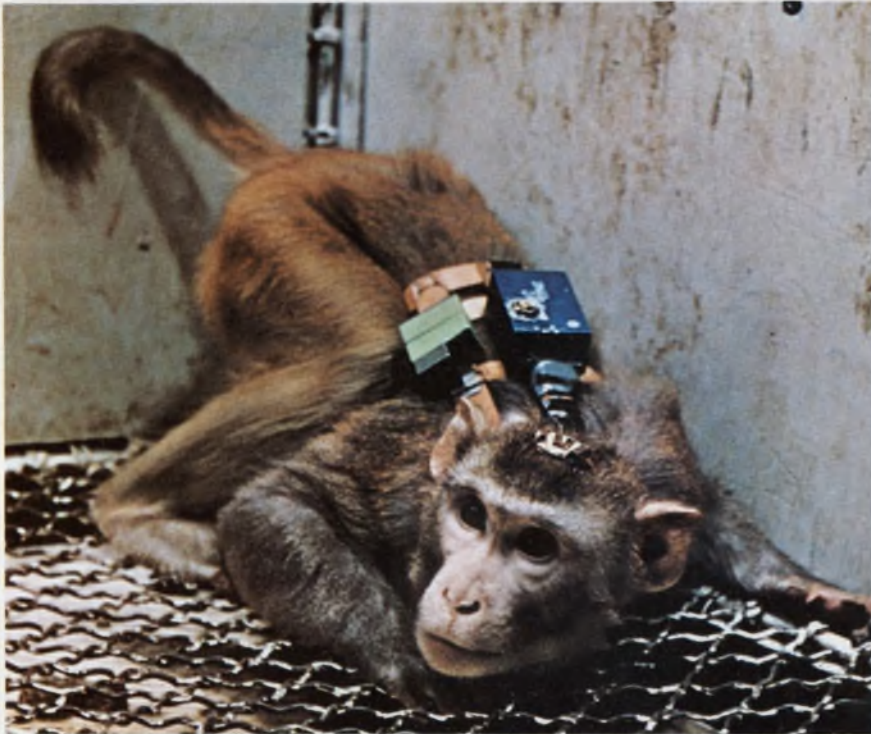
Radio-controlled stimulator weighs 28 grams, consumes 1.2 mA and operates at 100 MHz. Leads run to electrodes.
