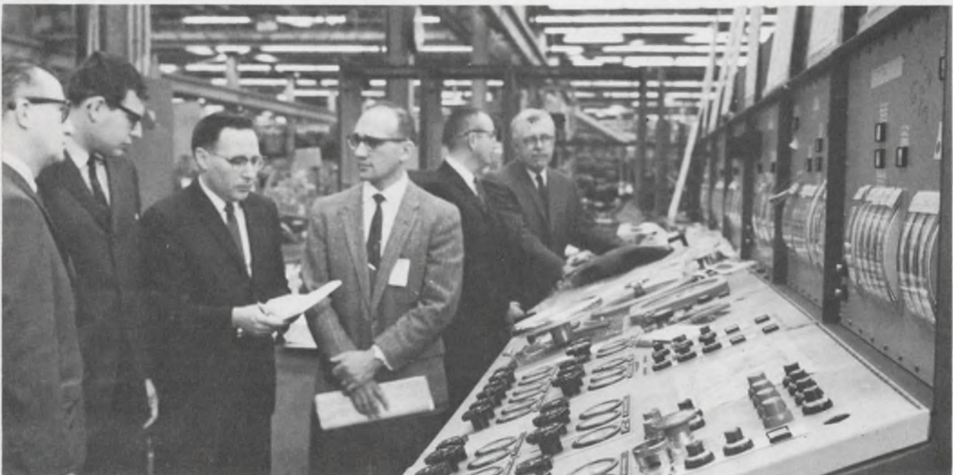
Engine-room console that will be installed in the American Lancer has three sections: data logging, ship's utility-
