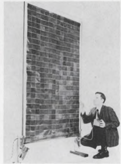
Thin-film solar panel that can be unfurled and furled in space is a possible spacecraft power source.
