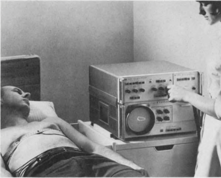
Vector cardiograph presents 3-dimensional data on heart activity. This Hewlett-Packard/Sanborn 1520A unit displays either vector loops of the total heart activity (shown on scope) or the individual vector components simultaneously (waveforms shown above). Sweep speeds as high as 1000 mm/s are possible with the unit.
