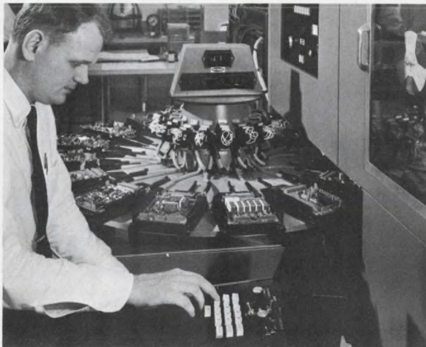
Infrared scanner detects any flaws in circuit production at Raytheon plant. Heat profiles of modules are compared with a standard as units rotate beneath the scanner on a "lazy Susan." Operator punches in circuit identification.
