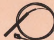
Surface Temperature Thermocouple Probe... Catalog No. 0187 (1000°F. Max.)
