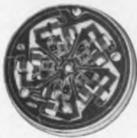
1-inch microcircuit developed at ECI for UHF digital synthesizer.
