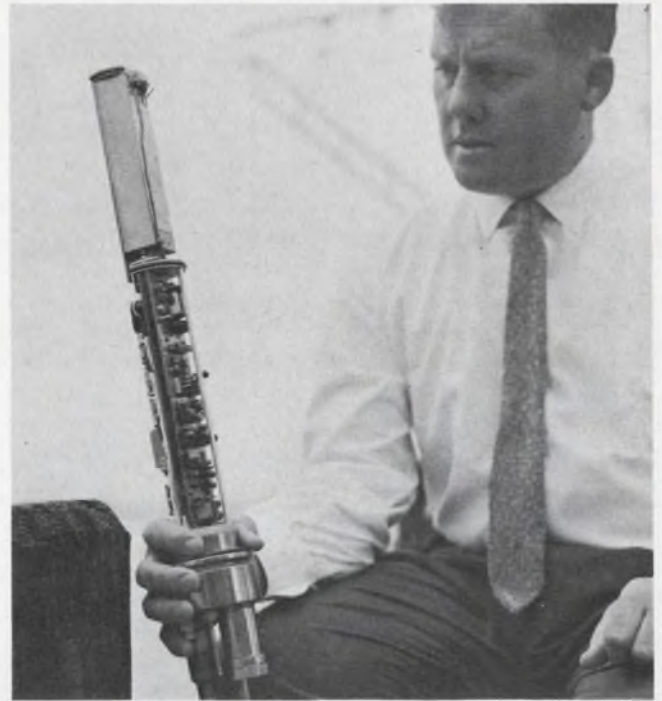
Latest Bissett-Berman in situ salinometer is held by its developer, Neil Brown. The unit incorporates a parameter-sensitive telemeter circuit. Instrument measures salinity of sea water by sensing its conductivity and automatically applying pressure and temperature compensation. Computed values are represented as frequency analogs.
