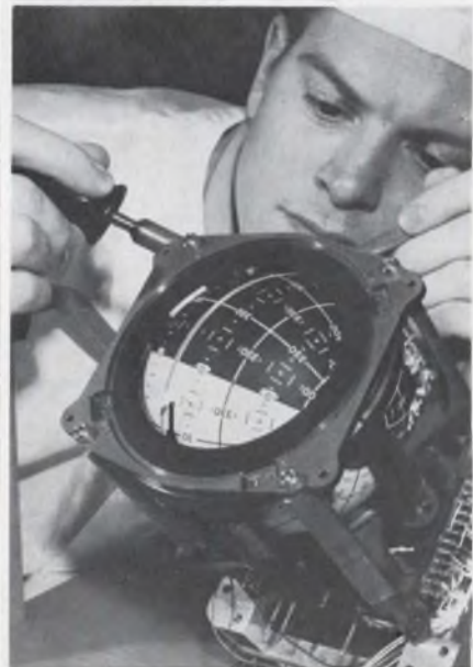
Flight director attitude indicator, examined by technician at Honeywell's Aeronautical Div. in Minneapolis, will help NASA's Apollo astronauts to keep their bearings in space. The electronic ball in the nine-pound cockpit instrument displays the Apollo spacecraft's attitude, attitude error and attitude rate along each of three axes—roll, pitch and yaw.
