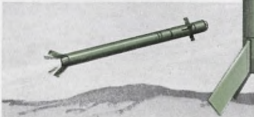
Infrared sensor locks on target. Miniature computer directs steering fins to guide Redeye.
