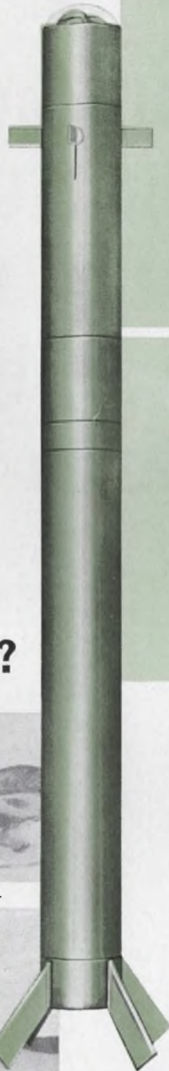
Infrared sensor locks on target. Miniature computer directs steering fins to guide Redeye.
