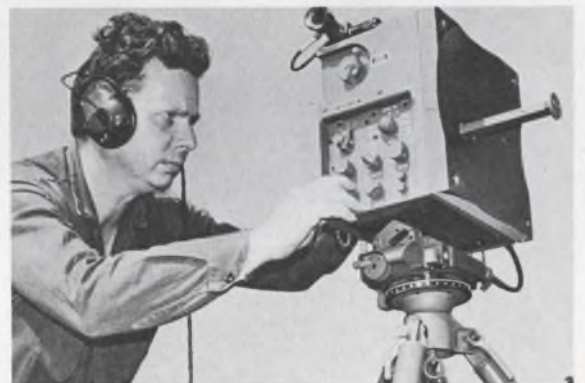
A 35-lb portable radar can detect a walking man a mile away. Page 40.
