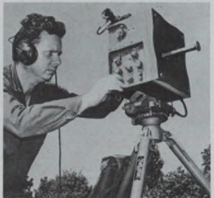
Portable radar in operation.
