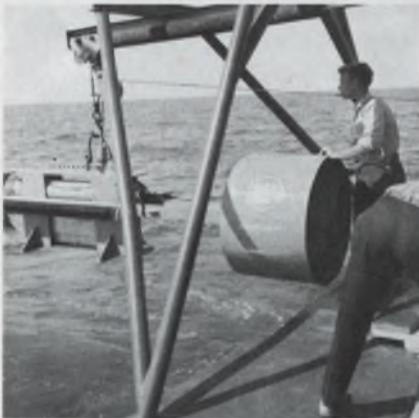
Westinghouse version of SLS fish is prepared for launch. Main frame of the unit is 6-in. steel I-beam. Transducer cases (black stripe) are along the beam sides, the electronic package is above, the batteries are below.
