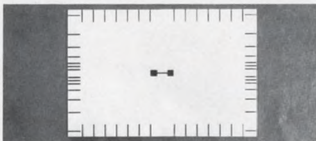
7. Sample for temperature variance versus area test has index lines to denote the various areas that are used.
