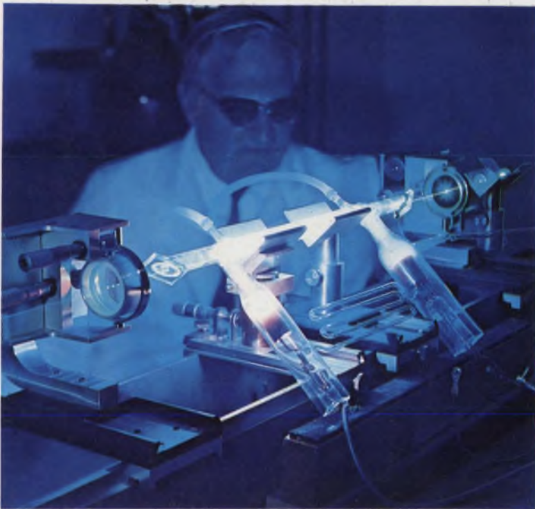
An early model of an ionized argon laser is adjusted by scientists of Electro-Optical Systems, Inc. This unit produced about 4.5 watts during continuous-wave operation. With a ceramic laser tube, advance devices produce about 3 watts continuous wave. These are being built under a classified military contract.
