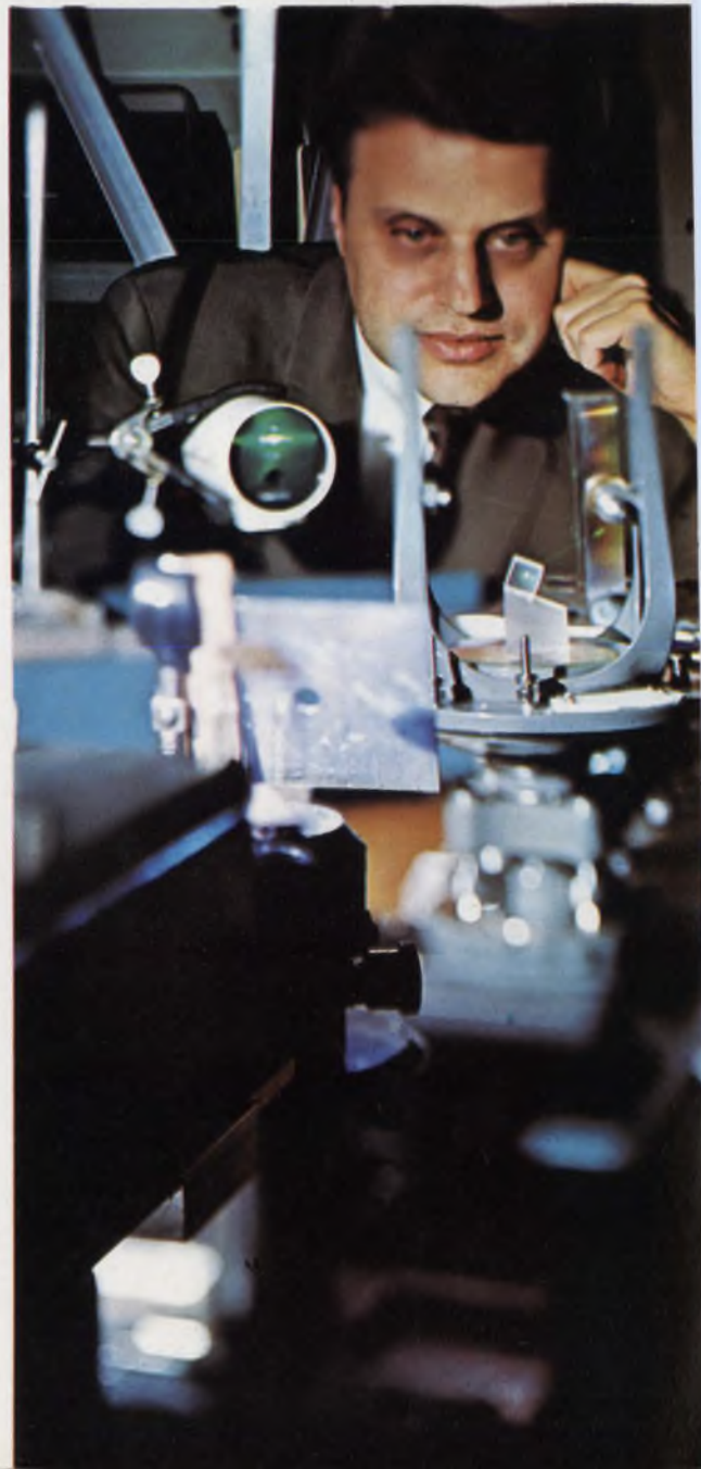
Green laser beam is generated by frequency doubling, from 1.06 to 0.53 \mu , with repetition rates up to 10 Hz at Electro-Optical Systems, Inc. Dr. Fred Johnson (in the background) says that it is particularly suitable for oceanographic applications, and may be used, with slight modification, for coded military systems.
