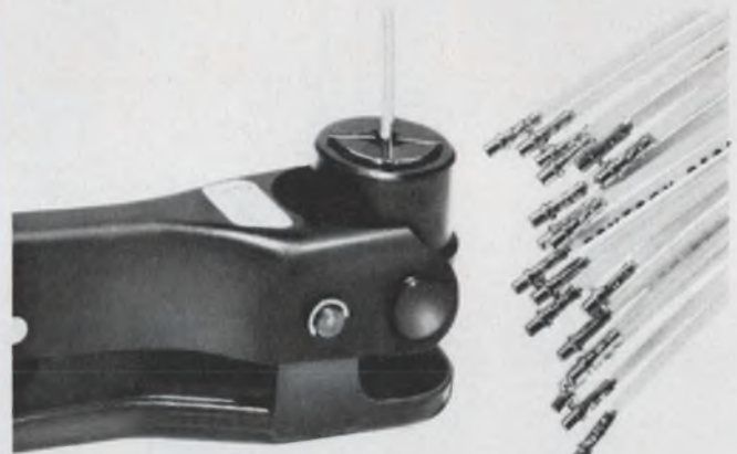
Quick, reliable crimp termination of wires with standard tools.
