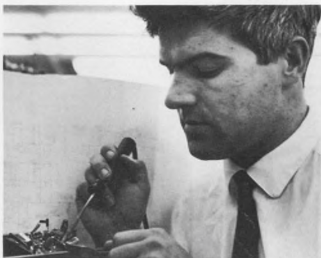
Using high-speed diodes, Author Bray constructs his remote gain-control circuit design. System gain is linear and temperature-stable, shows little distortion and is not subject to nonlinear characteristics of the diode.
