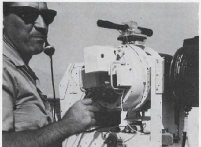
6. Feasibility of optical radars has been demonstrated with the Sperry system. The range and range rate data are presented in digital form.
