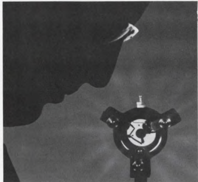
Sylvania's optical system uses an interference filter to modulate dual channel laser beam.
