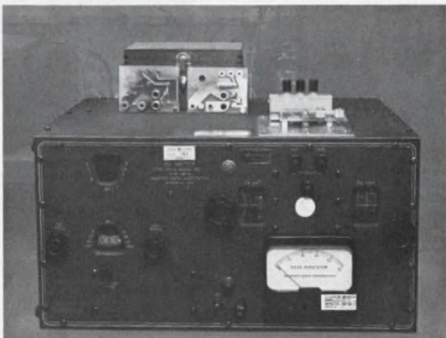
7. Boonton RX meter has extended capability with the addition of relatively low-cost transistor adapter plates.
