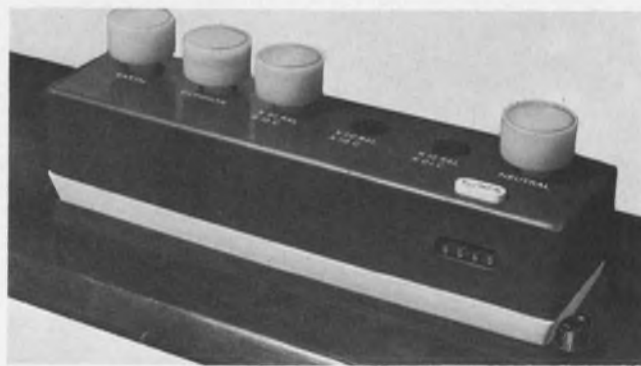
5. Adapter for WK601 unit measures just y_{21} parameter for npn transistor. Other adapters are available for other parameter measurements. Note the in-line socket arrangement which requires a socket adapter to mount transistor.
