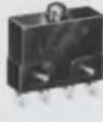
TYPE 18 SUB-SUBMINIATURE Smallest available single-pole, double-break, snap-action switch. Only .200" x .500" x .350". Over 15 million life cycles.
