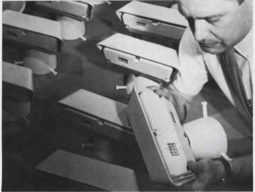
Antenna portion of ultrasonic detector is inspected by Sperry engineer.
