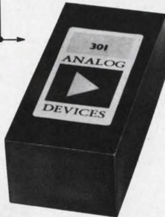
OFFSET CURRENT CHANGE of only 30 pa from -25^{\circ} to +75^{\circ}\text{C} , with 0.01 pa noise spec, enables current amplifier to resolve 10^{-13} amps, builds 9-decade log amplifiers
