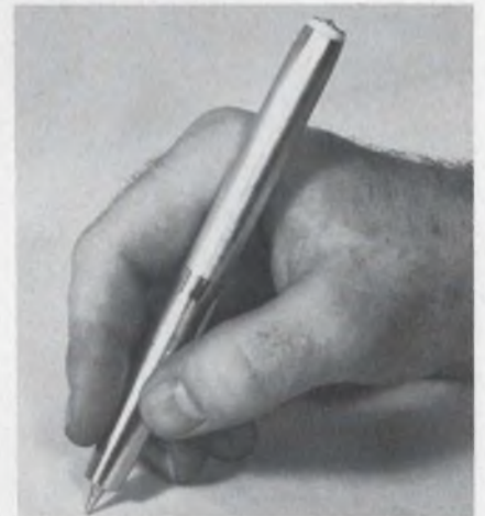
It looks like a pen, but don't expect it to write. This RF noise generator will effectively jam the output of any nearby bugging transmitter.
