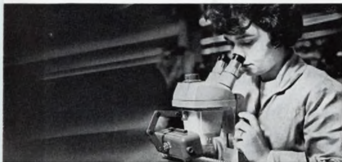
100% inspection of all components, and assemblies before sealing
