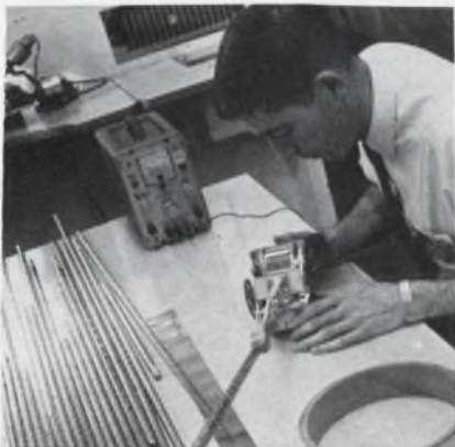
Tubular antennas, produced as flat metal strip, are unwound from drum.
