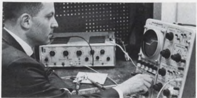
Tracing the key waveshapes. Circuit-designer Hilsenrath observes the step response of his common-emitter. By using a set of master response curves, he was able to predict performance before he built the network.
