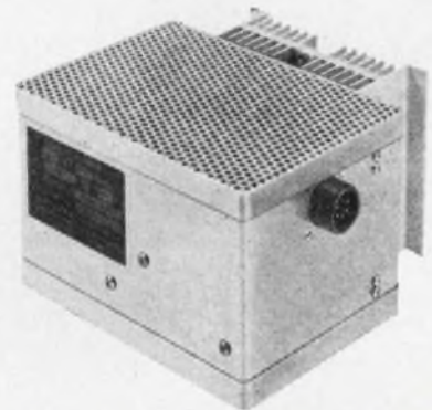
Dual output, regulated power supply. Outputs: +11 to 13 VDC @ 1.5A and -11 VDC @ 0.1A. Meets MIL-T-21200.
