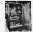
Output stations are for use at frequencies from 1 to 10 kc. Power levels to 100 kw can be handled in the smaller unit (type MFO-2) and to 500 kw in the larger station (type MFO-1). Both stations can be provided with electrically operated capacitor tap changing switches and an auto-transformer tap switch.
