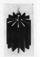
For stud-mounted transistors, rectifiers and diodes. Constructed of aluminum, the model HS 8040 is available for stud-mounted semiconductors with 8-32 to 1/4-in. pipe thread. The dull black anodized unit meets applicable MIL specs. The equipment is said to feature a very low contact resistance and has a surface area of 20 sq. in. per in. of length.
