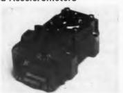
Model F2401-01A is a dc torquer-restrained device which possesses a dynamic measuring range of greater than 20 million. The element consists of a symmetrically located differential transformer pick-off and a pair of force coils mounted in common on the instrument measuring axis.
