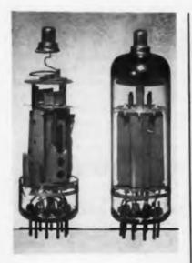
vertical partitions, which are at right angles to the plate. The effect of this is to form a number of cavities facing the cathode. The secondary electrons, ejected by the impact of the primary electrons on the plate, are for the greater part absorbed by these partitions. Secondary electrons that escape from the cavities will be forced back by the space charge formed by the beam-plate construction of the pentode.
