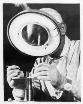
A tiny accelerometer, expected to be a key to increasing Polaris range from 1,200 to 2,500 miles, is assembled in a sterile laboratory at Sperry Gyroscope Co., Great Neck, L. I., N Y. The company is producing subminiature prototype models of the new MIT-designed devices for a smaller, lighter and more accurate missile-guidance system. The accelerometers can sense and measure changes in the velocity of the missiles in flight.
