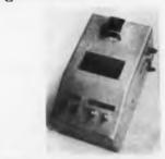
Uses palladium alloy tubing. Maximum flow rate is 100 cc per min at an inlet pressure of 50 psig and an outlet pressure of 10 psig. The unit is said to produce pure hydrogen with no measurable impurities. For complete systems, larger units are available with outputs up to 10,000 standard cu ft per hr.
