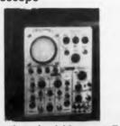
Rise time is 0.35 nsec. Type 661 shows Lissajous patterns on a 5-in. crt, in addition to dualtrace displays and signals added algebraically. The unit can expand the signal over 100 times vertically or horizontally and drive X-Y plotters or similar readout accessories. The equipment has a uniform, high writing rate at all sweep speeds over the full 8 x 10 cm display area.
