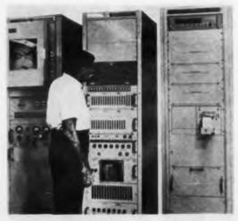
**Pulse-code-modulation** equipment is checked out at Bell Laboratories' Hillside, N. J., test site. The unit is one of three to be used in American Telephone & Telegraph Co. satellite.
