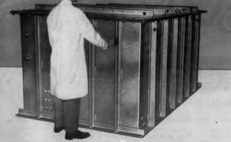
242 TON POWER SUPPLY delivers 52.5 kVA, is insulated for 70kV and is capable of withstanding heavy short circuit fault currents.
