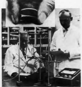
Fuel cell apparatus based on new organic ion-exchanging membrane uses basic cells about the size of a quarter that develop 0.95 v in an open circuit. Shown are co-inventors Andrew Dvarnieks, left, and Jack Bregman, of Armour Research Institute.
