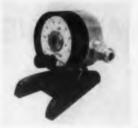
Frequency range of 0 to 3,000 mc is offered by model RT-1, variable attenuator. The accuracy of the device is  $\pm 2$  db over the entire range. Max standing-wave ratios are 1.2, input and 1.4, output. Models come in 50-, 60-, and 75-ohm impedances, with a power handling capacity of 0.5 w.
