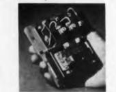
Type HRLR ac latch relays are designed for machine tool and other control uses where the control circuits must function independently of circuit or power failure. Mechanically held units feature: continuous duty coils on both main relay and latch assembly, unitized convertible poles, and electrical reliability. Relays are available with 2, 3, 4 or 6 normally open or normally closed unit poles.
