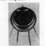
Current gain (hFE) of the 2N2060 is matched to within 10% at 0.1 ma and 1.0 ma collector current. Max base-emitter voltage differential allowed is 5 my at 0.1 and 1.0 ma. Noise figure of 8 db max is specified for both narrow and wide-band usage.
