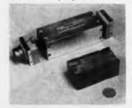
The standard MIDAS fm-fm radio telemetry system consists of a data transmitter, receiver and recorder. This solid-state unit has a dynamic signal input range of 0.02 to 20 mv. Input transducer impedance is 50 to 500 ohms and system linearity is  $\pm 1\%$  of indicator reading. Operation is 9 v dc for transmitter and 110 v ac for receiver/indicator.
