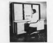
DDP-19 is a single address, parallel, binarystored program machine. The 19-bit machine uses a 5- $\mu$ sec, 4,000 or 8,000 word core memory, with additional memory units available. Memory access time is 2.5  $\mu$ sec, and read-write cycle time between memory accesses is 5  $\mu$ sec. Add time is 3  $\mu$ sec, average multiply time is 36  $\mu$ sec and average divide time, 45  $\mu$ sec.
