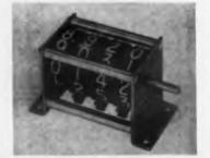
Model 3522 has large digits and is reversible. Drums and pinions are molded nylon in this 1-11/16 x 2 x 3-3/16 in. unit. The 0.420 in. high digits, on 1-7/16 in. diam drums, are either hot stamped or silk screened. The unit comes with either oilite or ball bearings.
