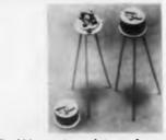
**PNP 400-mw transistors for switching and chopping** meet MIL-S-19500B specifications. Collector saturation resistance is less than 10 ohms. Units are manufactured in the 2N327A series and 2N1228 series. Leakage currents into the na range and high voltages in the reverse configuration enables them to be suitable for chopper service.
