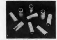
Ceramic utilized is 90-97% pure alumina. Bonding strength of the metallizing techniques used is 15-20,000 psi. Ceramic tubes can be metallized in sizes varying down to 0.080 in. ID. Ends of the tubes, which have a maximum length of approximately 8 in., can also be metallized where required.
