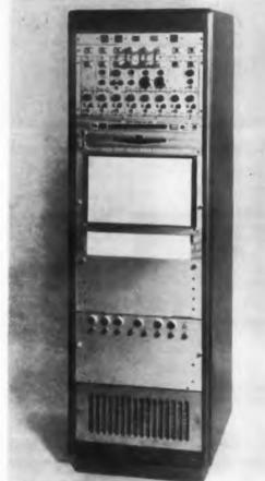
**The Tracemaster** 8-channel direct-wiring recording system.
