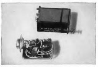
Sight amplifier module potted with RTV by the Armament and Control Section of G.E.'s Light Military Electronics Department. Used on the Lockheed CF-104 and F-104G jet aircraft, RTV provides mechanical support and vibration damping, protects unit against moisture and ozone. (Bottom photo shows module before potting.)
