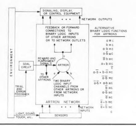
axon). The artron has 16 states and a delay capability.
