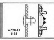
Lightweight oval or flush head stude of SAE 1010 steel, case hardened, are retained in door or panel. Five standard lengths provide for total material thicknesses from .040 to .159. Spring steel receptacle occupies minimum inside space. Weight per 1000: from 2.072 to 3.522 lbs. depending upon stud size.
