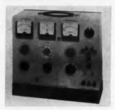
Power transistor measurements to 30 amp collector current and 300-v breakdown test potentials are possible with the Type 300 precision power transistor test set. Direct meter readings of large signal current gain,  $H_{PE}$  and collector characteristics,  $I_{CBO}$ ,  $I_{CER}$ ,  $BV_{CEC}$ , and  $BV_{CBO}$ , can be made under conditions typical of their actual applications.
