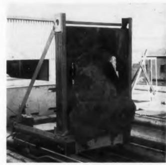
Fig. 1. In just over 1-1/2 hr, a hole was melted through this 1-in. lead shield by gamma flux of  $2 \times 10^{13} \gamma \text{cm}^2$ -sec.
