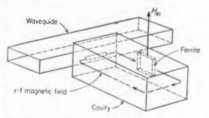
**Fig. 7.** Ferrite-loaded band elimination filter, *TE*<sub>101</sub> cavity mode.
