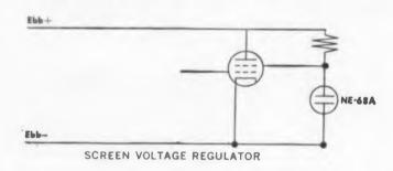
Here at last is a glow lamp with true voltage regulation specifications. Within a range of 52 to 65 volts, each individual General Electric NE-68A will not vary more than three volts even though current through the lamp fluctuates between .1 and .3 milliamps. Minimum maintaining voltage of all NE-68A's at .1 milliamps is 52 volts; maximum voltage at .3 milliamps is 65 volts.
