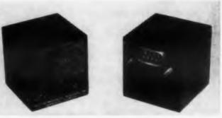
Designed for aircraft and missile fm telemetering systems, model 185C fm subcarrier oscillator is housed in a 1.5-in. cube. It accepts transducer outputs of +3,  $\pm 5$ , or  $\pm 1.5$  v and supplies a 5-v rms output into 5,000 ohms. It is available with IRIG channels 7 to 18 and A to E. Linearity is better than 0.1%. Data is translated with amplitude and harmonic distortion of less than 1% to a modulation index of 5.
