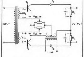
Fig. 2. Push-pull phase-sensitive circuit.
