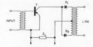
Fig. 5. Amplifier fed with pulsating current.
