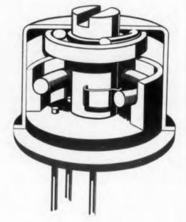
**Cut-away shows** simple construction of miniature trimming pot. Total outside diameter, including flanges, is 0.345 in. Pot is said to be one quarter the volume of conventional trimming units. Rotor screw is at top.
