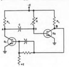
**Fig. 1.** Conventional, collector-coupled, monostable multivibrator.
