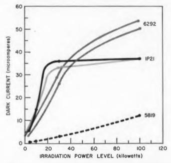
Fig. 2. In a typical transient effect, three photomultiplier types exhibit increased dark current during irradiation, return to normal afterwards.
