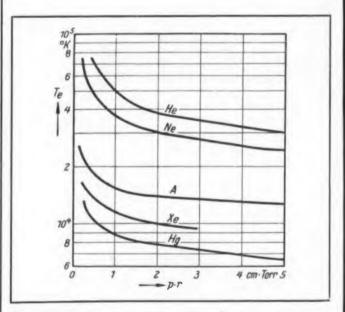
**Fig. 1.** Electron temperature,  $T_c$ , of various gasses as a function of discharge pressure-distance product (1 Torr = 1/760 atmosphere).
