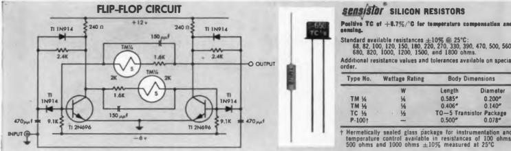
This flip-flop circuit, designed by Texas Instruments, uses sensistor® silicon resistors in the cross-coupling network to compensate for increases in hFE with temperature. At 125°C, it resolves 100 musec input pulses arriving at a 5 mc rate whereas a fixed resistor version was limited to 3.6 mc. In addition, at +125°C the circuit will operate at a resolution rate greater than 5 mc if the input pulse can be greater than 10 volts when the pulse width is decreased from 100 musec.
