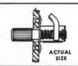
A new, minute version of the widely used Southco Adjustable Pawl Fastener. 1/4 turn opens, 1/4 turn locks. Turning tightens to compress gasket, resist vibration. Supplied assembled for quick installation. Cadmium-plated steel. Requires only 15/2 inch inside space. Weight per 1000: 11 lbs. Also available for use with your knob.
