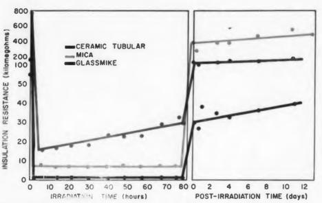
Fig. 3. Post-irradiation recovery of insulation resistance is illustrated for three capacitor materials.
