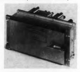
In model 100 diode function generator, a hole pattern in a punched card replaces the setting and adjusting of potentiometers. Functions are composed of 20 contiguous line segments. Slopes range from 0.005 to 10.16 v per v. Absolute accuracy is 0.1%, long-term repeatability is 0.02%, input impedance is 1 meg. output power is  $\pm$  100 v into 10 K, and frequency response is from de to 10 kc.
