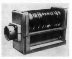
The model 602 electro-mechanical programer is designed for programing on-off functions. It will handle 30, 2-amp circuits. Time range is 60 to 5,000 sec. Accuracy is 1%, 3% or 5%. Units include reset, solenoid latching, and a positive zero-time indicator.
