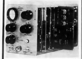
The Oscilloscope consists of 11 parts, the case, guide rails, "mother" board, 5 circuit cards, plug-in front and rear panel assemblies.
