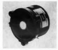
The V-line vane-axial blower, 2-in. in diameter and 1.5-in. long, delivers 64 cfm at an SP of 0 and 3 in. at shut-off in the two-pole version. It requires an input of 37 w and has a temperature rise of 40 C max. In the four-pole design, rated at 11,000 rpm nominal, input is 8 w at 0.08 amp. Temperature rise is 15 C.
