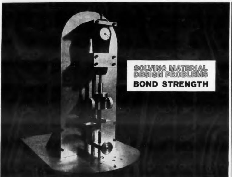
The trick is in the adhesive. CDF's Di-Clad® printed circuit boards are tested for bond strength in this precision machine.
