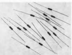
Types 1N625 through 1N629 diodes are fast recovery units providing 400,000 ohms in 1 μsec. Types 1N482 through 1N485 diodes are high-conductance units with a 100-ma max avg forward current at 1.1 v. The devices are designed for airborne and industrial computers. Shock and vibration resistance exceeds MIL-STD 202A.
