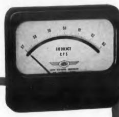
These highly accurate, dependable Frequency Meters by Airpax, are completely self-contained. Connection is simple. Two meter terminals protruding from back of case connect directly across 100 - 130 volt source. Airpax MAGMETER frequency sensing circuit is insensitive to voltage variations, responding only to frequency changes.
