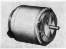
Type SS250 synchronous motor is designed primarily for industrial uses. It has a torque of 250 oz-in. and a constant speed of 72 rpm. A dc voltage applied to its field windings converts one revolution of the motor shaft into 200 precise steps. Ratings are: input, 120 v, single phase, 40 to 70 cps, 0.6 amp max at 60 cps; 72 rpm output at 60 cps.
