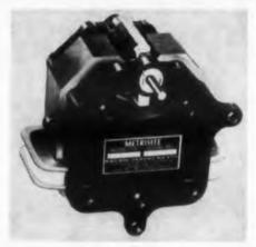
Type 34A rugged, angular motion Metrisite transducer converts angular motion of up to  $\pm 40$  deg to voltage outputs with 0.25% linearity. The device has a negligible reactive force. It measures  $3 \times 2.5/8 \times 1.7/8$  in. and weighs 20 oz.
