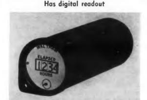
Type WT-3 elapsed-time indicator with digital readout weighs 3.75 oz, measures 1-1/16 in. OD x 2-3/4 in., and operates at 360 to 440 cps with a 2.5-w maximum power input. The digital presentation runs to 9,999 hr and the numerals are 5/32 in. high. Jewel bearings are used.
