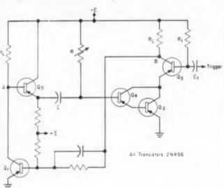
Fig. 4. This circuit gives high duty cycle with proper R value and maximum voltage swing.
