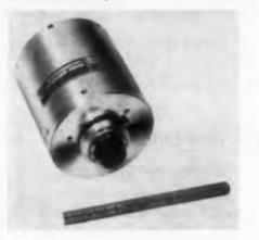
Model VM-1030 Delay Line features a continuous range of delays from 3 to 500 µsec with an accuracy of  $\pm 0.5$  µsec. It has an optimum pulse input of 1 µsec and can be supplied with an impedance range of 50 ohms to 4 K. Insertion loss at the end of the range is 56 db and the maximum number of pulses per second is 300 kc. The unit is 4.406 in. in length with an OD of 3.398 in. Total weight is 2 lb.
