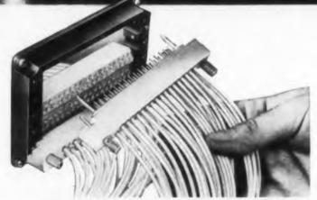
HYFEN-type connectors like those used in the "vest pocket" air defense system have pins and sockets tool-crimped on cable ends, snap-locked in inserts with wide range of configurations. HYFEN and STAPIN inserts are mounted in panels as required.
