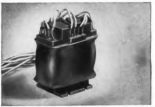
High-voltage, high-altitude transformers from Laboratory For Electronics, Inc. are encapsulated with General Electric RTV to meet MIL-T-27A specs. This prevents flashover at maximum ratings of 2200 volts rms and 80,000 feet. General Electric RTV was selected for its good heat transfer, low viscosity and mechanical strength.
