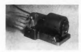
This machine is designed for stripping Form-var insulation from AWG 50 copper wire and enamel from No. 56 Nichrome. It uses two conical Grade 89 fiberglass wheels as abrasive. Designated Model 89 TwinCone wire stripping machine, the device is suitable for bench mounting and can strip wire leads to within 1/16 in. of component bodies.
