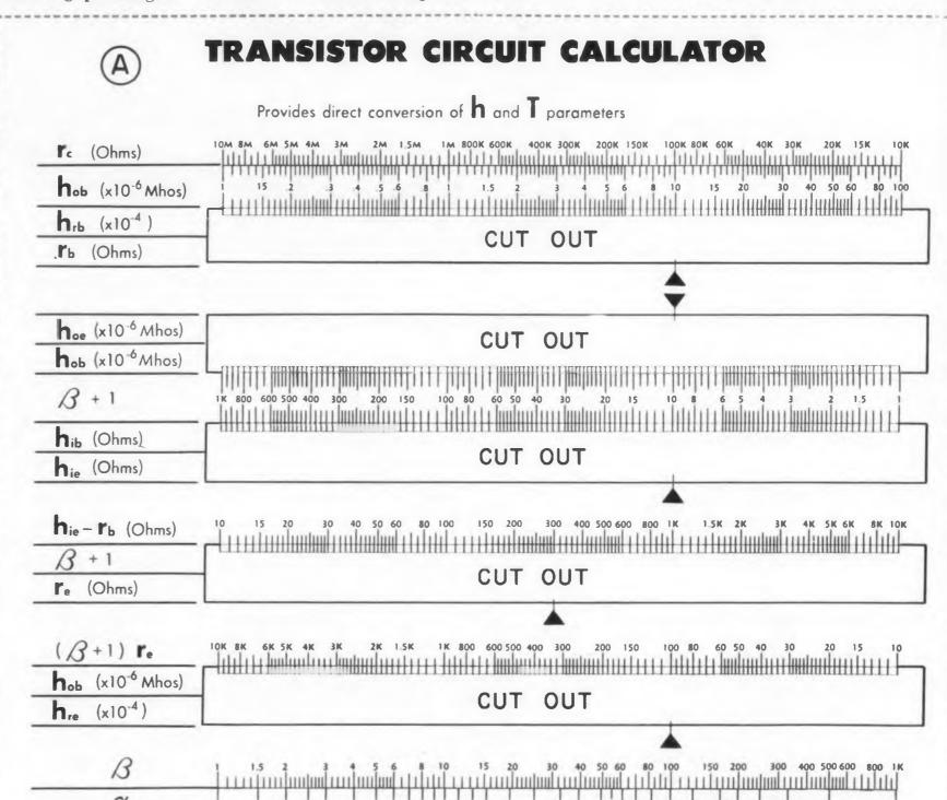
Next, center the A scale on one of the cardboards, and paste it in this position. Rubber cement is recommended. With a sharp razor blade or Exacto knife, trim along the outside guide lines, and then cut out the areas indicated, including those portions of the scales lying within. The A scale is now prepared.
