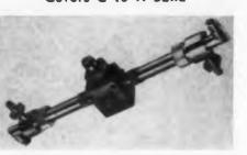
This C to H band balanced mixer uses a varying signal-local oscillator system that does not require very narrow-band, electronically tuned filters. The conversion loss is 6 db over 5200 to 5800 mc; vswr is less than 3:1 over the local oscillator band of 3900 to 4500 mc and less than 1.7:1 over the signal frequency band. All components following the mixer are designed for use at a single frequency rather than a band of frequencies.
