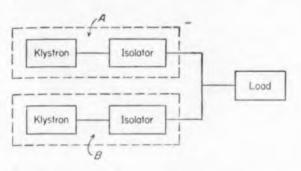
Fig. 2. Use of isolators in isolating sub-systems.
