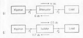
Fig. 1. Load isolation using attenuator and isolator.
