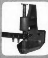
Using planning sheets as masters, terminals and sockets are swaged and eyeleted securely into place on pre-punched terminal cards.
