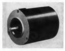
This self-orienting, synchronous motor insures synchronization of the rotor within ±5 deg with respect to the rotating stator field. No de excitation of the rotor is required. Motor is two phase, 60 cps, 115 v ac; synchronizing pull-in torque is 0.50 oz-in.; fall-out torque is 0.65 oz-in. Unit measures 2 in. long with a 1-3/4 in. diam and weighs 10 oz. Units designed for 400 cps are also available.
