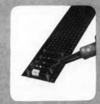
Components are snapped into terminal jaws, ready for soldering.
