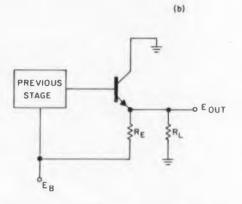
Fig. 2. With this circuit, the output voltage will clip at a value independent of the input voltage (for  $|E_{in}| > |E_b|$ ).
