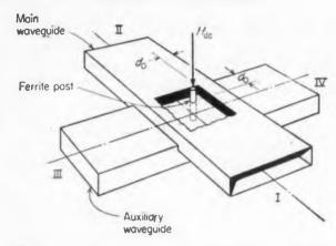
Fig. 5. Crossguide ferrite directional coupler.
