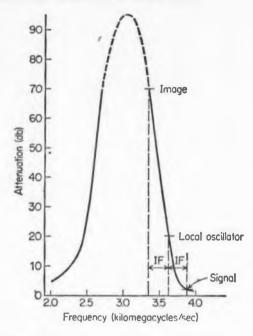
Fig. 8. Ferrite resonance absorption curve showing application to receiver image re-
