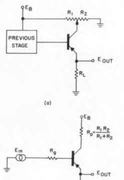
Fig. 1. Output voltage of this pulse amplitude limiting circuit (reprinted from Ideas for Design, ED, April 27, 1960, p 120) is still a function of the input voltage (see
