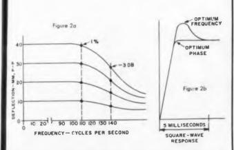
Frequency and amplitude response are shown in Fig. 2a, while Fig 2b depicts the square-wave response for optimum frequency and optimum phase monitoring.
