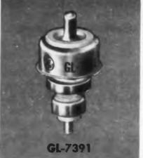
This is a Class C version of tube type GL-6299. It operates up to 6000 mc. Its power output is 65 mw at 5400 mc. Moreover, its power autput is greater than 0.5 watts at 500 mc. This new, metal-ceramic **UHF-SHF** low-power triode features conduction cooling and has a grounded grid.
