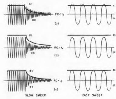
Fig. 2. Oscilloscope patterns for different values of capacitor C. In practice R is held constant and C is varied, until rectified and alternating waves are lined up as in pattern (c).
