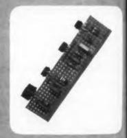
Terminal cards make neat component sub-assemblies, organized function by function into unit planes of circuitry.
