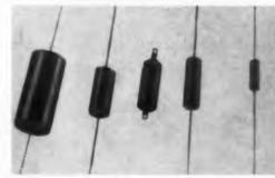
The HI-Lar mylar film capacitors are for high-altitude space probe applications. Other uses are in instrument-quality recorders, pulse networks, and computers. The line is available in increments of 100, 200, 400, and 600 v and in ranges of 0.0047 to 1 µf. Temperature range is —55 to +125 C, dielectric absorption is 0.1%, and retrace stability is less than 0.2%. Dissipation factor is less than 0.5 at 25 C and 100 cps.
