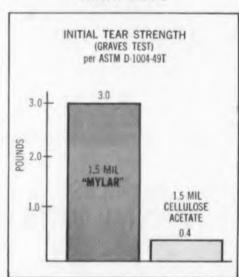
The superiority of "Mylar" can make an important contribution to the reliability of your magnetic-tape system. Ask your magnetic-tape supplier to recommend the specific tape of "Mylar" for your needs.
