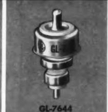
This derivative of type GL-6299 operates up to 3000 mc, and is notable for its high spike resistance capabilities. The tube is unilaterally interchangeable with type GL-6299. Only recently announced, this sturdy, UHF, low-noise and low-power triode features a grounded grid and conduction cooling.
