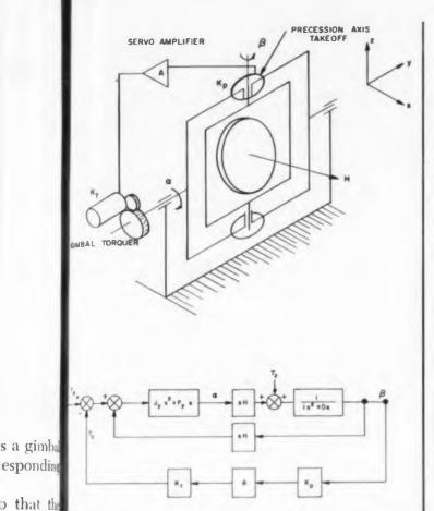
Fig. 1. Typical single axis platform with rate integrating gyros. The block diagram is used to analyze the platform motion.
