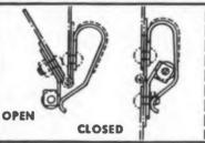
Nothing shows on outside of equipment. Clean appearance. Pull open, push shut. Held firmly in both positions by spring tension. Steel spring cam, brass roller. Maximum moment: 3/4 in. lbs. Spring and cam locations interchangeable. Weight per 1000: 14 lbs.
