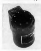
This potentiometeric accelerometer uses flexures and dual seismic masses. The seismic mechanism has no rubbing parts. Cross-talk is kept at a minimum. Linearity is  $\pm 2\%$  from -55 to +70 C. Error due to vibration is less than  $\pm 0.03$  in. displacement at 10 to 55 cps and less than 6% under  $\pm 10$  g at 55 to 500 cps.
