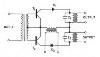
Fig. 4. Phase-sensitive circuit feeds load through twin transformers.
