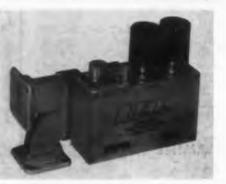
The MMX-6 matched X-band microwave receiver head end assembly covers the 8.5- to 9.6-kmc range with a maximum noise figure of 7.5 db. It has a typical noise figure of less than 7 db, an if bandwidth of 8 mc and an if gain of 25 db. The MMX-6 is electrically similar to the MMX-2.
