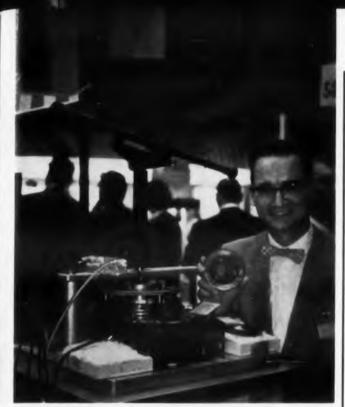
**Phasolver** (see p 19) measures angles to fraction of a second of arc, said Telecomputing Corp. Project engineer Ray Dunwell.
