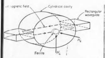
**Fig. 6.** Ferrite-loaded band pass filter, *TE*<sub>111</sub> cavity mode.
