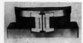
Model DTH 2132 digital magnetic-tape head is a 32-track interlaced unit for 1-in. tape. The gap length of the head is 10  $\mu$ in., allowing its use at high-bit densities. The unit is shown mounted on type TG tape slot guide. A precision unit, the tape guide virtually eliminates tape skew and scrape-flutter.
