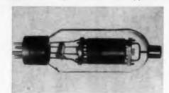
Type 572 triode is a ruggedized, one way replacement for the prototype 811A in most applications. Ruggedized construction includes hard lass envelope, heavy-duty tungsten lead wires, non-frangible filament and enclosed getter traps. The manufacturer claims the 572 has a 50% increase in plate dissipation over the 811A. United Electronics Co., Dept. ED, 42 Spring St., Newark 4, N.J.
