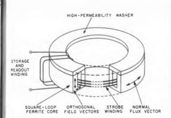
In this modified Biax element, orthogonal field is not uniform throughout cross-section.
