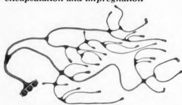
General Electric silicone rubber used extensively by Aerojet-General Corp. for the Titan ICBM's propulsion-system wiring harness. Breakouts and junctions molded from G-E RTV, wiring is silicone insulated. jacketing is high-strength G-E silicone rubber - all chosen for their stable insulating properties, resistance to temperature extremes and weathering, and stability in storage for many years.
