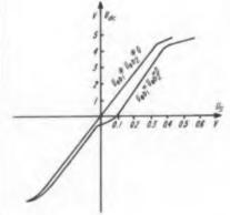
Fig. 3. Dependence of the dc load voltage of a push-pull phase sensitive circuit on the signal, for different (but constant), emitter - base voltages  $U_{cb}$ .
