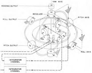
Fig. 2. Three-gimbal stable platform consists basically of three single axis systems to control roll pitch and yaw. An additional azimuth coordinate resolver in also required.
