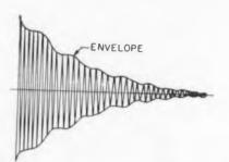
Fig. 3. This oscilloscope (slow sweep) pattern results when tuning fork is unbalanced (tines are at two different frequencies).
