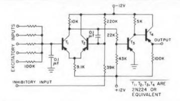
This electronic neuron, developed at Bell Telephone Laboratories is a four-transistor device with variable threshold capable of an integrating time constant of 2 msec and a refractory time constant of about 10 msec. These values approximate those of biological neurons.
