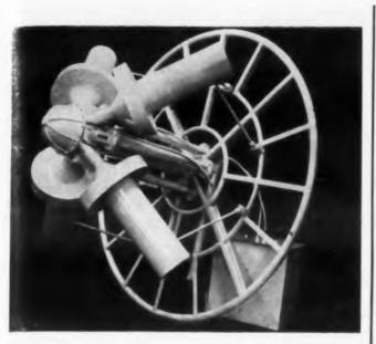
Feed system for Courier tracking antenna. Dome at front houses spinning dielectric lens which scans signal to provide error data for automatic tracking. Feed path for VHF is through the four extended arms; UHF is fed through waveguides down center of unit. Antenna and tracking gear is by Radiation, Inc., Melbourne, Fla.
