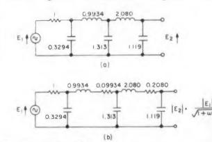
Fig. 3. A low-pass, 5-pole Butterworth network with coil Q's of 10 designed with the aid of Table 13. The lossless network (which does not have the desired response) is shown at (a). Adding the indicated losses for the proper response gives the network in (b).
