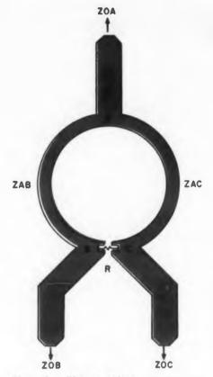
**Fig. 1.** The stripline directional coupler with a 3-db insertion loss shown here is designed about a simple path-length difference.
