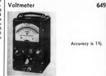
Type 300-G electronic voltmeter has an accuracy of 1% over the meter scale from 1 mv to 250 v and over the band of 20 cps to 20 kc. Accuracy is better than 2% up to 1,000 v and from 10 cps to 250 kc. The instrument covers 1 mv to 1,000 v in six decade ranges. It has a 5-in., mirror-backed scale.
