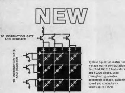
n-stage matrix configuration. Fairchild 2N1613 transistors and FD200 diodes, used throughout, guarantee acceptable leakage, switching speed and conductance. values up to 125°C.
