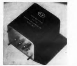
The Series F bandpass filters, available in 90-, 150- and 180-cps models, have bandwidths of 8, 11 and 12 cps respectively a 1 db down. Insertion loss, input and load impedances are the same for the three units. The instruments are designed for navigational aids, instrument landing systems. receivers, control units, monitors and associated test instruments. Units are hermetically sealed in 3 x 3-1/2 x 3-13/16 in. metal cases. Ambient temperature range is -20 to +60 C.
