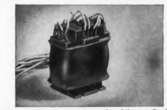
High-voltage, high-altitude transformers from Laboratory For Elec-tronics, Inc. are encapsulated with General Electric RTV to meet MIL-T-27A specs. This prevents flashover at maximum ratings of 2200 volts rms and 80,000 feet. General Electric RTV was selected for its good heat transfer, low viscosity and mechanical strength.
