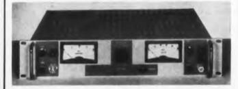
The model LQ35-2A dc power supply has an output voltage of 0 to 35 v at 0 to 2 amp. Regulation is 0.005% or 1 mv, whichever is greater, per 10% of line change at any rated load. Load regulation is less than 5 mv from no-load to fullload. Ripple is less than 50 usec. Line input is 105 to 125 v ac, single phase, 60 cps. Panel measures  $3-1/2 \times 19$  in.; chassis is 17-7/8 in. deep.
