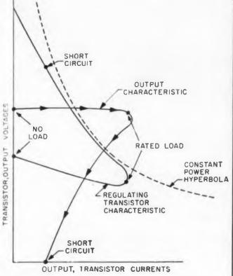
Current-voltage characteristics are shown for the output of the supply and for the regulating transistors. Arrows show direction of operation as loading increases from no load to short circuit. (Curves are to scale and apply approximately to each unit.)
