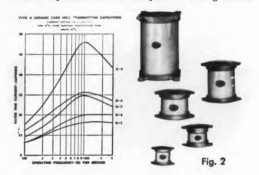
by the rf field. Because these factors are so important, transmitting capacitors are rated in rms current and peak working volts. They are usually potted in a material that has a high thermal conductivity and packaged to have a large surface area. Sangamo's Types E, F, and G are examples of high rf current application capacitors. Figure 2 shows, for example, the relative size and current-carrying ability of Types G1, G2, G3, G4 and G5.
