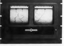
•Varian offers rack mounted versions too—either singles or twins. The latter is pictured, showing how four channels of recording can be fitted within the 19-inch width of a standard rack.
