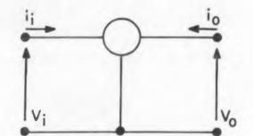
Fig. 1. Generalized transistor circuit.
