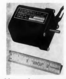
This solid state, subminiature servo drive system has a volume of 1.75 cu in. and delivers a torque of 2 in.-lb from a change of 0.001 v. Actuator arm speed is 270 deg per sec. The device consists of a servo amplifier, a precision gear train and a high-torque servo drive motor. Electrosolids Corp., Solidtronics Div., Dept. ED, 14751 Keswick St., Van Nuys, Calif.
