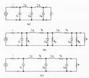
Fig. 1. A 5-pole, low-pass network: (a) as a lossless network; (b) as a uniformly lossy network in which dissipation of the reactive elements is represented by conductances in parallel with capacitors and resistors in series with inductors. Here,  $r_i = dL_i$ ,  $g_i = dC_i$  (c) as a lossy-L network in which losses are concentrated in resistors in series with the inductors. Here,  $r_i = dL_i$ .
