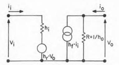
Fig. 3. Electrical equivalent of generalized circuit derived from flow graph of Fig. 2.
