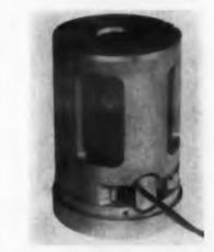
Type PHM pyrotechnic free gyro is for one-time use in short range missiles. Measuring 4.5 x 2.75 in. and weighing about 800 g, the unit stands 100 g shock. It has 2 deg of freedom. Active gyro life is 3 min with an average drift of 1 deg per min.
