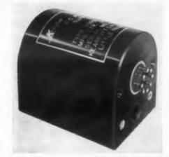
An output of 29 v dc at 300 ma, filtered and unregulated, and two isolated ac outputs rated at 4 w and 0.5 w respectively are provided by the model H3900-01 power supply. The do source is suitable for transistorized amplifiers and small servos. Input is 115 v, 400 cps. The device can be used to circumvent noise and severe transient voltages in 28-v dc lines of aircraft and missiles. Units, weighing 28 oz, are potted and sealed.
