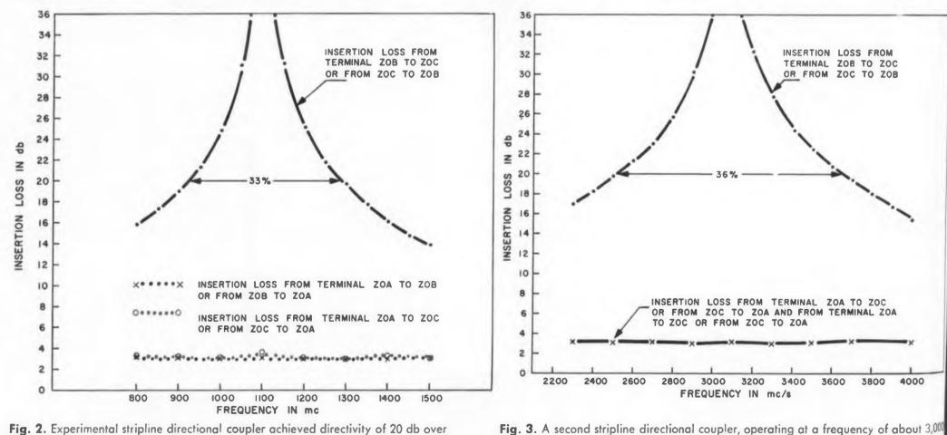
**Fig. 2.** Experimental stripline directional coupler achieved directivity of 20 db over a 33 per cent frequency band at 1,100 mc, with an insertion loss of 3 db.
