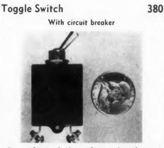
By combining both toggle switch and circuit breaker in this miniature unit, the need for replaceable fuse, fuse holder, and switch is eliminated. Weighing less than 50 g, the unit is suitable for use in radio, aircraft, and industrial electronic equipment. Its dielectric strength is over 3,500 v. Called the 3100 series, the device can interrupt circuits carrying up to 5,000 amp at 120 v, 60 cps. Units have current ratings of 5 to 50 amp.
