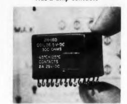
Type JH-18 6 pdt miniature relay has 0.2 in. grid spacing, 2-amp contacts, and occupies less than 1 cu in. of space. It weighs less than 1.8 oz. Standard coils include nominal voltage ratings of 6 to 115 v dc with a power rating of 2.5 w. Dielectric strength is 1,000 v rms at sea level or 750 v rms across open contacts. Insulation resistance is 1000 meg min. The unit stands shock to 50 g and vibration of 28 to 2,000 cps at 20 g or 5 to 28 cps at 0.5-in. double amplitude.
