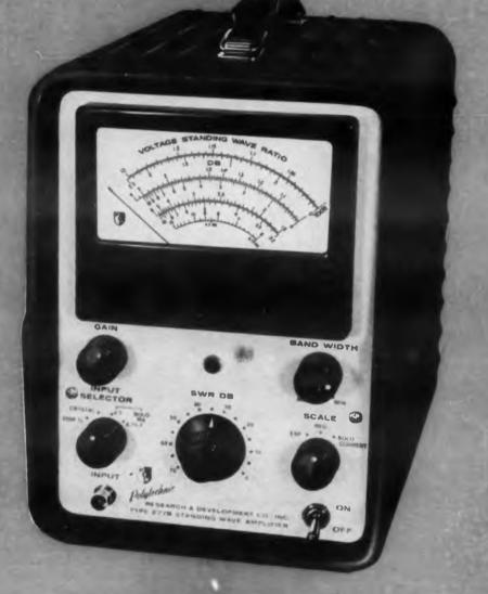
The new portable PRD 277-B Standing Wave Amplifier is designed to meet the present and future needs of microwave test laboratories. Due to its extremely low inherent noise, 0.007  $\mu$ v, weak signals which once were undetectable by conventional instruments can now be measured. Attenuation in 5 db steps combined with 4 VSWR scales and a large meter permit VSWR measurements to be made with maximum resolution and accuracy.
