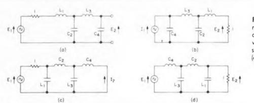
with coil Q's of 10, then we use the lossy-L tables, and enter the row of Table 13 for which d = 1/Q = 0.10. This gives the design of Fig. 3a. It is important to realize that this network *does* not have the desired response. This is obtained only by adding the indicated losses, as shown in Fig. 3b.
