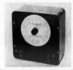
Model W-2 impedance analyzer is designed for precision measurement of polar parameters, phase angle and ohmic values of impedance. It computes and directly indicates phase angle as well as its sin, cos, and tan, power factor, Q, and D. Measurements can be made at the actual operating voltage and frequency of the component being tested. Accuracy is 1% from 60 cps to 12 kc, impedance measurements can be made to 1 meg.
