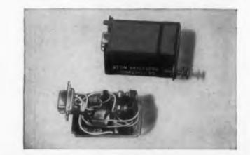
Sight amplifier module potted with RTV by the Armament and Control Section of G.E.'s Light Military Electronics Department. Used on the Lockheed CF-104 and F-104G jet aircraft, RTV provides mechanical support and vibration damping, protects unit against moisture and ozone. (Bottom photo shows module before potting.)
