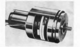
This size 23 precision servo motor-generator designed for application as a rate servo and o provide damping in very high gain systems. Motor stall torgues are available from 5.5 to in.-oz. No-load speed is 9,000 rpm. Generator characteristics include 2.9 v per 1,000 rpm and linearity of 0.2% to 3,600 rpm. The unit is wailable with either a plain or pinion shaft. Kearfott Div., General Precision Inc., Dept. ED, 1150 McBride Ave., Little Falls, N. J.
