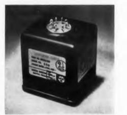
Developed for 115-v, 400-cps servo systems sed on aircraft and missiles, this solid-state mplifier drives standard size 11 or smaller 40-v enter-tapped servo motors. It can also be used operate 40-v motors in larger frame sizes where the 3.5-w output is adequate. The unit has gain stability of  $\pm 2$  db over an operating mperature of -55 to +102 C and operates with only slightly reduced gain at +125 C. Nornal power gain is 90 db max with no feedback 70 db min with feedback.
