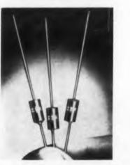
This series of miniature silicon diodes are diffused-junction units rated at 750 ma. Reverse current is 200  $\mu$ a, surge current rating is 50amp peak for one cycle, and forward voltage drop is 0.92 v. Designated types X5A2, X5A4, X5A5, and X5A6, the units have piv ratings of 200, 400, 500, and 600 v. Operating temperature range is -65 to +130 C. A typical unit measures 0.29 x 0.2 in., not counting leads.
