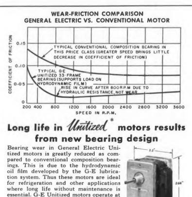
sound levels 25% below conventional motors, and their starting characteristics are excellent even at low temperatures. \* Trademark of General Electric Co. FREE Write to Section 727-02, BULLETIN Schenectady 5, N.Y.
