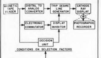
Cartographatron processes traffic data from magnetic tape to give visual display of traffic density. Decision unit is programed to select only those trips required for a particular study. Origin and destination of each trip is then plotted on the cathode-ray tube. If required, the two points can be connected by a trace.
