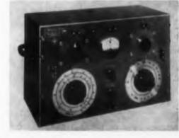
The model 385 general-purpose impedance bridge is a portable, self-contained, direct-reading unit which contains a Wheatstone bridge (ac or dc) with a range of 0 to 1 meg, a modified capacitance bridge with a 0 to 100  $\mu$ f range, or an inductance bridge with a range of 0 to 100 h. The instrument provides for tests at 1 kc as well as at dc. External signals from 60 to 10,000 cps can be introduced. A separate oscillator-amplifier accessory is available.
