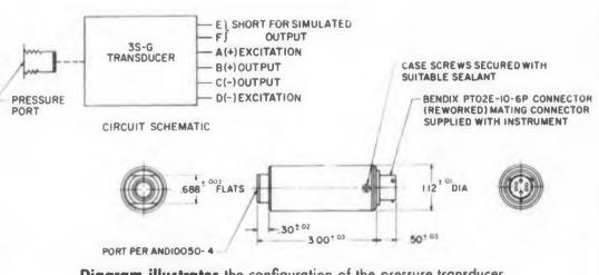
**Diagram illustrates** the configuration of the pressure transducer, and transducer excitation and output.
