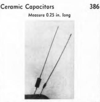
The Ceramin ceramic capacitors measure only 0.25 in. long without leads. Units having a diameter of 0.098 in. are for capacitances of 47 to 560 pf and units with a 0.125-in. diameter, 680 to 1.200 pf. These barium-titanate units are tuned to a tolerance of  $\pm 5\%$  up to 125 C or 10% up to  $\pm 150$  C. They comply with applicable portions of MIL-C-11015A and EIA-SMC-1 specs.
