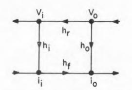
Fig. 2. Flow graph for generalized transistor circuit of Fig. 1.
