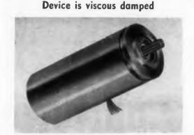
A size 8 servo motor, type 5702-03 is an adjustable viscous damped unit for feedback damping applications. The unit is 1-3/4 in. long and weighs 2 oz. Damping, gain and no-load speed are adjustable. Rotor moment of inertia is 0.65 g-cm<sup>2</sup>; stall current is 0.113-amp fixed phase and 0.077-amp control phase; stall power is 2.4 w per phase; stall torque is 0.2 oz-in. min. Housing is bright finish stainless steel.
