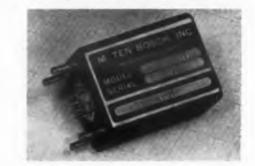
Model 1805-0100 amplifiers provides a transistorized compensating lead network for 400cycle servo systems. Quatrature rejection of the unit is 20:1 or better. Input impedance is 10 K, output impedance is 2 K. Dynamic voltage gain is 4. Power source is 28 v dc and 115 v, 400 cps. The unit is hermetically sealed and meets MIL-E-5400 specifications. It measures 1-3/16 x 1-11/16 x 2-5/8 in. and weighs 7 oz.
