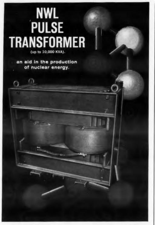
The unit illustrated is the largest transformer manufactured by NWL. It can be made in either air, air-blast or oil-filled versions. The pulse transformer has an output of 10,000 ampere pulses at 1000 volts. The approximate weight is 11,000 lbs. This transformer is typical of the many special units currently being produced by NWL. Pulse transformers can be manufactured up to 200 KV and up to 50,000 KW peak power.
