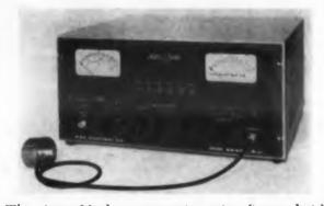
The Auto-Node automatic noise figure bridge is designed to obtain noise-figure meter displays for making noise-figure adjustment. Useful frequency range is 2 to 2000 mc. Sine-wave temperature-modulation is 10 cps with temperatures from 300 to 400 K. Noise-figure stability is better than 3.5 db and the gain is sufficient to raise the input noise to 10 v after final detection. The bandwidth is 2 mc and center frequencies can be 30, 60, or 70. The accuracy is 0.2 db for gain or loss measurements.
