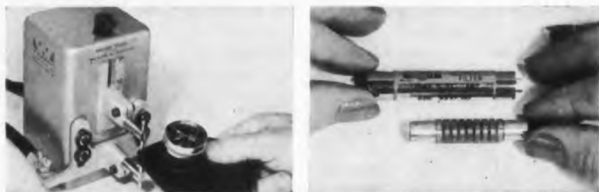
Weldmatic pressure gage reads firing force...calibrated from 0 to 50 lbs., insures exact weld pressures from job to job. (Right) Welded filter cartridge and completed miniaturized Collins filter.
