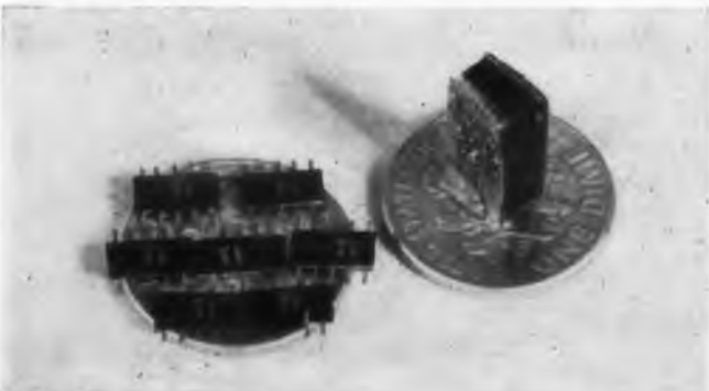
Solid-circuit added package developed by Texas Instruments for American Bosch Arma is a combination of seven individual semiconductor networks.
