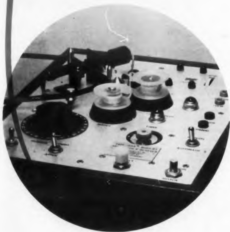
Fig. 1. Mechanism of automatic tape indexer.
