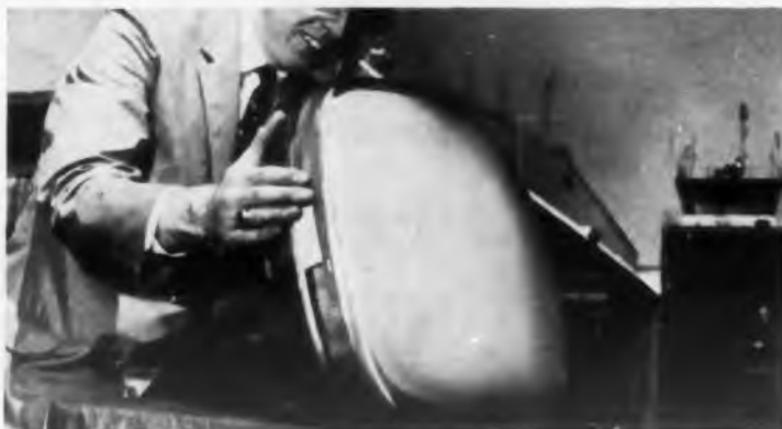
From G.E.'s CRT Development Laboratory came the GL-4619 21-inch, closed-circuit TV monitor tube, which provides more than 1000-line resolution in critical airport operations.
