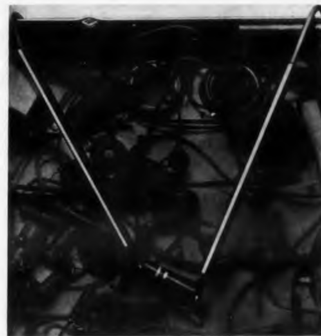
Fig. 1. Stripes on the probe's handle make locating it easy against a background of varicolored elements.
