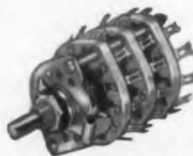
Series 275: 1/8" diameter Rating: 2 amp. at 15 VDC, 150 ma at 110 VAC Breakdown: 1500 V. R.M.S. Up to 23 positions/section
