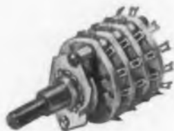
Series 20: 1/8" diameter Rating: 2 amp. at 15 VDC, 150 ma at 110 VAC Breakdown: 1500 V. R.M.S. Up to 12 positions/section
