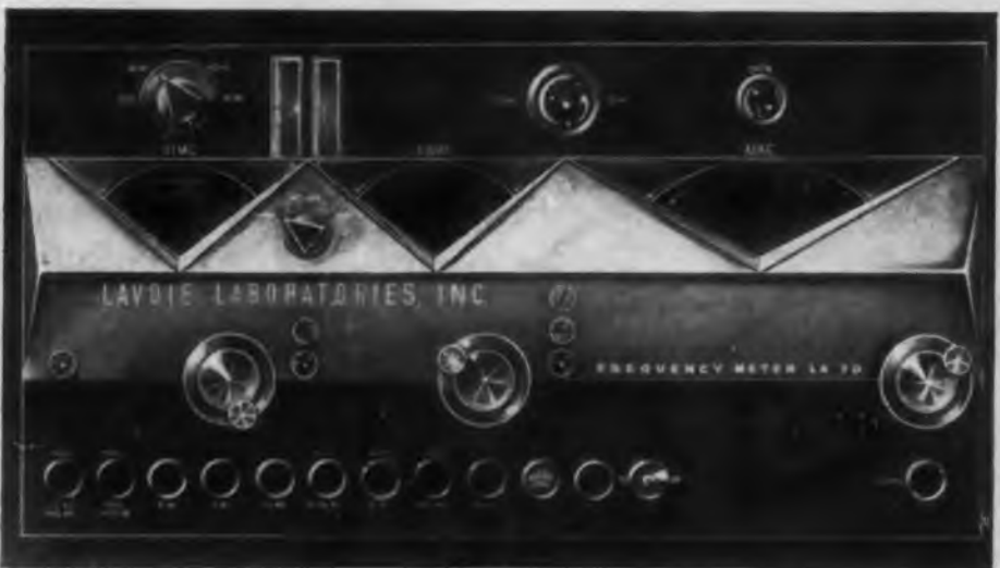
Fig. 3. An alternate redesign proposal emphasizes vertical separation of functions by means of color areas.
