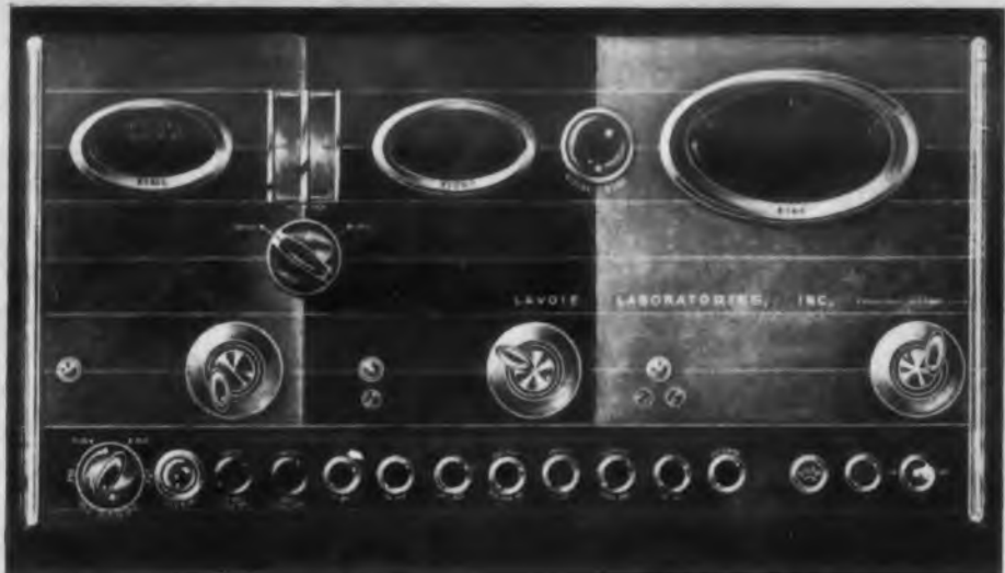
Fig. 2. A study revealed that pie-cut openings placed in a horizontal plane reduced time and errors.
