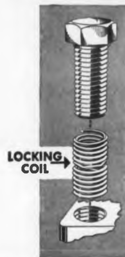
Principle of Heli-Coil Screw-LOCK Insert. Locking center coil grips internally, holds screw firmly
