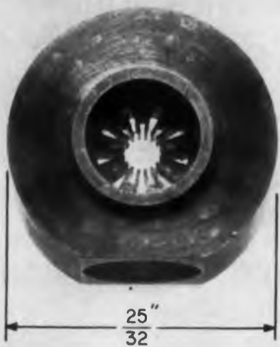
Tiny anode block , only 25/32 inch in diameter, employs sunburst cavity structure.
