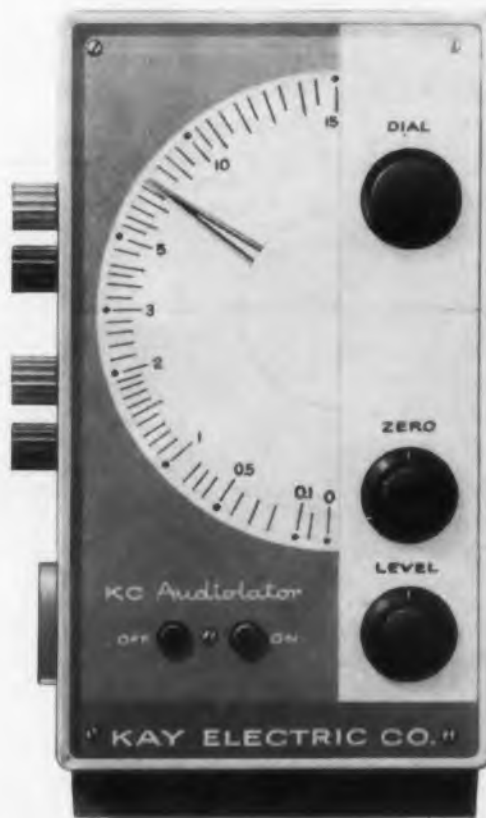
Fig. 6 (a). (left) A delicate touch and a tiny hand are required to vary the frequency due to poor dial drive placement.
