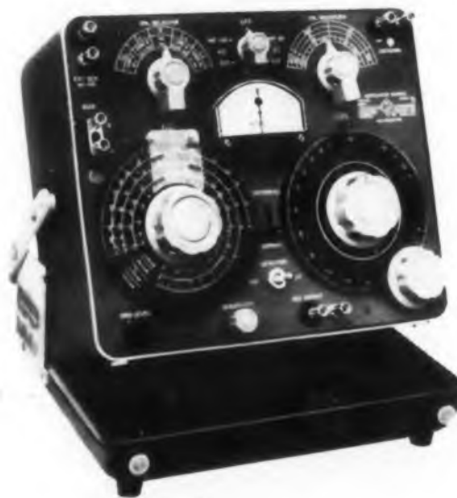
G-R's Type 1650-A includes all the best features of the 650 and higher accuracy and greater convenience in use.
