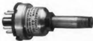
VTP 6343 THERMOCOUPLE GAUGE TUBE Fast response; less than 0.1 second! Pressure range: 0.1 to 1000 microns. Ruggedized all-metal construction. Useable for leak detection on vacuum systems as well as absolute pressure measurement.
