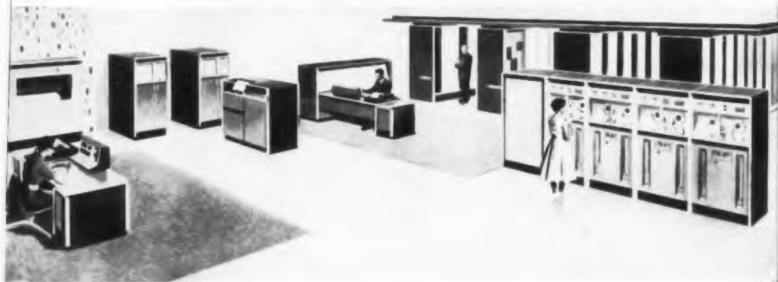
An artist's view of the Larc (Livermore Atomic Research Computer). This modern machine adds or subtracts a quarter of a million 12-digit decimal numbers per second.
