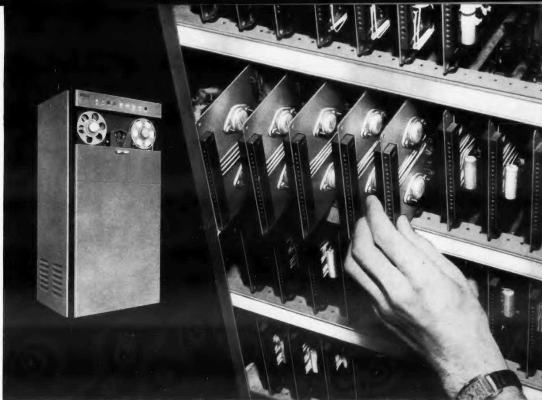
Exposed view of plug-in panels shows battery of Tung-Sol 2N459 power transistors in National's 370 High Speed Paper Tape Punch.
