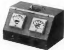
VTP TC-43-1 THERMOCOUPLE GAUGE CONTROL Dual meter control. Indicating meters for heater current and system pressure. Rotary switch permits selective measurement of pressure at any one of four separate measuring points.
