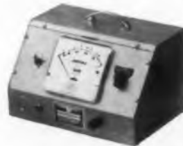
VTP PGC-25-01 DUAL RANGE PHILIPS GAUGE CONTROL Simple, inexpensive and rugged Philips gauge (cold cathode) control measures pressures in two ranges: (1) from 25 microns to 0.1 micron, (2) from 0.11 micron to 0.01 micron.
