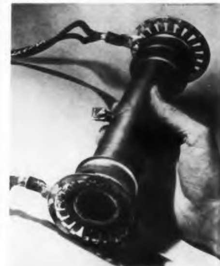
Thermionic generator developed by RCA and Thiokol fits over flame tube of solid-propellant rocket engine and converts rocket heat to electric power.
