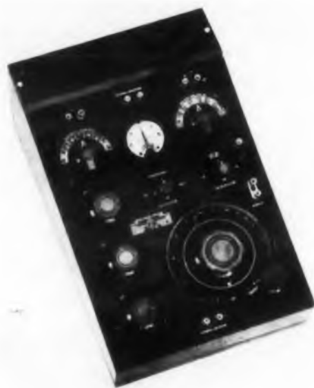
General Radio's Type 650 Impedance Bridge has remained virtually unchanged for almost three decades.
