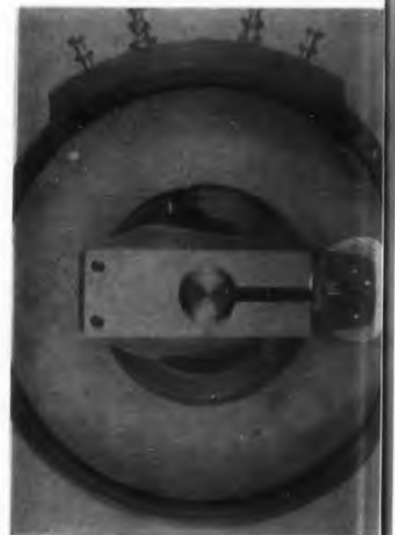
A rolling pressure piece increases the reliability of the potentiometer.
