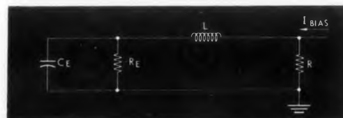
Fig. 2. Simplified equivalent circuit of the microwave tunnel diode oscillator.
