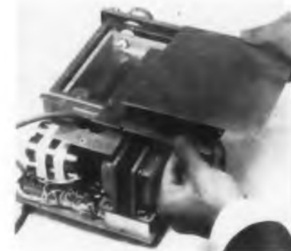
Unbuttoned, precision voltmeter shows nesting of relative-coupled amplifiers. Note concentric input jack.
