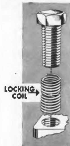
Principle of Heli-Coil Screw-LOCK Insert. Locking center coil grips internally, holds screw firmly
