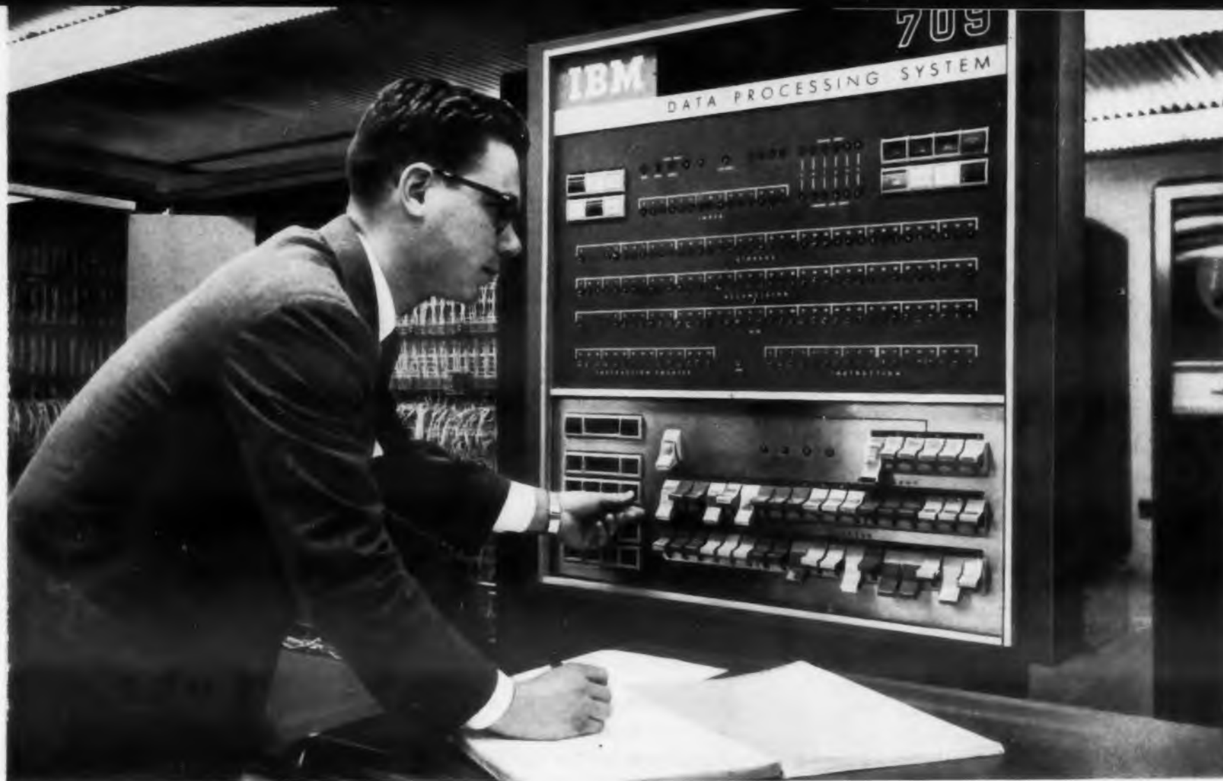
Programmer makes operational check from "driver's seat" of IBM 709 Data Processing System — the most up-to-date system utilizing electron tubes.
