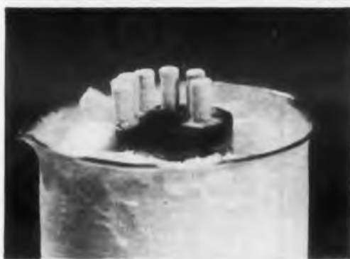
AT MINUS 50°C. aluminum pegs set at varying distances from rim of cake of "SCOTCHCAST" Flexible Resin are so cold they collect moisture in the form of frost—yet resin is unaffected and shows no sign of cracking.
