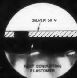
Enlarged section of Elasta clamp's inner cartridge.
