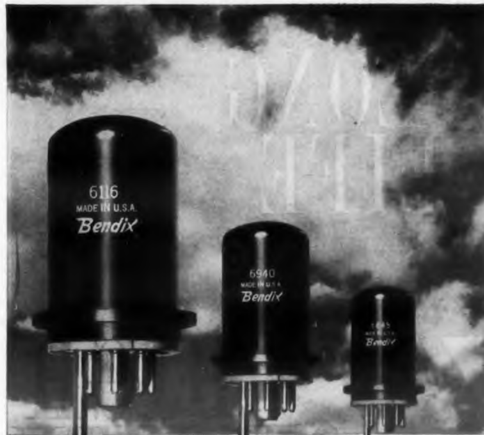
The 6116/TE-39 ruggedized Reflex Klystron thermally tunes a band of 8500 to 9660 MC by means of a diode within the vacuum envelope. Tuning speed over the required frequency range is 0.7 seconds min. to 3.0 seconds max.
