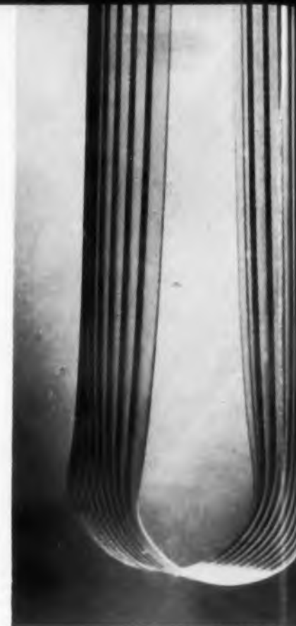
Fig. 13. (right) A curved cross-section makes a flat cable self-supporting.
