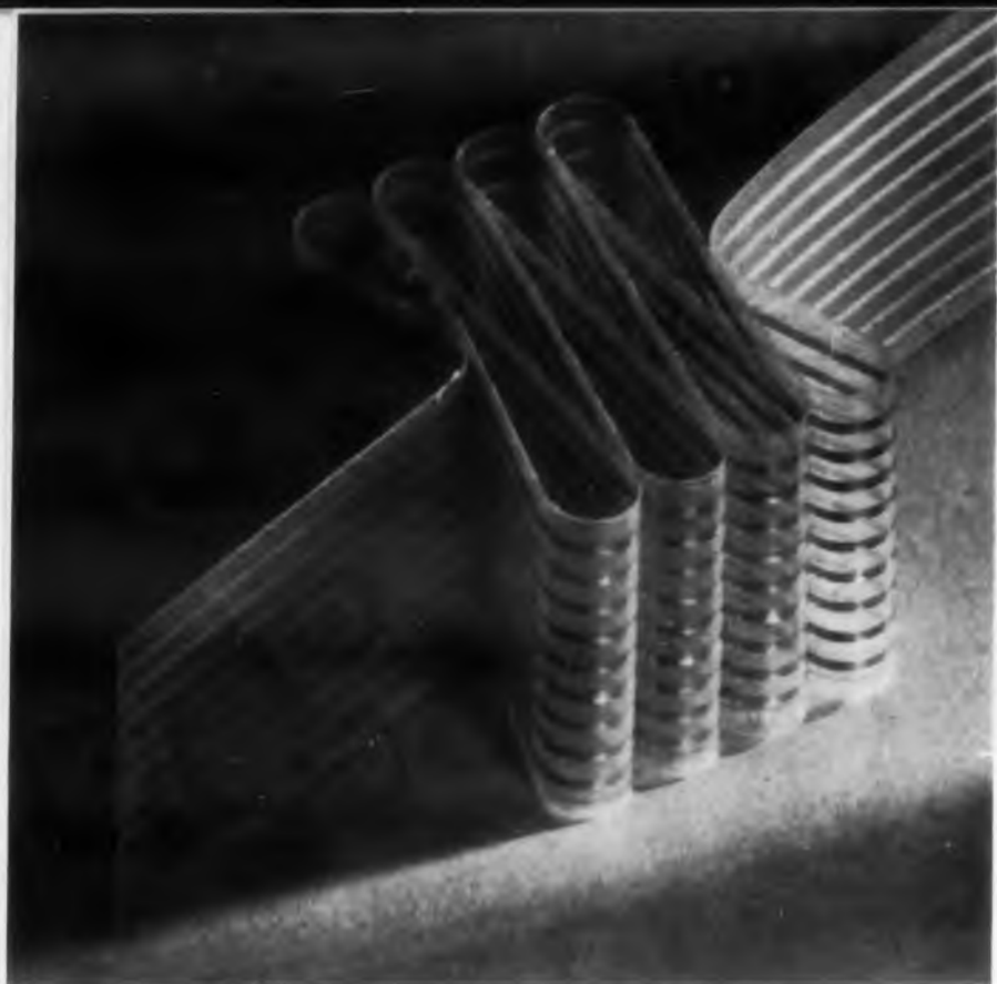
Fig. 11. (left) An "S" shaped retractor cable can be used for connecting a sliding chassis to a rack.
