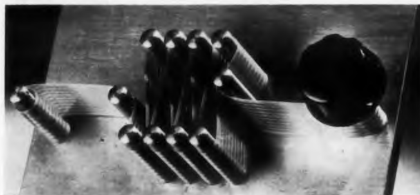
Fig. 12. (above) Heat forming fixture for retractor cable.
