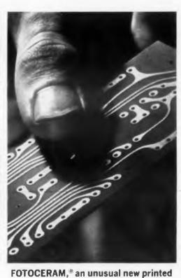
circuit board We've resoldered more than fifty times on this board without damage to circuit runs or through-plate holes. No adhesives needed to bond copper to board. Bond strength between Fotoceram and metal is 15 to 20 lbs., when 1" strip is pulled perpendicular to board. Takes over 60 g vibration shock. All electrical properties equally outstanding.
