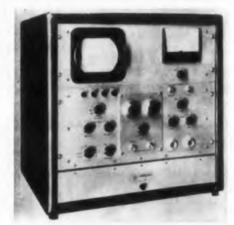
Model 34-8 transistorized 200 channel analyzer uses ferrite core memory system for rapid, accurate spectrum analysis. Linearity is better than 0.5%, average dead time is 60  $\mu$ sec, and normal capacity per channel is 100,000 counts. The unit employs direct parallel decimal readout to printer. Input counting rate without distortion or shift of data is greater than 5 x 10<sup>6</sup> counts per min.
