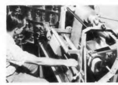
Interleaving sheet-type insulation with aluminum strip.
