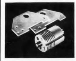
accuracy of ±.001 and the hole spacing is held to a tolerance of  $\pm .002$ . The drum with its stainless steel bearing sleeves is a direct ceramic-to-metal assembly. The bearings must withstand a vertical load of 60 lbs. Three of the end holes are tapped. The slot, the pitch and the depth of the spiral winding groove are ground to tolerances of  $\pm .001$ .
