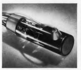
Protection from high altitude arc-over and corona is provided for this cathode ray tube by encapsulating all lead wires with RTV (room temperature vulcanizing) silicone rubber. Designed for airborne operation and installed in a non-pressurized section of the aircraft, tube is protected from arc-over and corona at altitudes up to 70,000 feet.
