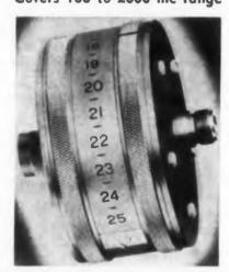
Model S-200 radial double-stub tuner covers 100 to 2000 mc range. The rotating tuning rings of the unit give calibration references from 0 to 25 and the double-stub provides adjustment of 12.6 in., with 1.9 in. spacing. Characteristic impedance is 50 ohms. The unit weighs 2 lb and measures  $3-3/8 \times 4 \text{ in.}$
