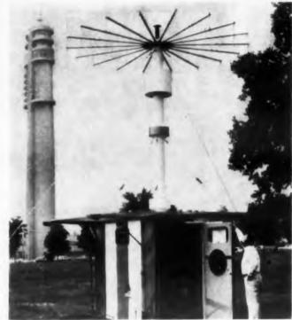
Portable version of CADF direction-finding system functions in both whf and uhf. Roof of shelter is part of uhf counterpoise.
