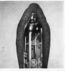
New resilient, shock-absorbent RTV sponge offers improved shock and vibration protection at elevated temperatures; permits easier fabrication than previous methods of cutting, inserting and sealing sponge in place. With RTV, just add sponging and curing agents to compound and mix.
