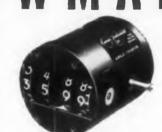
ANGLE COUNTER 1503. Counts from 000.0° to 359.9° and returns to 000.0; Input speed; 1800 rpm max. int., 500 rpm cont.; Weight: 2.5 oz.; O.D.: 1.310 in. Typical of many Bowmar designs currently being manufactured.
