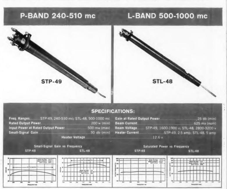
In these two new TWT's, Sperry brings you the unique combination of high output power, broad bandwidth, and rugged environmental construction for the P and L bands. They are the only tubes of their kind available. Together they offer a frequency range of 250 to 1000 mc for such cw applications as "overthe-horizon" communications, long-
