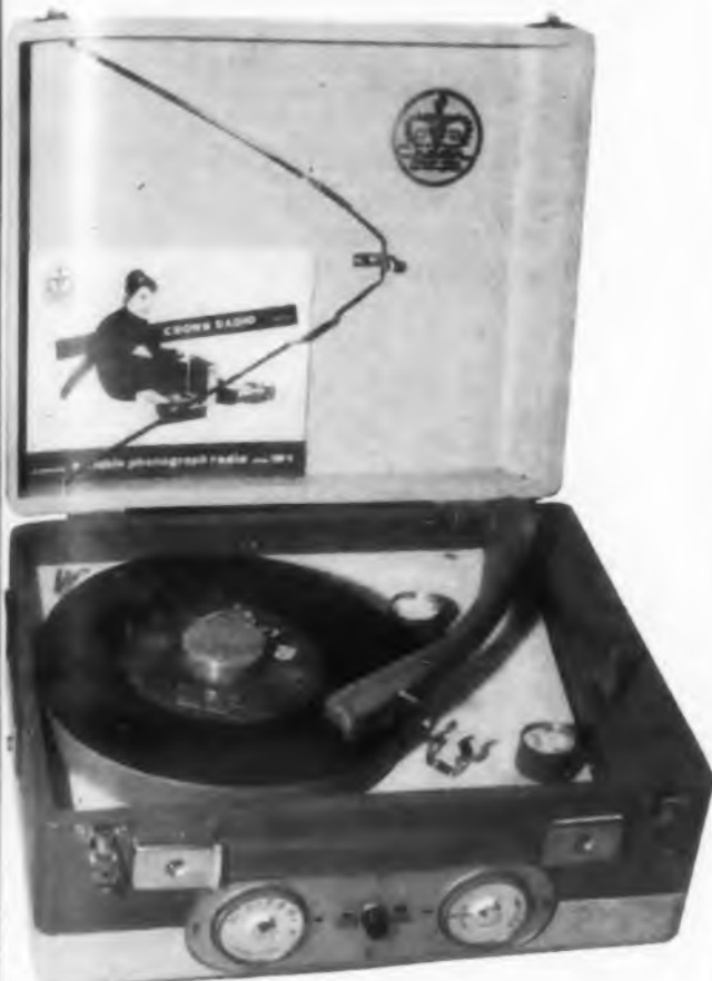
Three speed, seven transistor portable radio-phonograph by Crown Radio of Tokyo weighs only three pounds.
