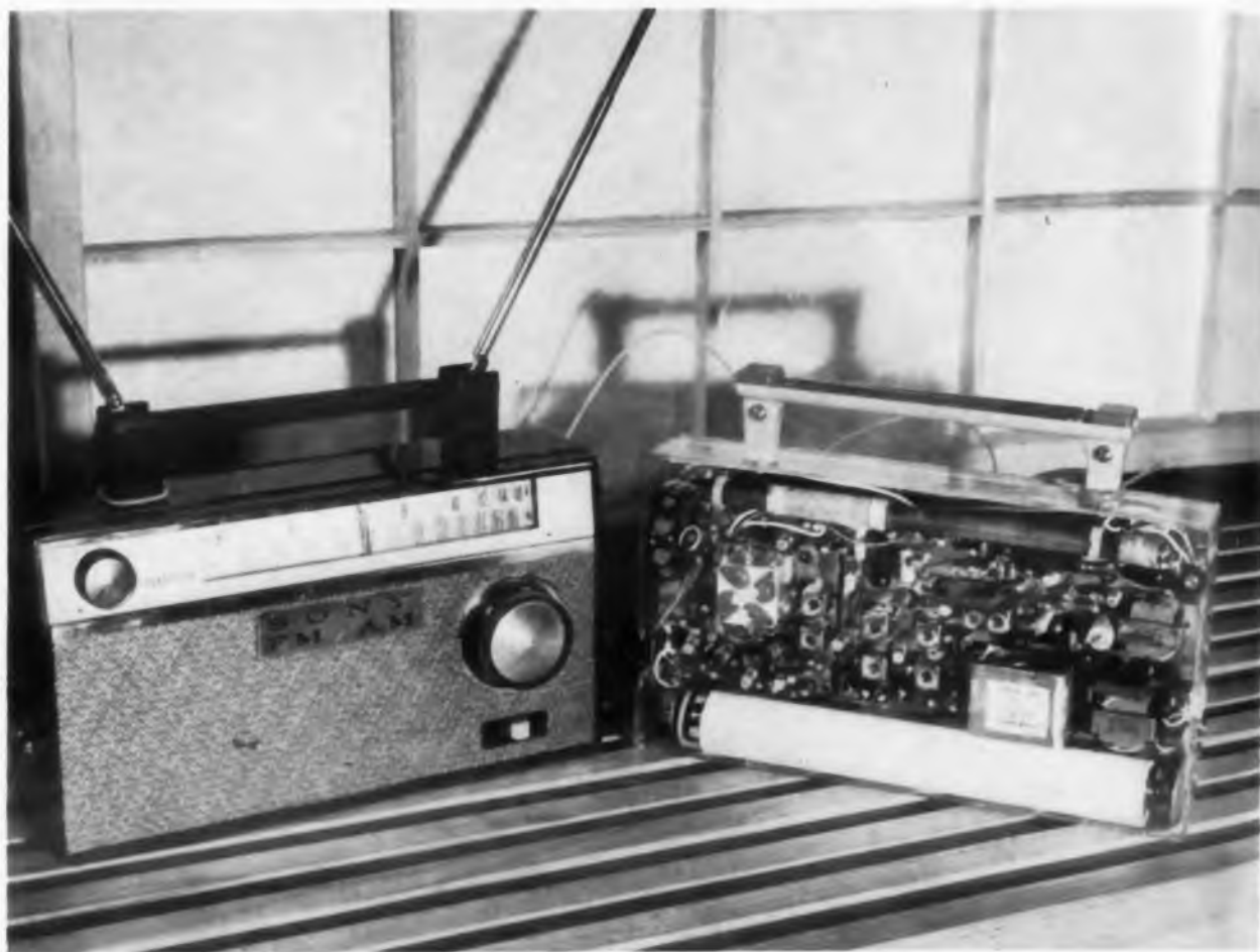
Latest AM-FM transistorized portable from Sony Corp. contains 12 transistors plus 2 diodes and is provided with a multiplex output jack. The FM antenna conveniently folds into the carrying handle when not in use. The retail price is under $100.
