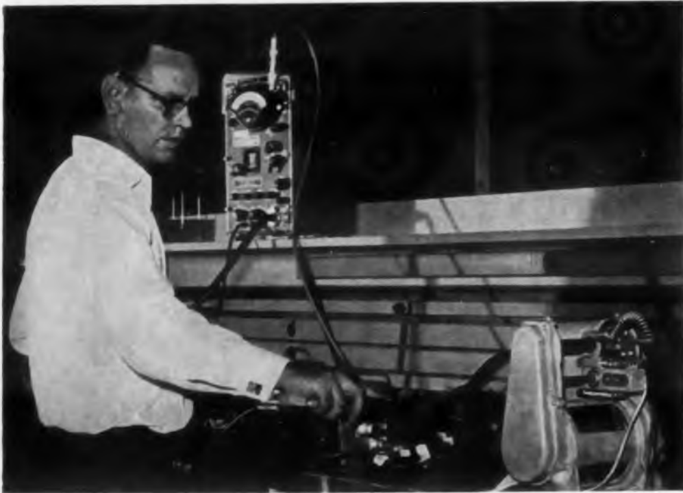
A technician probes radiated interference from an aircraft hoist in the Los Angeles laboratory of Sprague's Interference Control Field Service Dept.
