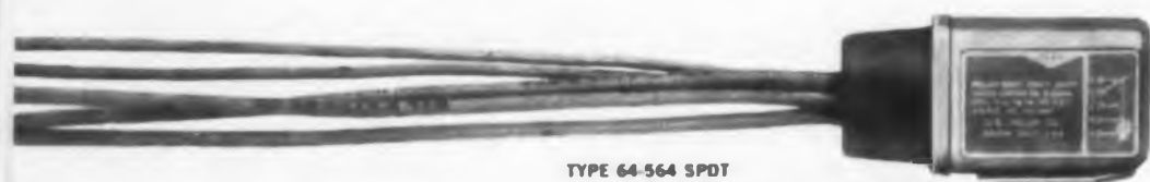
TYPE 64-564 SPDT Nominal operating voltage . . . 14 to 29 VDC Contact Load at 29 VDC . . . 15 Amp. Res. Temperature . . . -65°C to +120°C Hermetically sealed, potted leads.
