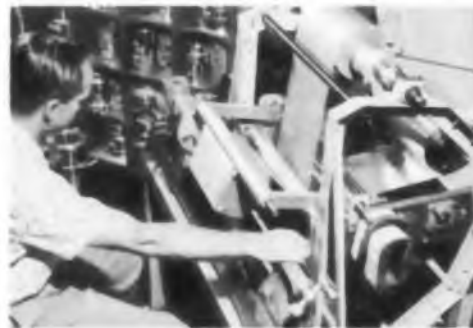
Interleaving sheet-type insulation with aluminum strip.
