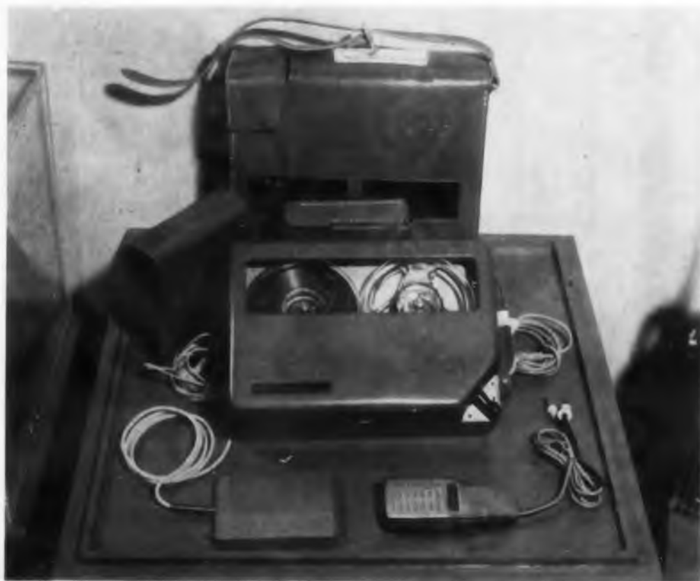
Single-lever control , battery-operated tape recorder, with four-transistor amplifier, operates at 3-3/4 ips. Only 7-1/4 in. by 2-1/2 in. by 5 in., the unit, made by Victor of Japan Ltd., weighs a mere four pounds.
