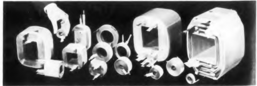
Versatile is the word for aluminum strip in electromagnetic equipment. The strip winding technique is applicable to a wide range of coil sizes and dimensions.
