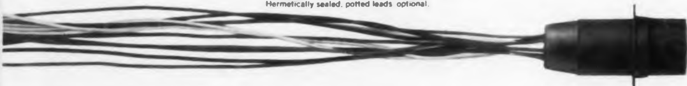
TYPE M-101 and M-102, 2PDT Magnetic latch or Standard. Crystal case size. Voltage . . . 28 VDC Standard; other voltages on request. Contact Load at 29 VDC-2 Amp. Res. Temperature . . . to 125°C. Terminals and mounting optional. Hermetically sealed.
