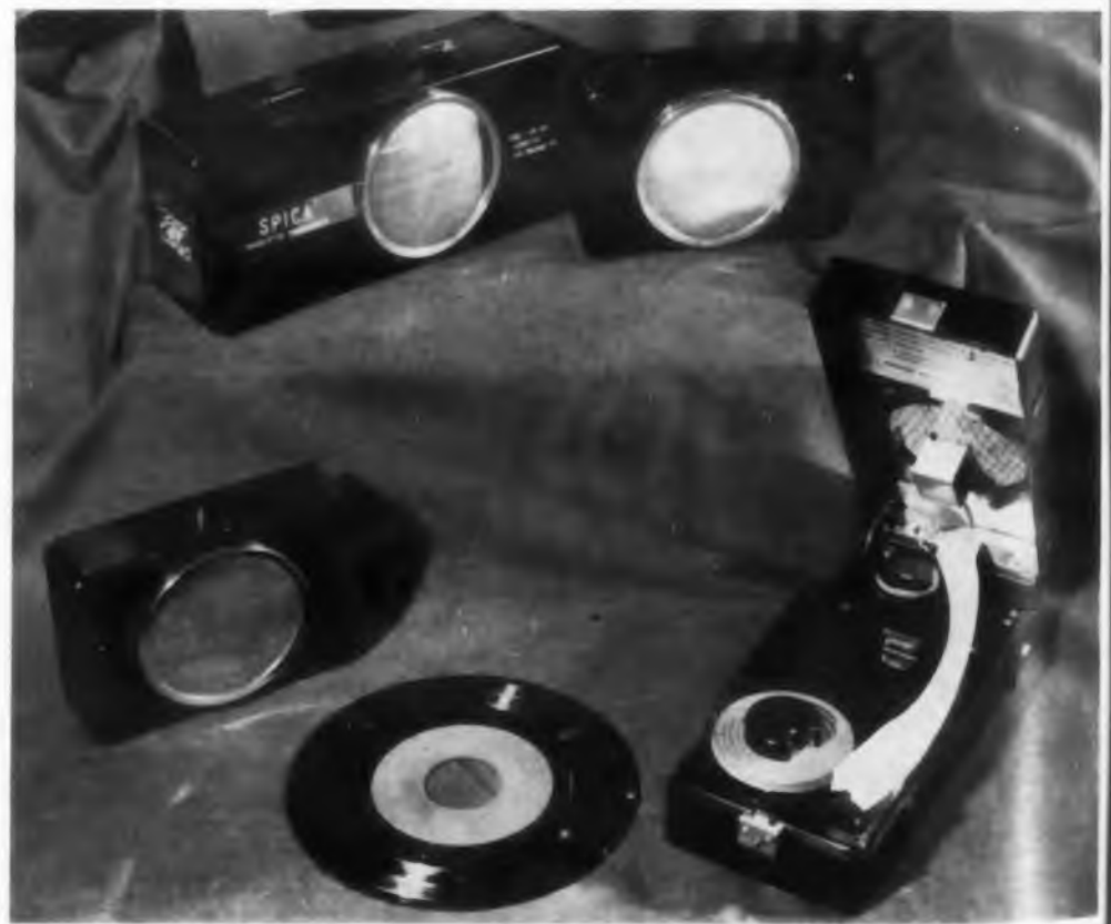
Portable four-speed stereo phonograph, shown by Sonritsu Elec. Mach. Co. of Tokyo, includes a self-contained four-transistor amplifier and speaker. Although the turntable is only slightly larger than 2 in. diam, records up to 12 in. size can be played. The complete set weighs only three pounds and is approximately 3 in. by 3 in. by 8 in. A separate speaker plus transistor amplifier accessory is available for stereo playback.
