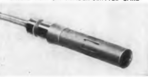
Inconel-sheathed total temperature probe mounted on Redstone missile nose cone — assures high strength at high temperatures and readily withstands oxidation, erosion and thermal shock at extreme velocities. Probe (shown at right) is product of Aero Research Instrument Company, Inc., Chicago, Illinois.
