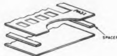
Fig. 1. Cardboard spacers are inserted as above. Spacers should be the same width as the inside slider to provide the proper amount of friction.
