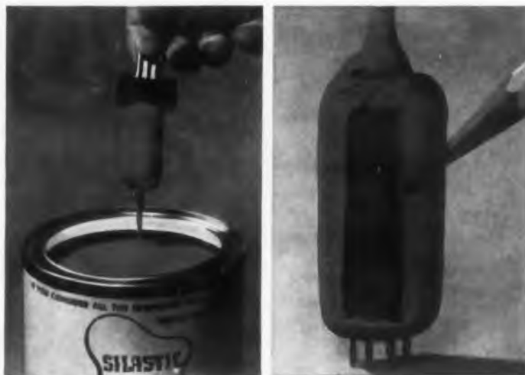
Electronic tube encapsulated with Silastic.
