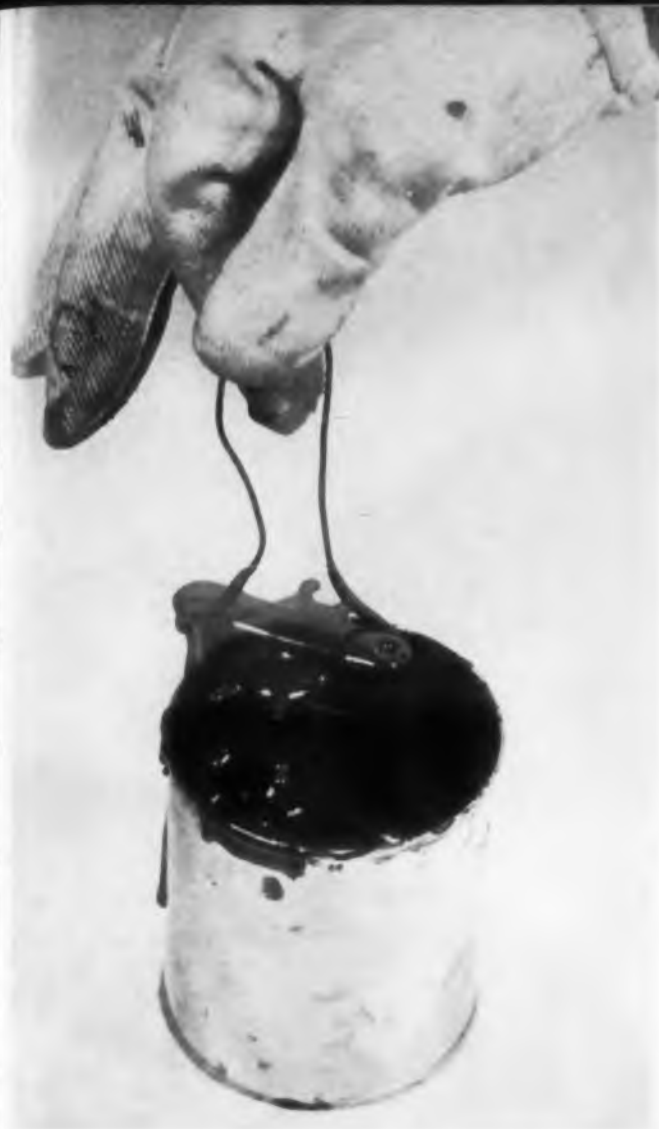
Fig. 1. Units dipped in thixotropic resin will meet military specs without the necessity for molding.
