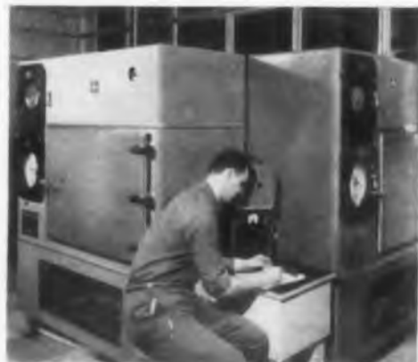
Test for insulation resistance as conducted by Synthane Corporation.
