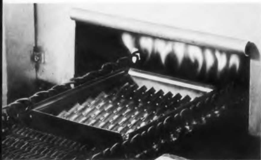
EXCLUSIVE FLAME SHIELD firing of grids and parts removes microscopic lint particles
