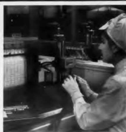
Comparator measures dimensions to one-millionth of an inch. One of many pieces of ultra-precision equipment in the New Departure instrument/miniature ball bearing laboratories.
