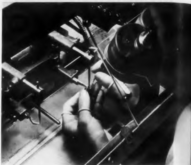
ALL TUBE MOUNTS are precision-welded under stereo microscope
