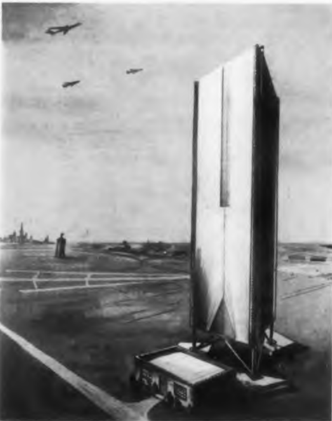
Artist's conception of the Air Height Surveillance Radar Antenna. Radar signals reflected by aircraft from as many as 100 different elevation levels are detected.
