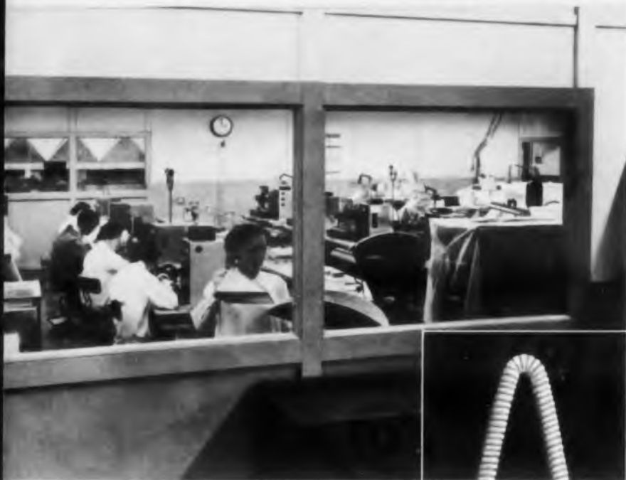
SYLVANIA'S ORIGINAL folded coil heater design is processed in this ultra-clean room to prevent contamination
