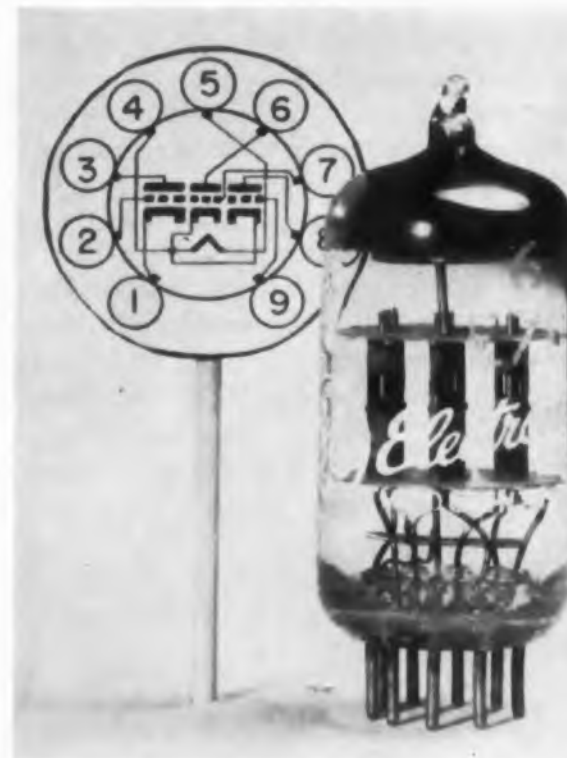
Fig. 1. Having three triodes packed into one envelope, this tube can serve as a one-tube tuner for frequencies as high as the fm band.
