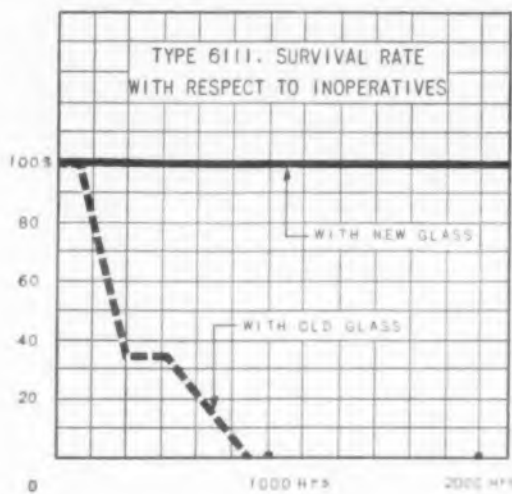
Life tests above to military specifications except for bulb temperatures, raised to 300 C. Left: shows 2000-hour inoperative percentages for Type 6111, a subminiature known to suffer from glass electrolysis at higher-than-rated temperatures. Right: shows reduced G_m drop for new glass versus old, Type 5899. At high temperatures this tube had a tendency to slump in transconductance.
