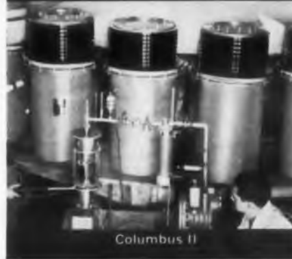
Naval Research Lab's Condenser Battery
