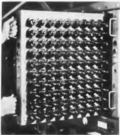
OVER 1.5 MILLION TUBES a month receive burn-in stabilization on specially designed stabilization equipment
