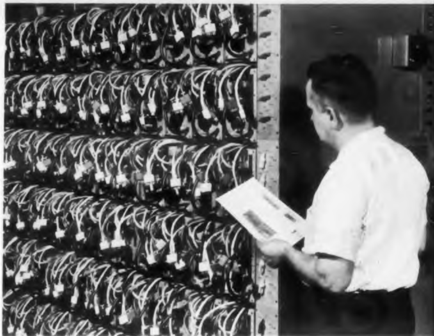
ALL SYLVANIA GOLD BRAND TUBES receive thermal and electrochemical aging on Sylvania designed equipment
