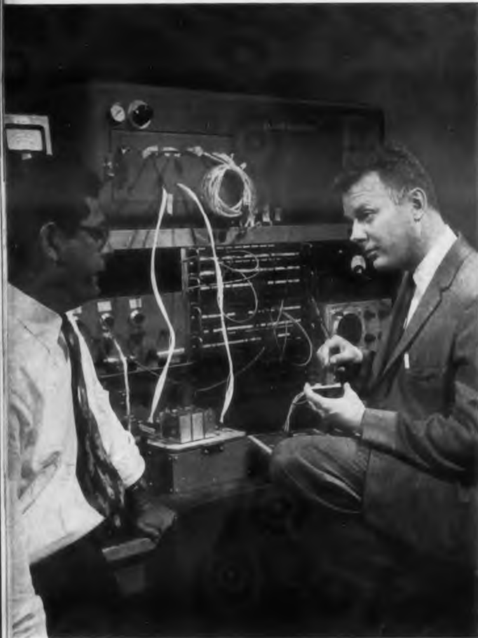
Transistorizing missile flight control systems by Lockheed scientists has meant significant reductions in weight and space requirements.
