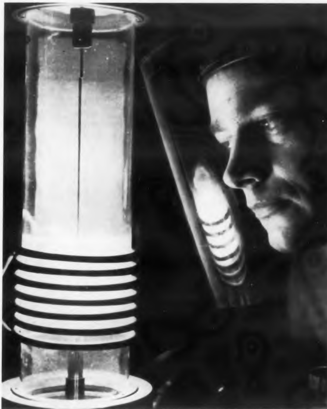
A ribbon of germanium rises from molten pool in a crystal-growing furnace at Westinghouse laboratory as technician observes progress.
