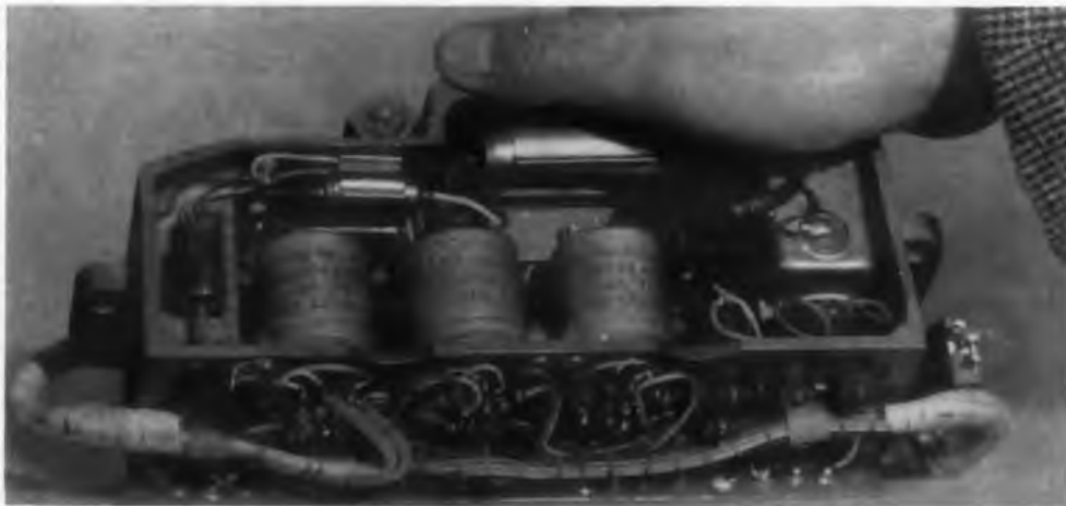
Three UNION miniature 6PDT relays positioned in part of the Talos guidance control system.
