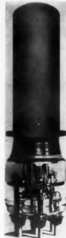
High Power Triode Handles 8 megawatts peak
