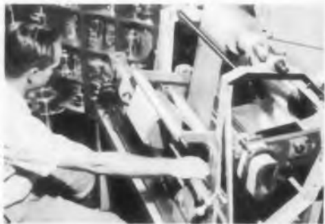
Interleaving sheet-type insulation with aluminum strip.
