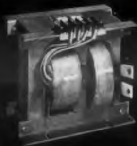
High impedance type transformer from 0.01 to 50 KVA and up to 10 KV. This unit is used for applications where short circuit current must be limited.
