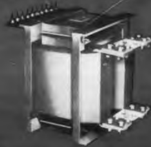
This transformer features low voltage high current secondary windings up to 4000 amps., and up to 300 KVA. Taps on the primary windings afford a wide range secondary current.
