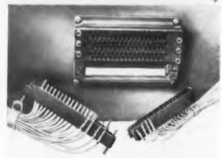
Feed-thru, modular design, multiple insert connector. 35 contact inserts, can be re- moved from frame for easy contact insertion or removal. 5 or 8 insert frames available.
