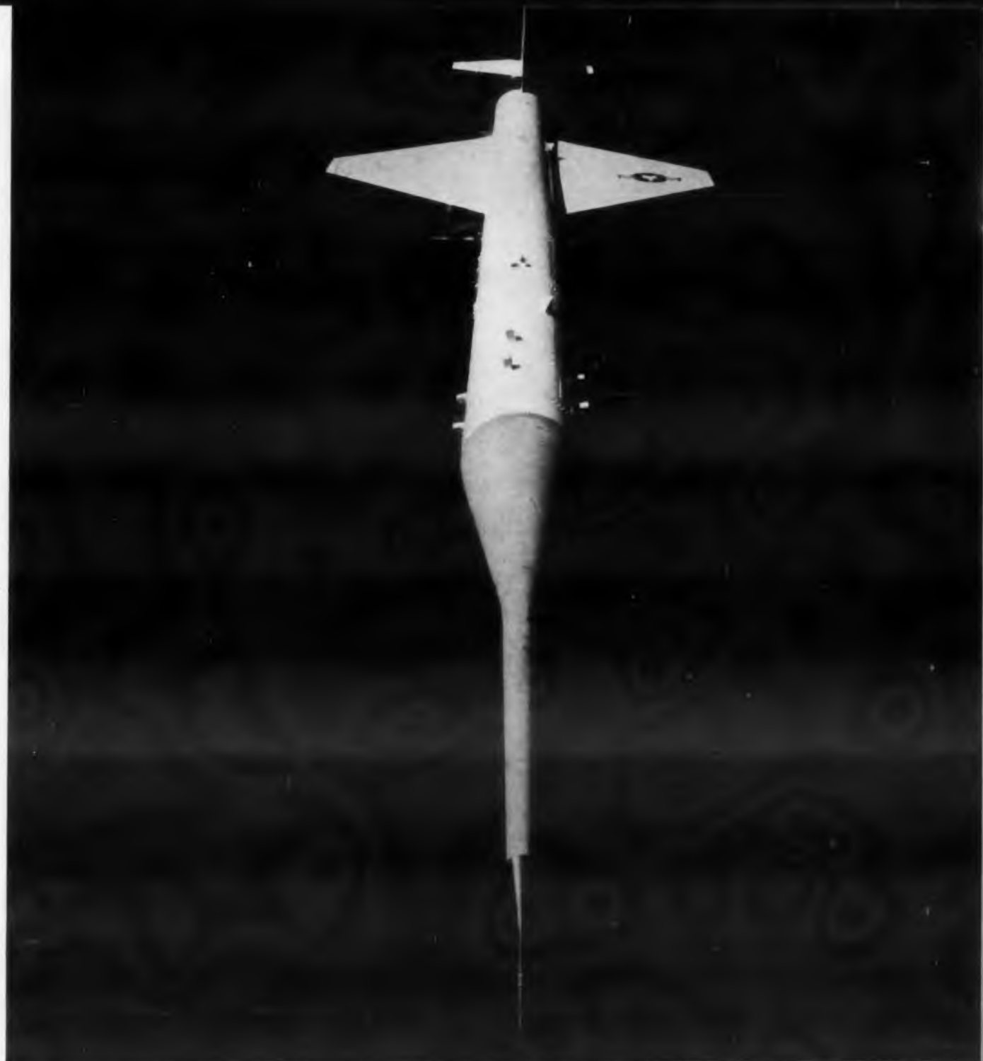
Lockheed Q-5 target missile features telemetry that registers miss-distance and theoretical hits in testing accuracy of other missiles.
