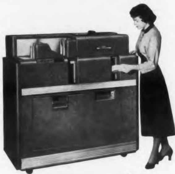
The IBM 528 Accumulating Reproducer is a high speed punch that performs addition and subtraction in combination with any of the operations of gang punching, reproducing and summary punching.
