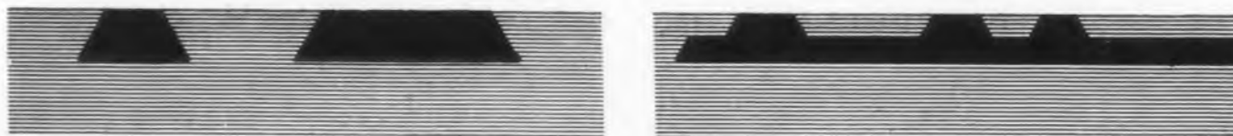
Fig. 1. Flush circuitry (left) and imbedded circuitry (right).
