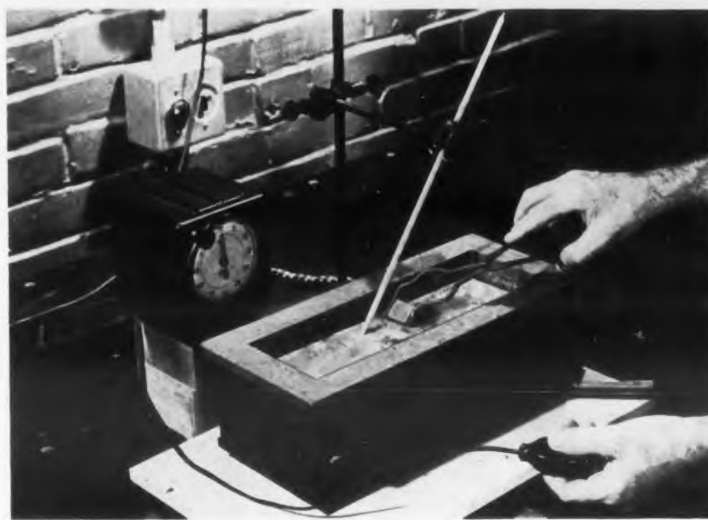
Fig. 1. Test specimens are floated in a 475 F solder bath to determine blistering characteristics. One-inch square specimens are standard, but Synthane also uses round pieces of the same area.
