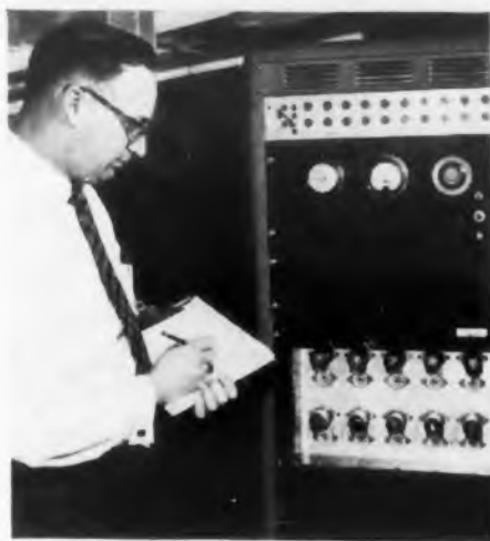
Quality Control inspector examines destructive life test tubes, the oldest of which has been counting continuously since July 2, 1955—a total of over 21,000 hours
