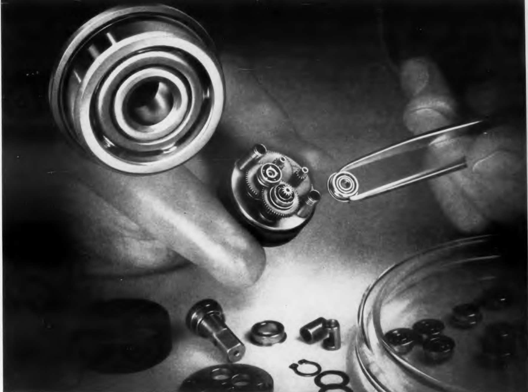
Barden Precision SFRI-5 miniature bearings as used in a computer gear train.
