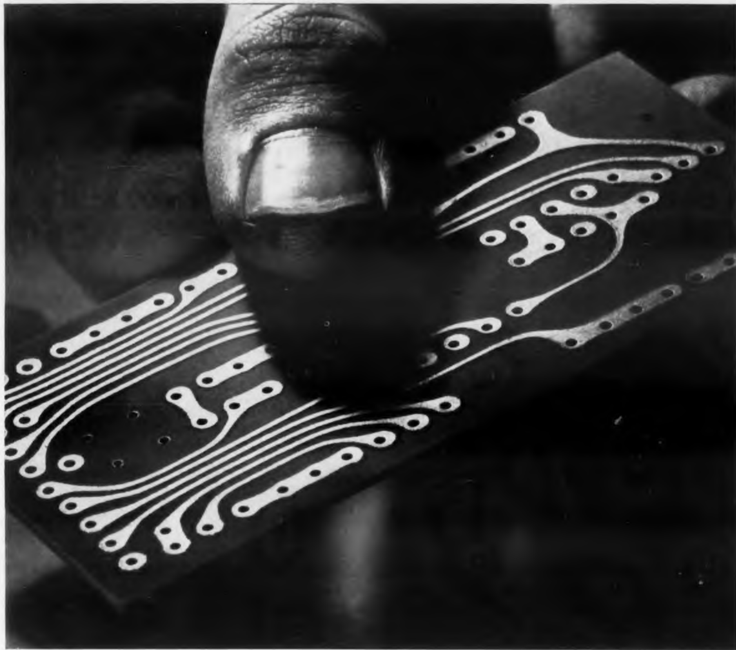
FOTOCERAM circuit board blanks are made photographically. All holes and shapes are produced by simple exposure to light, heat, and an etching operation.
