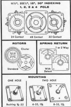
ELECTRICAL SPECIFICATIONS: Operating Voltage—to 2000 volts; Breakdown Voltage—to 3000 volts; Breaking Current—5 amp @ 125 V. ac.; Carrying Current—15 amp.
