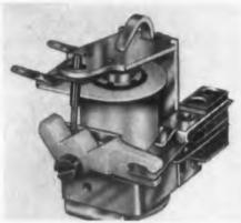
Type W impulse latching relay features an insulated rocker arm activated by a single coil, instead of the two coils usually used. In this one-coil design, the contacts are set up in one position when the coil is energized or pulsed and return to the first position on the next pulse.
