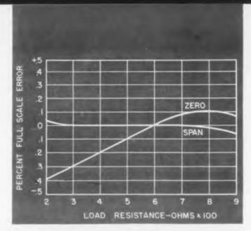
Fig. 6. Ratio amplifier constant current properties.
