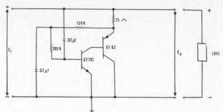
**Fig. 6.** Practical two-stage transistor-simulated shunt capacitance, designed to replace a 6 v, 150 uf capacitor.
