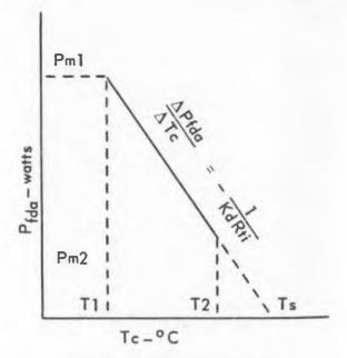
Fig. 1. Modified thermal limit curve. The range covered is usually limited to some extreme temperatures,  $T_1$  and  $T_2$ .
