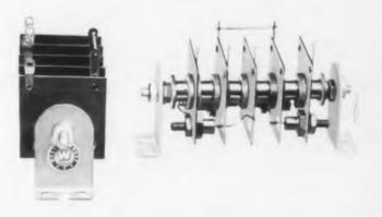
This is a 4-1-1 single-phase full-wave bridge using 305 cells on  $1\frac{1}{2}$ " x  $1\frac{1}{2}$ " copper plates. At an ambient temperature of 30° C, it will deliver up to 3.2 amperes d.c. with convection cooling. The primary applications are power supplies, relays, solenoids, mag amps, etc.
