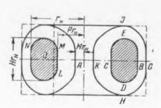
**Fig. 1.** Transverse section of toroidal core of the (oval) form investigated by Rabkin and Novikova.
