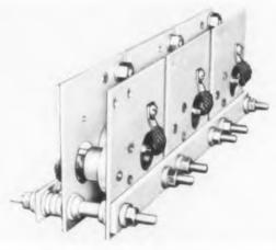
This is a 6-1-1 three-phase full-wave bridge using 322 cells on 5" x 5" copper plates. At an ambient temperature of 30° C it will deliver up to 132 amperes d.c. convection cooled, or 330 amperes d.c. with forced air cooling at 1000 l.f.m. The primary applications are welding, electro-plating, chemical reduction, arc furnaces, motor drive, battery chargers, etc.
