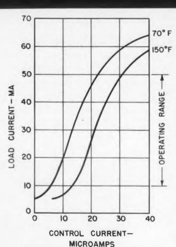
Fig. 4. Open loop transfer characteristic of ratio amplifier.
