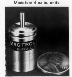
These units are available in a number of configurations, consisting of clutches, brakes, clutchbrakes, and a special dual clutch-brake. Other models are available for fail-safe or reverse energization applications. The method of mounting is with a standard 1/2 in. diameter servo mount, on either or both ends, with concentric output and input members. Shown is the model FB-59 Microbrake.
