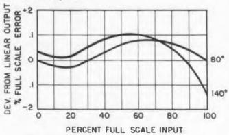
Fig. 5. Linearity and temperature response.
