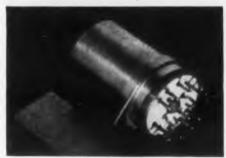
This 4pdt relay has the following characteristics: Operates in an ambient temperature of +200 C, withstands 55 g shock for 11 msec, withstands 25 g vibration up to 2000 cps, and has a contact bounce of less than 250 usec. Insulation consists of all ceramic material in order to maintain high resistance at maximum operating temperature. The coil is hermetically sealed from the contact structure. The relay retains the rotary principle of operation standard in the Company's line of relays.
