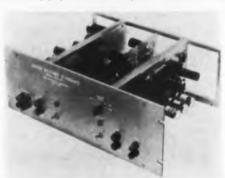
The model AVS-320 audio voltage standard has output voltages of 1, 10, 100, and 300 rms. Frequency range is 30 cps to 20 kc; input voltage 1 v rms; output regulation of plus 0.1 per cent for a period of 30 days, with distortion of less than 0.025 per cent. Power source is 105 to 125 v ac 60 cps, 150 w.
