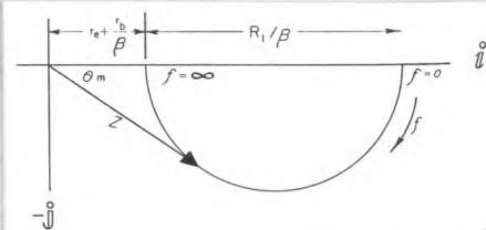
Fig. 2. Complex plane representation of eq. (3) illustrating the variation in impedance with respect to frequency.
