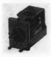
Type BHSM-HT relay is rated at 500 cps at 10 g vibration. The unit uses cross-bar palladium contacts, silicone-glass pile up insulators, a welded bracket assembly and frame, Teflon magnet wire, and a Kel-F-Coil bobbin. The relay is designed to operate at a temperature range of -65 to +125 C and will withstand 30 g operating shock or 70 g non-destructive shock.
