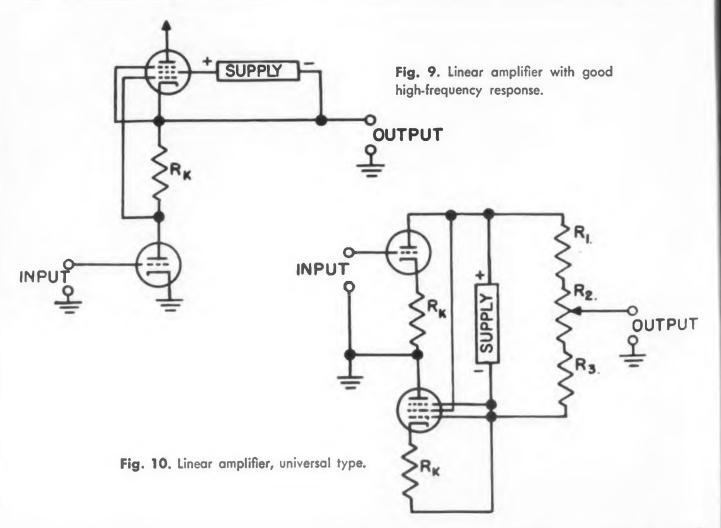
od linearity obtained by means of a constant rrent plate load impedance. Along with the aprovement in linearity over the conventional tode amplifier comes higher gain (very close to ie mu of the triode) nearly constant output imclance, and better high frequency response. A ombination of the circuits found in Figs. 8 and produces the circuit of Fig. 10 having a group desirable properties:
