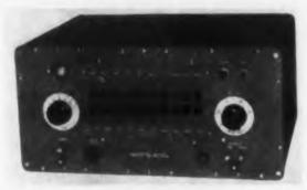
Push-button selection of frequency is featured in the model TO-258 telemetering test oscillator. The unit is designed to provide convenient calibration for sub-carrier units of fm/fm telemetering systems. Standard fm/fm frequencies from 400 cps to 70 kc are supplied with calibrated deviation control of  $\pm 15$  per cent of center frequency. Distortion is less than 1 per cent to 21 ma rms, frequency error is less than 1 per cent and output voltage is constant to 1 db from 1 to 25 v.
