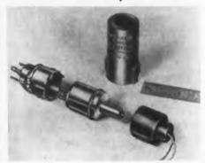
Having low thermal construction, this chopper is useful in de amplifiers requiring thermal stability and low noise. Contact ratings and reliability are identical with the company's standard external coil units. As in the standard ← CIRCLE 122 ON READER-SERVICE CARD
