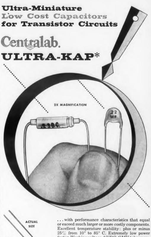
Excellent temperature stability: plus or minus 25% from 10° to 85° C. Extremely low power factor. Working voltage, 3 VDC. GMV tolerances. Maximum thickness, 0.156".
