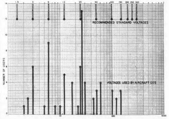
Fig. 1. Proposed standard power supply voltages.
