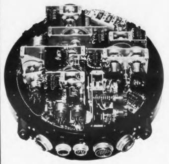
The Air Data Computer provides pressure altitude, indicated air speed, Mach number, true air speed, and vertical speed information.
