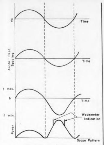
**Fig. 4.** Time relationship of the drive voltage, anode reed spacing, frequency variation, and power output.
