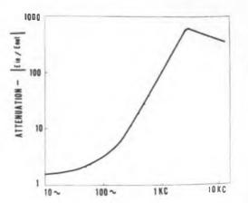
Fig. 9. Attenuation for circuit of Fig. 8. Maximum attenuation of 55 db occurs at 2kc.
