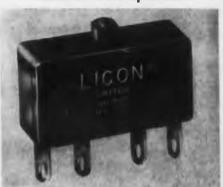
The type 16 10-amp miniature switch measuring 1/4 x 7/16 x 25/32 is available with screw end terminals, and bottom taper tab and solder terminals. The switch provides over 20,000,000 life cycles. Double break contact arrangement is employed. A broad field of application is possible by combining the switch with an assortment of miniature actuators. Actuator designs include panel mounted toggles, oil-tight push-buttons, and spring pivoted lever, roller, levers.
