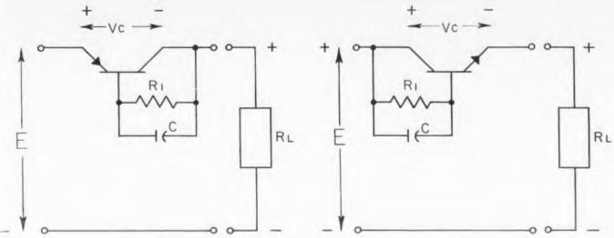
Fig. 3. Transistor simulated series capacitance, modified from the circuit of Fig. 1.
