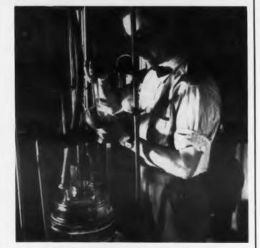
**Atom-by-atom buildup** of the transparent phosphor screens is accomplished with this vapor phase deposition equipment. An evaporation process may be used.
