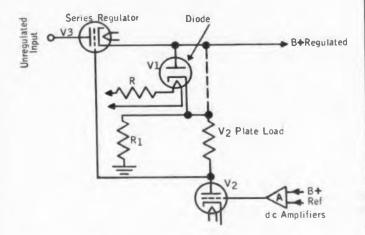
Modified Voltage Regulator Circuit. Diode prevents V<sub>8</sub> from being overloaded until heater reaches normal operating temperature.
