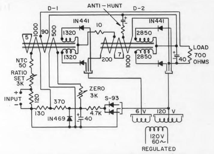
Fig. 3. Ratio amplifier schematic. The system uses two stages of magnetic amplification.
