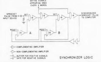
**Fig. 5.** Synchronizer logic. Two flip-flops (A and B) are used in a set, partial set, or reset condition.
