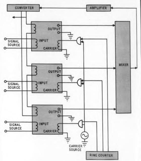
Fig. 4. A more accurate commutation system than that of Fig. 1. Here the magnetic amplifiers function as null detectors.
