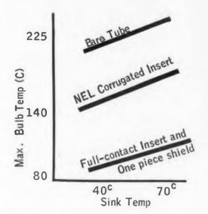
Fig. 2. Bottom curve approximates the cooling performance of the insert in a one-piece shield, using a type 5687 tube.
