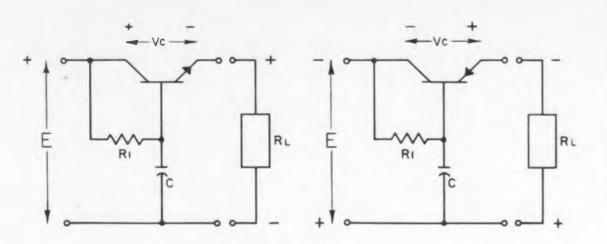
**Fig. 5.** Transistor simulated series inductance, using only capacitance as the reactive parameter.
