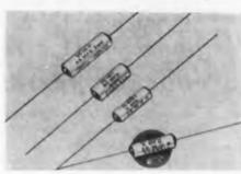
Type EC electrolytic capacitors are available in ratings from 3 to 75 v dc working, and in capacitances from 1 to 250  $\mu$ f, depending on voltage ratings. Operating temperature range is -20 to +65 C. The smallest case size is 0.187 in. diam and 1/2 in. long, and the largest is 0.375 in. by 1-1/2 in. The capacitors are housed in tubular ceramic cases. Capacitor sections are sealed with cast resin making them moisture-tight and heat resistant.
