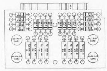
Fig. 6. A shift register package on a single card.
