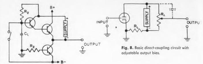
Fig. 7. Bootstrapped transistor ramp-voltage generator.
