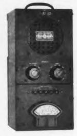
Direct-Reading Output-Power Meter for Audio Frequencies
