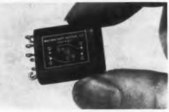
Frame and header assembly or bridge-type construction affords high resistance to shock, vibration, and temperature in this relay. Oversize instrument type bearings at both ends minimize hinge friction. The unit is hermetically sealed and filled with inert gas.
