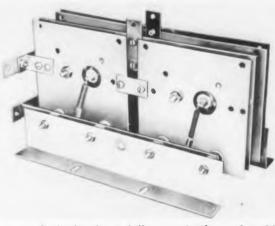
This is a 4-1-2 single-phase full-wave bridge using 302 cells on  $5" \times 5"$  copper plates. At an ambient temperature of  $30^\circ$  C, it will deliver up to 94 amperes d.c. with convection cooling, or 178 amperes d.c. with forced air cooling at 1000 l.f.m. The primary applications are d.c. power supplies, vibrator and magnet coil supplies, motor control, etc.
