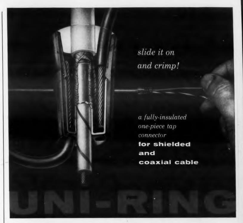
UNI-KING offers a tremendous saving in installation time over any previous method of tapping or terminating shielded or coaxial cable. As the inner ring slides under the shielded braid, the tap wire is held between the braid and the outer ring. Single or multiple taps, from either the front or back of the connector, can be accommodated . . . A single crimp, using the same basic hytools used for installing hyrings, completes the uniform, secure, and insulated assembly.
