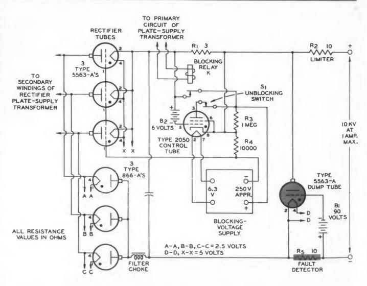
Fig. 1. High-speed fault-protection circuit showing dump tube.
