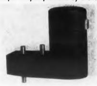
Three output shafts are provided on this permanent magnet dc motor to satisfy multiple use applications. The motor, used with this gearhead, incorporates the manufacturer's symmetrical, progressive lap type armature winding to provide electrical balance, superior commutation, and low radio noise output. Magnets are stabilized to eliminate demagnetizing effects due to sudden reversals. Elementary control circuits provide dynamic braking.
