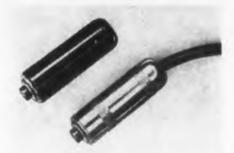
Designed for numerous remote control applications, this push button switch, enclosed in a handle, provides a cord mounted or pendant switch. Housing is nickel plated brass or black phenolic. The red or black push buttons are nonlocking. The switch is rated at 250 ma, non-inductive load, ac 30 w maximum.
