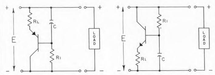
Fig. 4. Shunt inductance circuit, using only capacitance as a reactive parameter.
