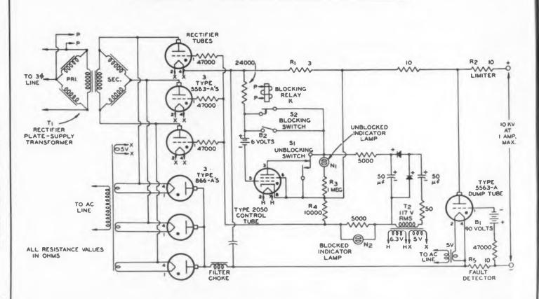
Fig. 2. Complete fault-protection circuit.
