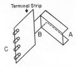
A. This part of the terminal strip is fitted over the core prior to the winding. The windings will act as mechanical security for the strip.
