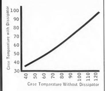
This graph compares transistor case temperatures with and without the heat sink. Temperatures are in degrees Centigrade.
