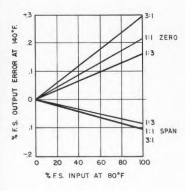
Fig. 9. Effect of ratio setting on temperature response.
