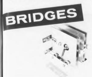
This is a 4-1-1 single-phase full-wave bridge using 303 cells on 5" x 5" copper plates. At an ambient temperature of 30" C, it will deliver up to 27 amperes d.c. with convection cooling, or 53 amperes d.c. with forced air cooling at 1000 l.f.m. The primary applications are d.c. power supplies, vibrator and magnet coil supplies, motor control, etc.
