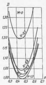
Figs. 2 and 3. Dependence of loss angle (D) on the dimensional ratios H and P (which are defined on Fig. 1) for cores in which the magnetization losses predominate (Fig. 2) (left) and for those in which hysteresis losses predominate (Fig. 3).
