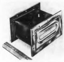
The MA-336/7166, first in a series of L-band high power duplexer tubes, is conservatively rated at 2 megawatts peak power and 4 kw average power for continuous operation over a minimum life span of 500 hr.
