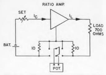
Fig. 8. Circuit for precision testing of ratio amplifier.
