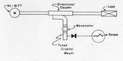
Fig. 1. The components employed for the simple measurements are a directional coupler to sample the energy, a wavemeter, a tuned probe crystal mount, and an oscilloscope.
