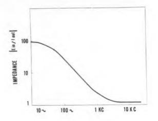
Fig. 7. Effective impedance versus frequency for circuit of Fig. 6.
