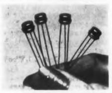
Four germanium alloy transistors designed for computer applications will be among the semi-conductor devices exhibited by this company. Designated types 2N312, 2N356, 2N357, and 2N358, the units feature rapid switching, high constant beta characteristics, and excellent leakage stability. The transistors have base-off-the-can construction for applications where it is necessary to isolate all elements.
