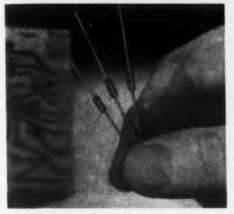
A line of miniature glass Zener diodes has been designed for clipping, limiting, regulating, and similar applications. They are made with gold alloyed ohmic contacts in order to withstand high operating temperatures.
