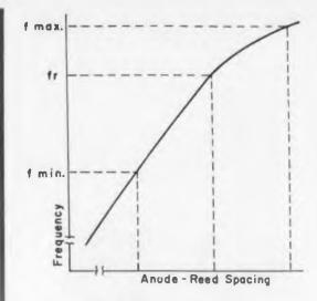
**Fig. 2.** The magnetron's tuning rate curve.
