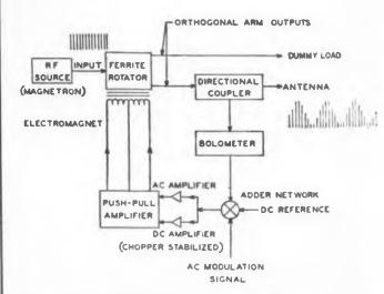
This block diagram (discussed in the text) shows how the plumbing and electronic components work together.
