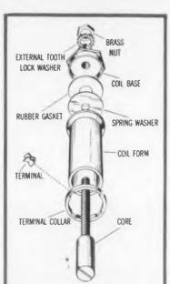
National Company, one of the nation's oldest suppliers of quality coils and coil forms, now introduces, for immediate delivery, a new line of ceramic coil forms, engineered to meet the most rigid military and commercial applications.
