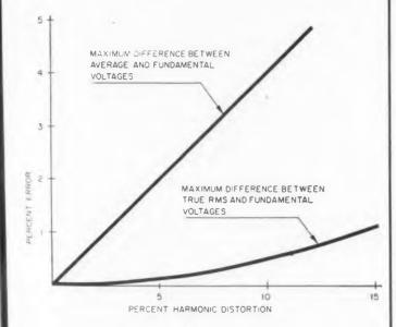
Computed errors between true rms voltage of a complex wave and value of the fundamental, and between average voltage and value of the fundamental.
