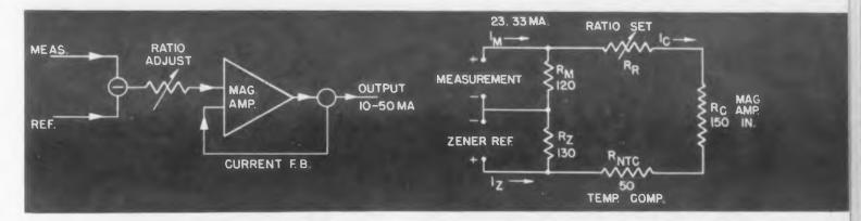
Fig. 1. Block diagram of ratio amplifier.
