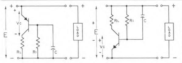
Fig. 1. Circuit for transistor-simulated shunt capacitance. The value of the capacitance used in the base path is multiplied by the transistor gain.
