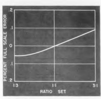
Fig. 7. Effect of ratio setting on "zero."
