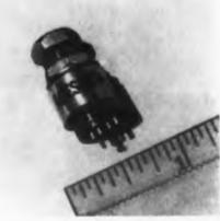
Offering high stability under temperature cycling in a small size, these Aceset potentiometers will dissipate 2 w at 60 C. They are available in nine resistance ranges between 100 and 25,000 ohms. Temperature cycling stability is made possible through the use of 20 ppm temperature co-efficient wire.
