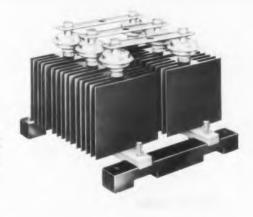
Large area junction type. Operating temperature to 200° C. D-C outputs as high as 85 amps per rectifying element. Lower cost 4JA62 and 6211 units are for applications which do not require the full current ratings of 4JA60 line. Reverse polarities provided in 4JA61 and 4JA63 units. Stack combinations offer d-c outputs up to 915 amps.
