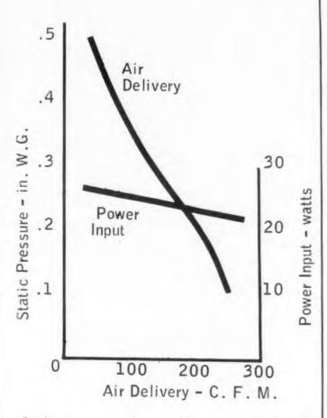
**Static pressure** and power input curves for 60 cycle operation.
