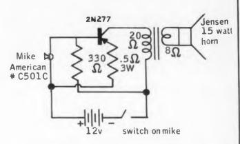
During the course of designing a portable public address system various circuits were tried and discarded because of relative complexity. What was needed was a battery operated, transistorized, 3 to 5 w unit. The circuit shown indicates how this unit was simplified without sacrificing performance.
