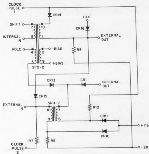
Fig. 4. A typical shift register. There is an additional input winding for each amplifier. In addition, there is a second core with two windings for each bit of information.
