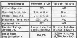
Haydon 6100 Series Switches are available with a wide range of characteristics and can be used with a variety of Haydon standard actuators, such as those shown at the left. Haydon also provides a complete design and development service to solve your problems in hermetically sealed switches and suitable actuators. For further information, write for data on the Haydon No. 61191 Switch.
