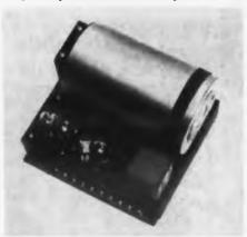
The fork amplifier, model FK5, is designed for maximum frequency stability. An oven is added for applications requiring a frequency source accurate to 1 part in 10<sup>7</sup>. The FK5 chassis is 6-5/8 x 6-1/2 x 4 in. high, and the FK5A (with oven) is 5-1/6 in. high. The amplifier may be mounted in any position. Power requirement is 200-300 v dc and 6.3 v ac. No regulated B+ supply is required. Temperature stability of the oven is well within 0.1 C at the fork assembly.
