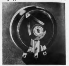
These 100 and 150 w ring rheostats have twin-shoe self-lubricating contacts; molded ceramic base and core featuring high density, low porosity, and high dielectric strength. Ratings of 100 and 150 w rings are based on a 300 C rise in 40 C ambient. Both sizes are available in resistance values to 10,000 ohms. Tapered windings, tandem mountings, dial plates, and other accessories are available.
