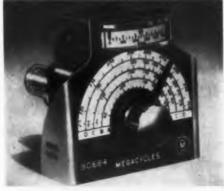
The 90680 series consists of self-indicating, absorption frequency meters covering the range of 170 kc to 700 mc. This frequency range is covered by five basic heads. Each head has three or four plug-in inductor probes and the same number of individual frequency calibrations. A single 500 µamp, end-indicating, plugin circuit is used with each of the heads. The indicating circuit is partially self-limiting so that a high power signal will not damage it.
