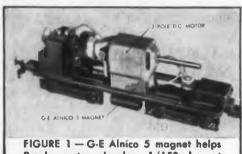
FIGURE 1 — G-E Alnico 5 magnet helps 2-pole motor develop 1/150 hp at 10,000 to 15,000 rpm.
