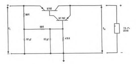
Fig. 8. Emitter follower effect used to match a 75 ohm load to a 470 K terminated filter.
