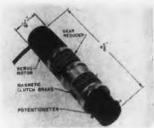
Model T-950 which is a compact servo-package combining a servo motor, a geared reducer, a magnetic clutch-brake and a potentiometer. In this particular unit, the motor drives the potentiometer arm at a speed corresponding to a radar scan rate of approximately 40 rpm. Upon a given signal the motor can be uncoupled and the potentiometer braked within 2 msec.
