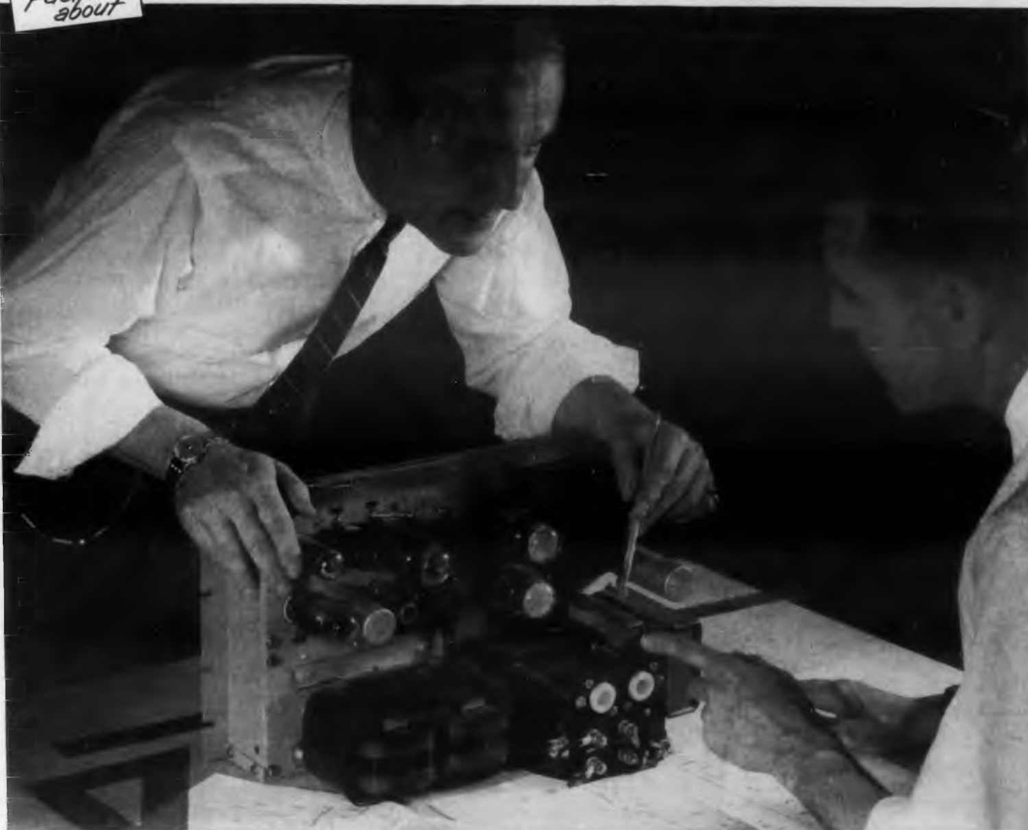
STABILINE type IE (Instantaneous Electronic) is available in 115 volt units — input range from 95-135v. and 230 volt units — input range from 195-255v. STABILINE type IE5101R shown above.
