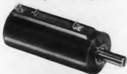
1" 10-turn Metal Case Type 920. Elec. Rotation: 3600°; Res. Range 1K to 1 Meg.; Tol. ±5%; Std. Lin.: ±.25 to ±.05%; Power Rating: 3.5 Watts. Gangable.
