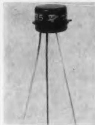
Germanium Transistors For Computer Use
