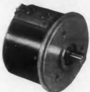
1-13/16" 3-turn Metal Case Type 933. Elec. Rotation: 1080°; Res. Range: 350 to 600K ohms; Tol.: ±5% (±1% on specials); Std. Lin.: ±.25 to ±.05%; Power Rating: 5 Watts; Gangable.
