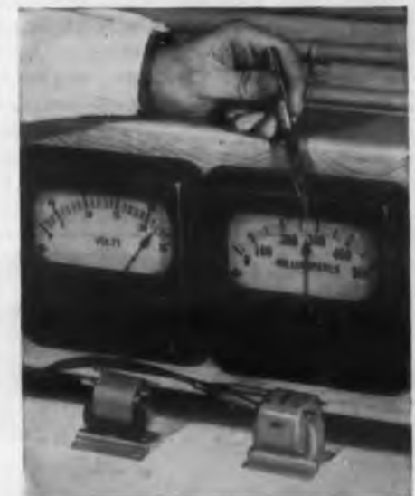
Un-"normalized" core, with the same applied voltage, records considerably higher exciting current after encapsulation.
