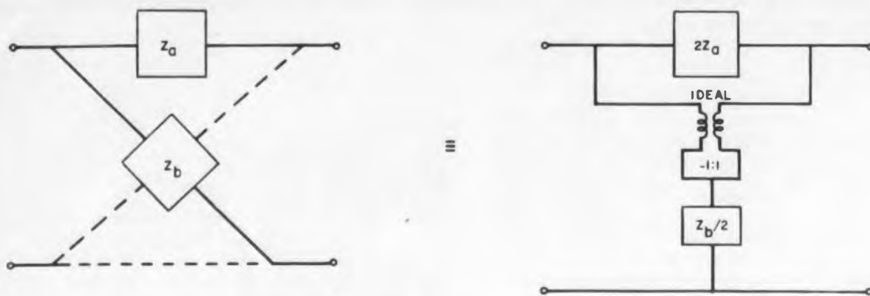
Fig. 3. Reduction of the lattice to a grounded network.
