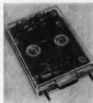
Magnetic Amplifier Controls Low Power Devices
