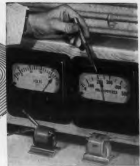
Both "normalized" and un-"normalized" cores record the same exciting current before encapsulation in high-temperature resin.
