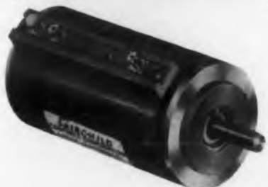
7/8" 10-turn Metal Case Type 908. Elec. Rotation: 3600°; Res. Range: 100 to 100K ohms; Tol: ±5%; Std. Lin.: ±.25 to ±.05%; Power Rating: 2.5 Watts.
