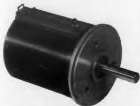
1-3/16" 10-turn Metal Case Type 930. Elec. Rotation: 3600°; Res. Range: 1K to 2 Meg.; Tol. ±5% (±1% on specials); Std. Lin.: ±0.1 of ±0.25%; Power Rating: 5 Watts; Gangable.
