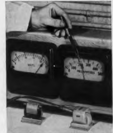
"Normalized" Hipersil core shows exciting current unchanged after encapsulation.
