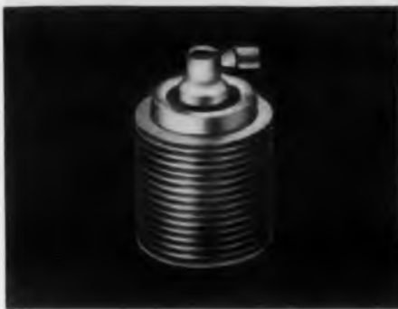
WESTINGHOUSE SILICON RECTIFIER WN-5082, modified as shown, with maximum peak inverse voltage ratings of 50-400 v (300 to 5000 amperes in bridge assemblies).
