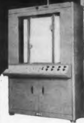
Variplotter Model 205N— for use when record must be viewed from remote location.
