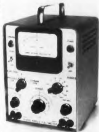
Phase Angle VTVM Measures Phase and Magnitude
