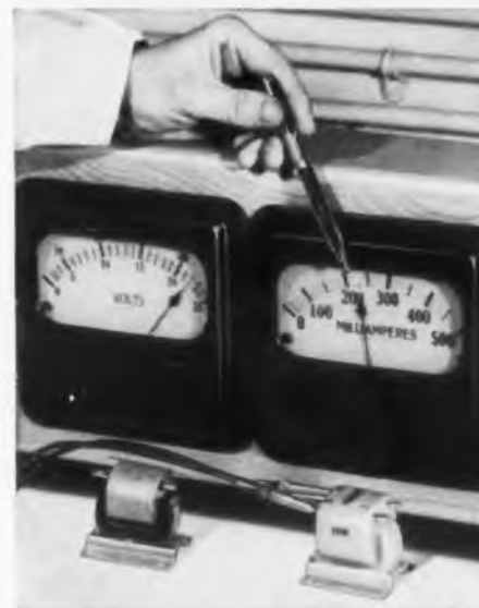
"Normalized" Hipersil core shows exciting current unchanged after encapsulation.
