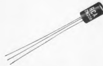
RCA-2N206 —For moderate-power AF amplifier service. Meets military specification MIL-T-25380/4 USAF. (Max. collector dissipation, 75 mw. at ambient temp. of 25°C.)
