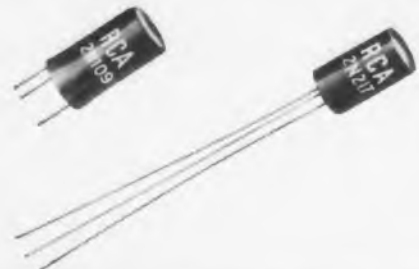
RCA-2N109 —For large-signal AF amplifier service. In class B push-pull, two RCA-2N109's can deliver max. signal power output of approximately 150 milliwatts. Linotetral 3-pin base. For flexible-lead version, specify RCA-2N217 .
