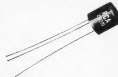
RCA-2N270 —For large-signal AF amplifier service. In class A, one RCA-2N270 can deliver a max. signal power output of approximately 60 milliwatts; in class B push-pull, a pair can deliver up to 500 milliwatts.
