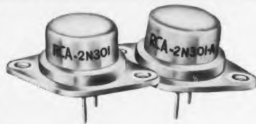
RCA-2N301 —For audio-power output stages of equipment requiring high output with low distortion at high power gain. In class A, one RCA-2N301 can deliver a max. signal power output of approximately 2.7 watts; a pair can deliver up to 12 watts in class B push-pull. For operation at peak collector voltages as high as 60 volts, specify RCA-2N301-A .
