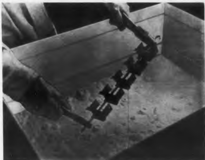
Preheated metal parts being dipped into a tank containing fluidized coating powders.
