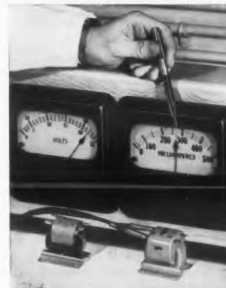
Un-"normalized" core, with the same applied voltage, records considerably higher exciting current after encapsulation.
