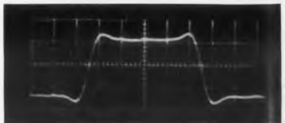
Pulse output from 0.7 \mu sec Delay-Line. Impedance, 6800 ohms. Pulse width, 1 \mu sec.
