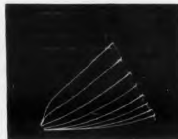
Fig. 2 — Same triode section of 12AU7 with only 20-v peak plate supply and sensitivities increased to 0.2 ma/div vertical and 2 v/div horizontal. Grid voltage is changed 2 v between curves, from -14 v to zero. This is essentially a 25-times magnification of the lower left portion of Fig. 1, showing the operating characteristics at low plate-supply voltage.
