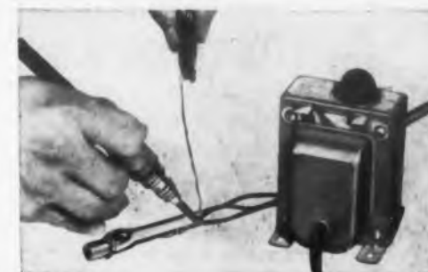
Soldering large telephone jack with Thermo-Tip Resistance Soldering Tool and low voltage Ideal power unit.
