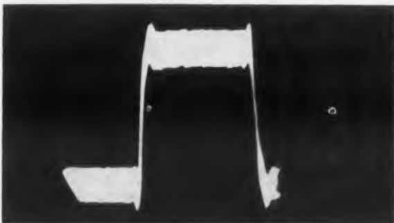
Video amplifier pulse output from commercial TV receiver after passing through 0.7 \mu sec, 1700 ohm Delay-Line Flat.
