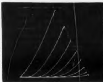
Fig. 1 — Plate current plotted against plate voltage for one triode section of a 12AU7. Plate load is 5 k, peak plate-supply voltage is 500 v. Grid voltage is changed 5 v between curves, from -35 v. to zero. Vertical sensitivity is 5 ma/div, horizontal sensitivity 50 v/div. Calibrated controls permit accurate current and voltage readings directly from the screen.
