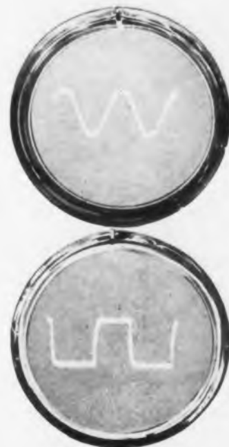
Photos show single transient pulses, 20 microseconds wide with a one microsecond rise time, showing writing capabilities of one million inches per second. These photos were taken in full daylight without a hood.
