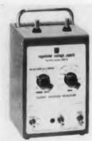
The Model 2004A Regulated Voltage Supply features high stability, compact size, and a wide range of test potentials. Line regulation is within 0.01%; output is 0 to 1 ma. Six taps of 500v, 250v, 100v, 50v, 25v, and 10v are furnished, accurate within 2%. In addition, the potential can be
