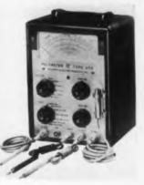
The "302 Polymeter" is a vacuum tube voltmeter that offers a subminiature vacuum tube r-f probe, a peak-to-peak scale, a new 7" meter movement, a lighted scale, a patented linearity circuit, an input impedance of 17 megohms, shielded a-c and r-f leads, and screw-on connectors. The brushed aluminum
