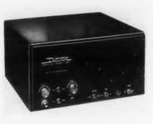
The DS-6100 Frequency Counter will count and display any electrical or mechanical events that can be converted to electrical impulses. The range is from 10 to 100,000 events
