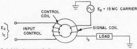
Typical Magnistor gate circuit connections showing control and signal coils.
