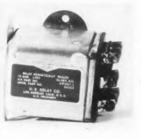
3311-1 relay for military use, this unit is a dpdt, hermetically sealed device with eight screw terminals. Nominal coil voltage is 24-28v d-c. Rated load (contacts) at 29v d-c is 10amp resistive; at
