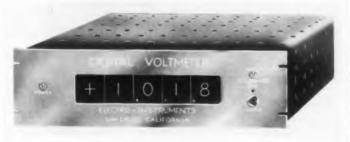
These "Automatic Digital Voltmeters" are designed for reliability, flexibility, and precision. Standard models are available ranging from two to five in-line digits, in voltage ranges from 1mw to 1000v, with automatic ranging indicated by a moving decimal point. Input impedance is 1000 megohms, accuracy is 1 digit, and average time for reading is less than 1see. Models may be specified to operate printers, electric typewriters, or IBM punches.
