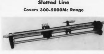
Operating over the frequency range from below 300Mc to 5000Mc, the Type 874-LBA Slotted Line is a convenient and accurate instrument for measurements of impedance, standing-wave ratio, and attenuation. Measurements on dielectric materials, lumped components, coaxial elements, and networks, and antennas in the u-h-f range can be made.
