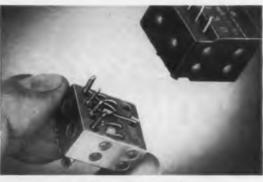
Miniature Rectifier and mount for parts...injection molded of KEL-F Plastic.
