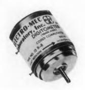
The Type 15 "Digitometer", an analog-digital rotary converter is offered with a shaft torque of only. 0.15oz-in. It provides an accurate means of transposing rotary motion into an equivalent binary numerical notation.
