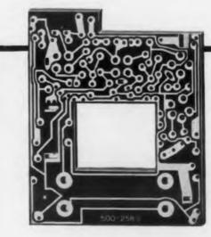
Here's the printed-circuit board used in the Regency ...made with Richardson T-725 copper-clad INSU-ROK. Engineers of I.D.E.A., Inc. of which Regency is a division, laid out the circuit. Croname, Inc.\* Chicago, took it from there .. printed the complex circuit on Richardson T-725 copper-clad INSUROK, then etched it. Results: a lightweight, compact, efficient circuit .. tedious, time-consuming wiring eliminated ...faster assembly.
