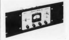
This 8-tube servoamplifier, the Model 32, is designed to drive pneumatic or hydraulic servovalves in power servo applicacations. Features
