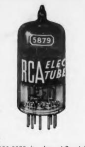
RCA-5879-is a sharp-cutoff pentode of the 9-pin miniature type intended for use as an audio amplifier in applications requiring reduced microphonics, leakage, noise, and hum. It is especially well-suited for input stages of medium-gain public address systems, home sound recorders, and general-purpose audio systems.
