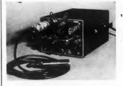
The "Glennite" F 408 decade amplifier is designed for general laboratory use and is provided with an input cathode follower probe. The probe is mounted on a 9'
