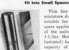
This line of efficient miniature d-c solenoids is suitable for many small space applications. Some of the units weigh only 1-1/2oz. Model A-205 (illustrated) has a push-pull capacity of 9oz with a 1/6'' stroke; 7-1/2oz with a 1/8'' stroke; 6oz with a 3/16" stroke, and 5oz with
