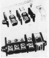
Series N "Alpha Blocks" are sectionalized, easily hand-assembled, terminal blocks designed to provide a variety of combinations with only five major interchangeable parts. Blocks having from one to 100 or more terminal pairs, with or without insulating barriers, can be made from a small box of parts. Any
