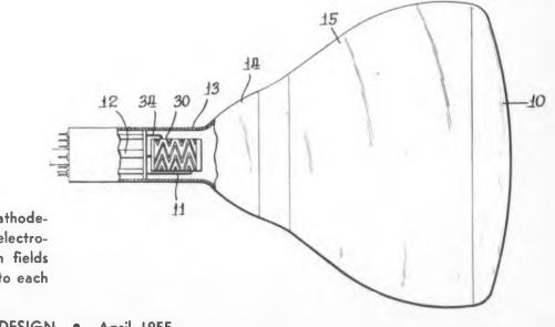
Fig. 2. This cathoderay tube has electrostatic deflection fields at right angles to each other.
