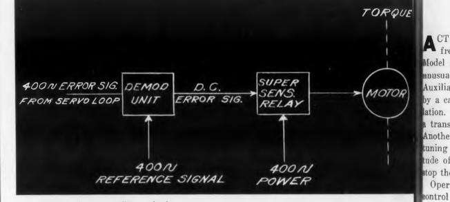
The relay controlling a highpowered motor in a nonproportional servo system.
