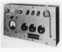
The Model 592 Standard Voltage Ratio Comparator is used for setting accurate voltage ratios, both a-c and d-c, by means of an accurately calibrated voltage divider network
