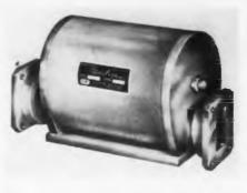
This series of "Uniline" Microwave Load Isolators is capable of operation at peak powers up to 300kw. The units provide substantial load isolation with very low vswr and negli-
