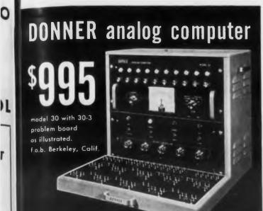
This versatile and compact Donner Model 30 is the first electronic computer specifically designed as a personal tool of the engineer, mathematician and scientist. It offers the speed and accuracy of electronic computation with slide rule operating simplicity wherever differential equations are used.
