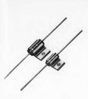
COPPER clamps encircling a standard composition resistor increase its heat transfer capabilities. These copper clad resistors are considerably smaller than wire-wound units of comparable rating and are relatively non-inductive. All standard values and tolerances for composition resistors are available starting at 2.7 ohms in one instance and extending to 22 megohms.
