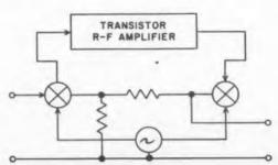
Fig. 25. D-c amplification by carrier techniques.
