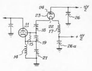
Fig. 4. This high-voltage supply does not require a high-frequency transformer.
