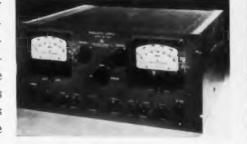
Designed to be utility power supplies for laboratory and development use, the units have ratings ranging up to 500v d-c at 200ma. The dual unit has a switch for series or parallel connection, thus making possible combined ratings to 1000v or 40ma.
