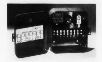
The Model EB Electronic Pilot Relay is able to control large values of current and power with a current flow of 2µamp. It permits delicate mechanisms with extremely light contact pressures to control larger electrical currents. Its unusual cold cathode triode tube design and construction gives instantaneous action, unlimited lead lengths, and a current amplification up to 2.5 x 10<sup>6</sup>.
