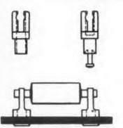
Three types of diode clips have been made available, capable of holding crystal diodes with shaft diameters of 0.075" to 0.080". Model No. 9000 is designed for front panel mounting and Model No. X9000 is for front panel mounting with a
