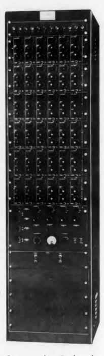
Generator has 5 channels and 40 line segments. Accuracy depends on number of diodes used.
