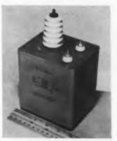
This oil-immersed a-c transformer is for use in high-voltage test equipment and high - voltage power supplies. At present, its production is limited to custom business, including prototype and large production orders.
