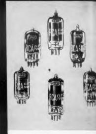
YOUR CHOICE OF COMPUTER TUBES RCA-5915, 5963, 5964, 5965, 6197, 6211 ... Dependable performance, a must in computer applications, is accomplished in these six RCA tubes—by using production controls correlated with typical electronic computer conditions. RCA computer tubes feature controlled cutoff for switching applications, low-grid current for applications utilizing high values of grid resistance, high zero-bias plate current, special cathode material to minimize interface, and low leakage.
