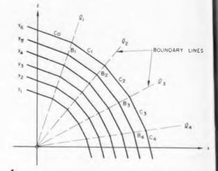
Simple function z=f(x,y) where y, as fixed by boundary lines, is linear.
