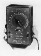
Capacitance Bridge Model C-10 has been added to the line of "Signa-Glow" instruments. It incorporates a newly designed visual null indicator consisting of a pair of glow lamps which indicate both the degree and direction of unbalance at a glance.
