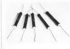
The LP-5 is a 5w glass resistor unit available in ratings from 200 ohms to 60,000 ohms and should be especially valuable for color TV. It is manufactured by having a
