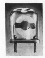
The "Cryst-O-glas" quartz crystal unit features an all glass case and holder, providing a perfectly hermetically sealed container. Because heat alone is used in the bonding operation, the crystal itself is never subjected to the chemical fumes given off by conventional sealing compounds. This absence of contamination re
