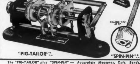
Ejects and Assembles both leads simultaneously to individual lengths and shapes — 3 minute set-up — No accessories — Foot operated — 1 hour
