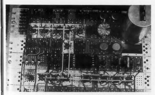
A relay-rack-mounted prototype constructed with the Circuit Assembler.
