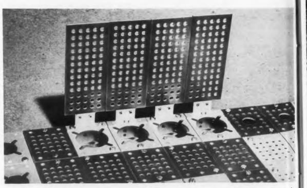
These are some of the panels that can be used in this breadboard system. The terminals are easily inserted into the panels with a screwdriver.
