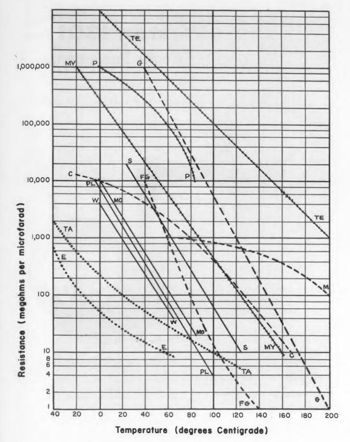
Capacitors with low leakage characteristics can be chosen by means of this chart. 13 insulations given.
