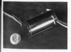
The HIG-3 Hermetically sealed Integrating Gyro is a 400ey unit. It has an angular momentum of  $10^3$ gram cm<sup>2</sup>/sec. Gimbal travel is  $\pm 6^{\circ}$ max. Input rate is 2 radians per sec
