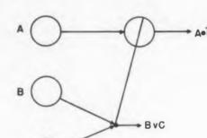
Fig. 4. A magnetic-core inhibit circuit, its symbolic representation, and two other symbolic inhibit circuits are used for high-speed logic in computers.
