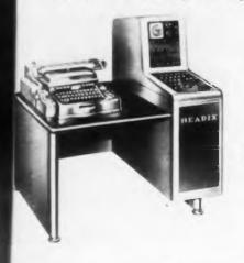
The "Readix" is a decimal, serial, single-address machine with a magnetic storage capacity of 4000 words. Each word consists of 10 decimal digits with sign, or two commands, complete with addresses. Use of the decimal system ible with standard
