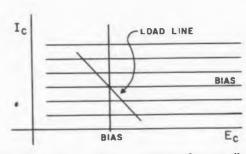
Fig. 23. Very linear characteristics for small signals.
