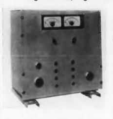
The Model 306 regulated d-c power supply is designed to deliver high-current, highvoltage power for microwave and nuclear applications. It features high stability and regulation. Originally developed to supply a traveling
