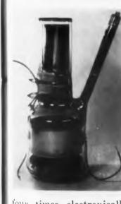
Known as the Super Iconoscope, this tube has a continuously coated surface replacing the standard mica mosaic of the more costly image orthicon-type tubes. The Super Iconoscope requires a simpler power supply (-1200v) and provides up to 1000-line rasters. The resolution and sensitivity approaches that of orthicon tubes. The tube enlarges pictures up to
