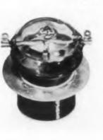
This firm's smallest highvoltage tacuum relay, the Type R5-E, is designed for pulse network, antenna transfer, and guided missile applications. Size is only 3" long x 2" diam, including a 12v or 24v d-c actuating solenoid located in the base. The vacuum dielectric
