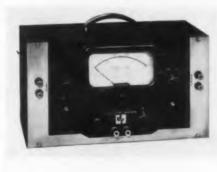
This portable, low-cost Flutter and Wow Meter, Model FL-3B, measures flutter and wow at 3kc in tape, film, wire, and disk recordand reproing ducing equip-
