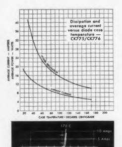
HIGH CURRENT - to 15A HIGH VOLTAGE RATINGS HIGH TEMPERATURE - 175°C
