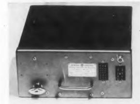
were designed to enclose the chassis. Support for the chassis is supplied by the illustrated internal relay rack arrangement instead of the enclosure. This construction affords the greater rigidity necessary for mobile installations. Known as the "Progress Line", this equipment is made by General Electric Co., Syracuse, N. Y.
