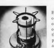
The "Horo" Electro-Bunsen Burner, is capable of achieving temperatures of 850°C under continuous operation, yet eliminates the hazard of fire and explosion. Operation is clean and odorless, because heating is accomplished by a stream of hot air, and no soot is deposited on the heated object. Heat is even, with no local over-
