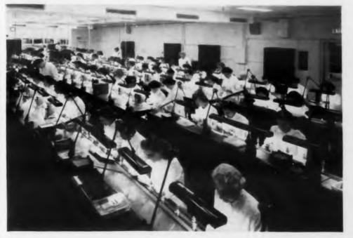
**HOSPITAL-CLEAN** conditions minimize danger of contamination from air borne lint or dust particles that might lead to catastrophic tube failures.
