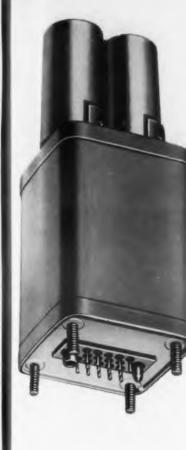
The thyratron tubes can be removed from this version of the unit.
