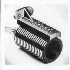
"Eldec" standard slip ring and spring loaded brush contact assemblies are available in 10 combinations of either 2, 4, 6, 8, 10, 12, 14, 16, 18, or 20 silver rings, 4µinch finish, with 1, 2, 3, or 4 silver graphite brush contacts
