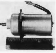
Available in six different models with or without gear-reduction units, the motor operates with a smaller air gap than is customary, without any deterioration of commutation and without increasing the loss in field shoes, due to specially shaped and laminated field shoes. Longer life and better motor performance is assured by mica insulated commutators.
