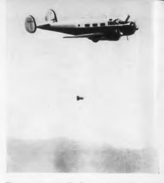
This magnetometer "bird" is measuring the earth's magnetic field. The bird is nothing more than a streamlined case enclosing a bottle of water and a coil of wire. The aircraft's magnetic field does not influence the accuracy of the results.
