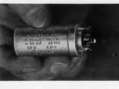
"Push-Lok" 28D dry electrolvtic capacitors have a mounting design which makes assembly - line connection in printed wir-
