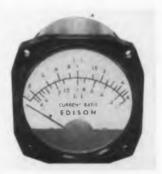
This panel meter has the capacity to handle 50ma in either coil, and will accurately indicate a ratio on an input of 2ma minimum. Scale tolerances are based on an angular tolerance of 1°.
