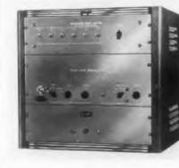
The CPA-1 Color Phase Analyzer is designed to analyze the chrominance components of composite color video signals. The unit compares the phase of chrominance components with respect
