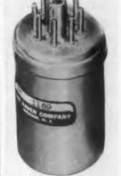
These hermetically sealed wire-wound resistance and resistance-capacitance networks can be supplied with resistance values to  $\pm 0.02\%$  and temperature coefficients matched to within  $\pm 3$  parts per million per degree centigrade. The networks are encased in "Sealed-Ohm" cases with plugin or solder terminals. All units are hermetically
