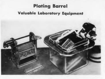
The 3II miniature oblique plating barrel has a cylinder 3" in diameter x 3" deep, with approximately 1/4 lb load capacity. It is a complete bulk plating machine, consisting of a high temperature plexiglass tank and cylinder and a 110v 60cy single-phase motor drive. Because tank capacity is only 1 gal, the unit is well suited for precious metal plating where solution volumes must be kept small. In addition, it is useful for cleaning, pickling, and deplating of precious metal parts for reclamation
