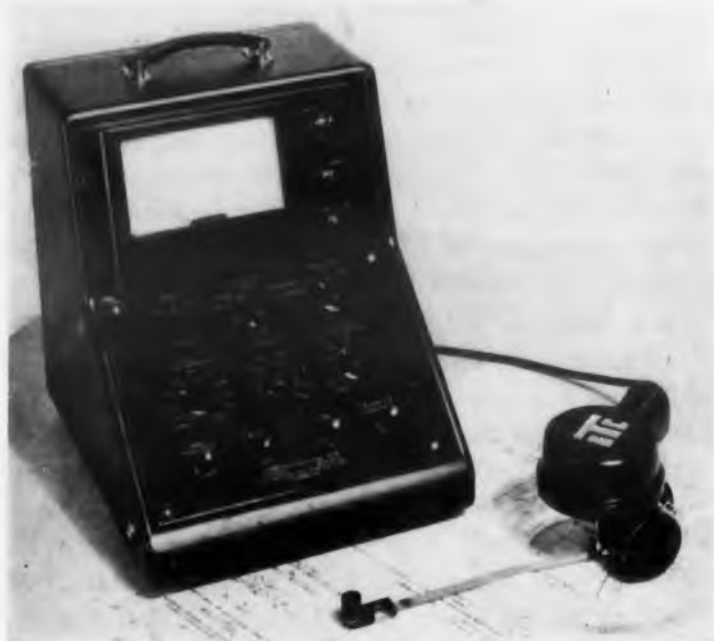
Fig. 1 (above). Complex vectors can be multiplied and divided quickly and accurately by the Complex Plane Analyzer. The vector measuring unit is at the right.
