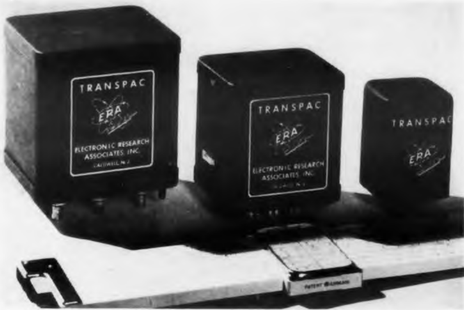
Fig. 1. These miniaturized d-c power packs come in many sizes with inputs and outputs to suit a wide variety of electronic applications.
