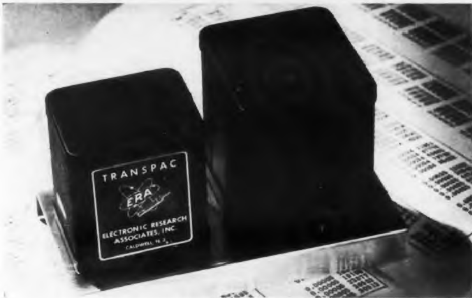
Fig. 2. A typical application of the "Transpac" is this transistorized computer unit. The transistors and other components are in the can at the right.
