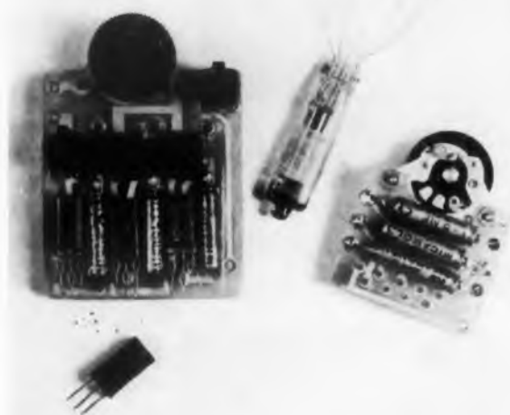
Fig. 5. Model Two (left) and the Model One (right) amplifiers next to a subminiature tube and a transistor to show relative size.
