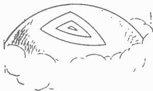
Fig. 2. Three triangles drawn on the earth's curved surface. The sum of the angles is obviously greater than 180 degrees.
