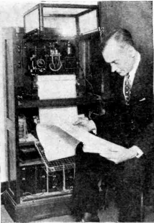
The photograph at the left shows New York's Health Commissioner Wynne studying the chart of the sunlight recorder in the office of the National Conference Board on Sanitation, as picked up by the photo-electric cell illustrated below.
