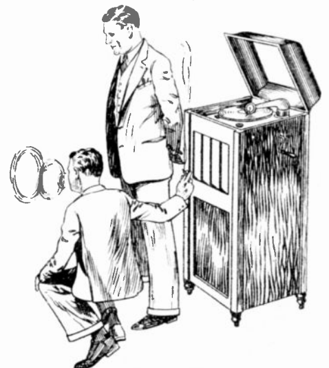
Fig. 5—Sound waves pass through the body of the man standing in front of the phonograph. They strike the smoke ring and turn it around 90 degrees.
