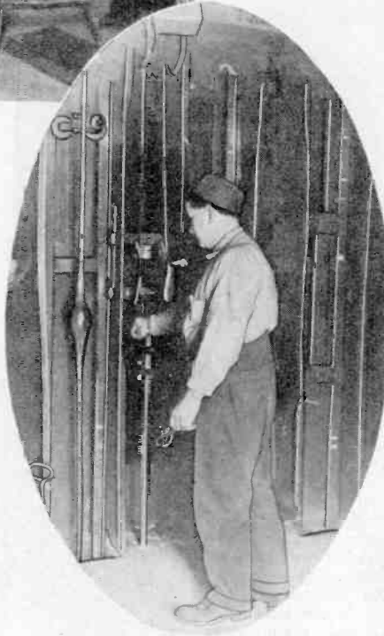
Left — Hand tube drawing. The man at left slowly pulls the semi-liquid mass of glass attached to the end of his blow-pipe, into tubing of the correct diameter. Below—At the base of the thermometer tube drawing tower. A "gather" of glass is set in a long vertical corridor where it is drawn upward.
