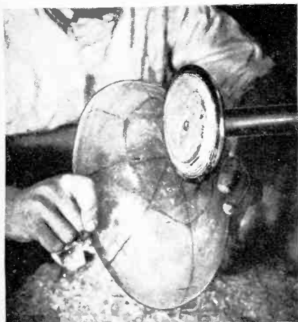
Having marked the main guiding lines of the design, the craftsman starts out to make a beautiful cut-glass bowl.
