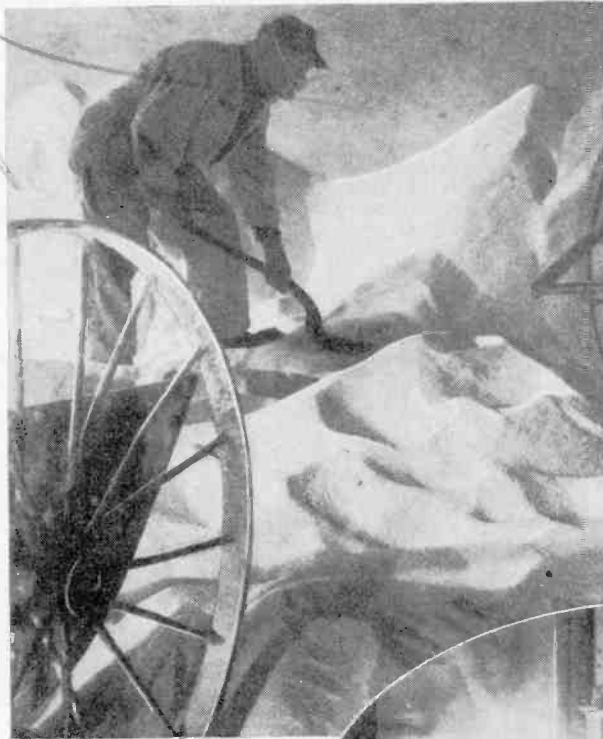
Above — Mixing the raw, or "batch" material ready for melting. Right — Feeding one of the furnaces with raw material for melting into glass.
