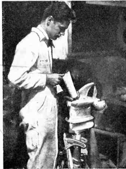
Malcolm Pope, well-known outboard racer, putting racing compound in the lower unit of his engine.
